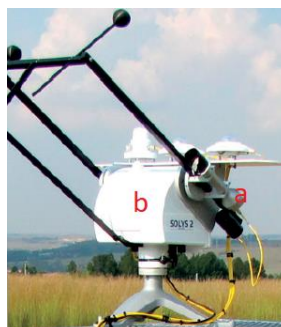
Figure 2-14: Assembly to measure BNI.
