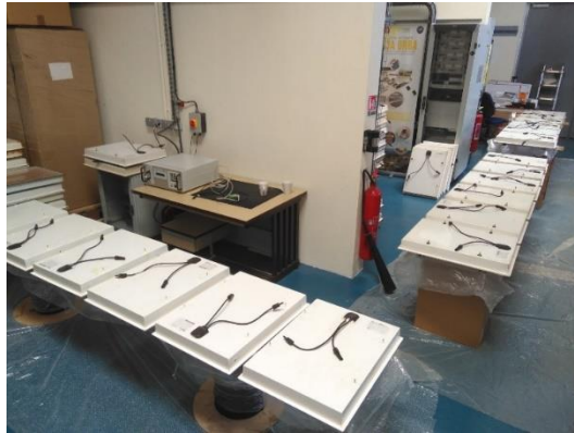
Figure 3-21: Cleaning and inspection of all HCPV modules
