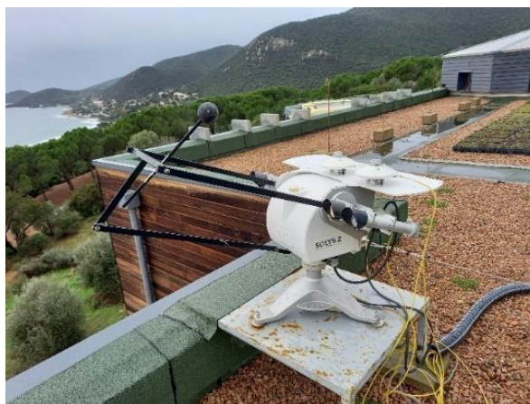
Figure 3-16: Tracker assembly to measure GHI, BNI and DHI
