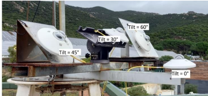
Figure 3-14: Pyranometers for tilted global irradiance measurement.
