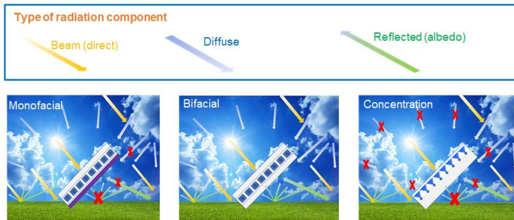
Figure 1-2: Different PV modules and usable radiation components
