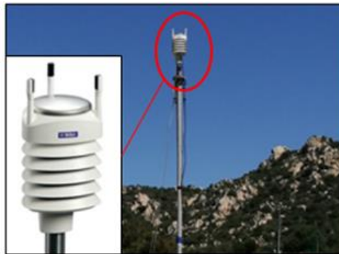
Figure 3-15: A weather station installed for wind, humidity and temperature measurements.
