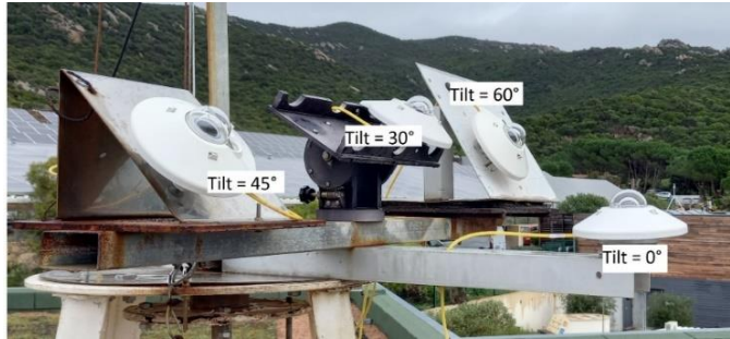
Figure 3-14: Pyranometers for tilted global irradiance measurement.
