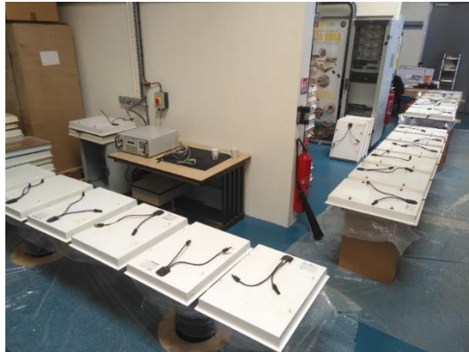
Figure 3-21: Cleaning and inspection of all HCPV modules
