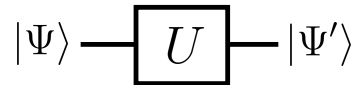
Figure 1.2: A quantum system in state |\Psi\rangle evolves under the transformation U , which results in the new state |\Psi'\rangle .
