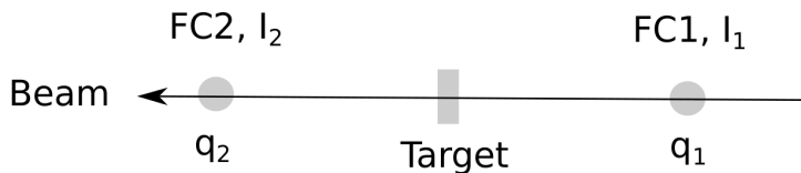
Figure 2.18: Scheme of the Faraday cups system used in the STELLA experiment before and after the target, measuring intensities I_1 , I_2 at charged states q_1 , q_2 [40].
