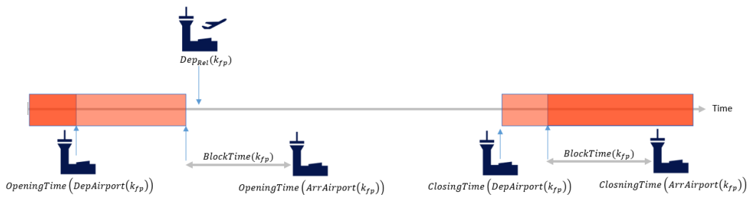
Figure 8: Illustration of Departure Constraints caused by the opening and closing time of the airports.
