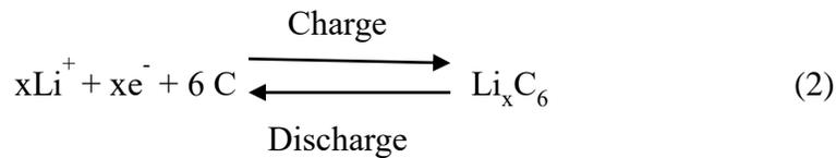
During the discharge, the opposite phenomenon is observed: the transition metal is reduced and the lithium ions are again intercalated in the positive electrode host material. The interest of such system lies in the possibility of storing electrical energy (in chemical form) during charging and in the restitution of this energy during discharge.
