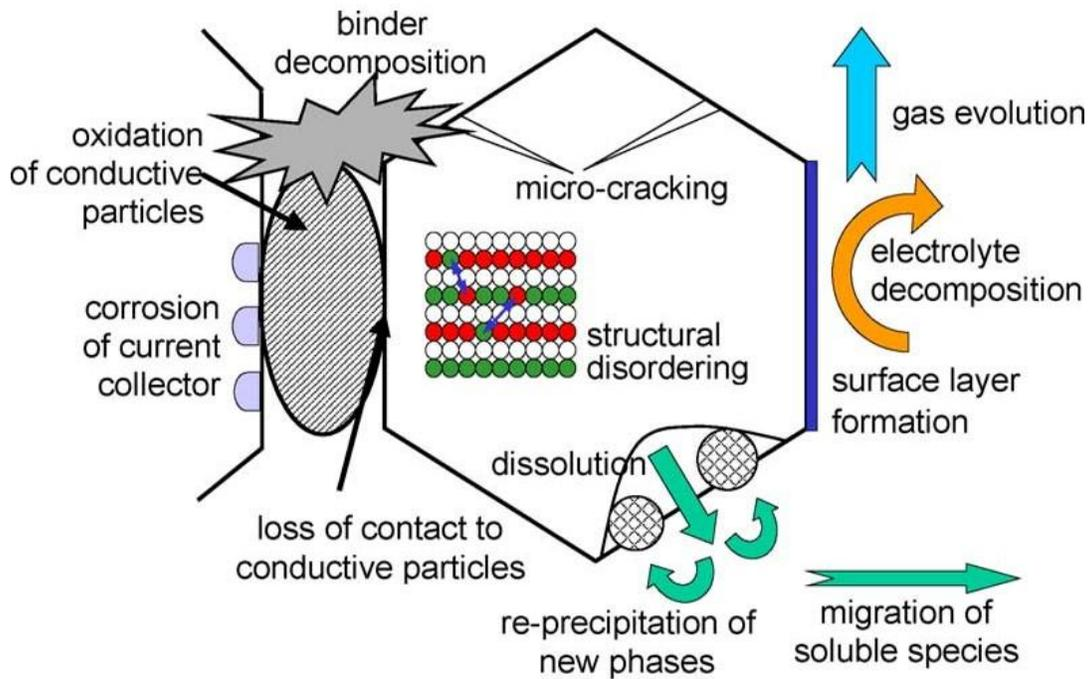
Figure 7. Overview on degradation mechanisms of positive electrode material from Vetter *al.*<sup>22</sup>
