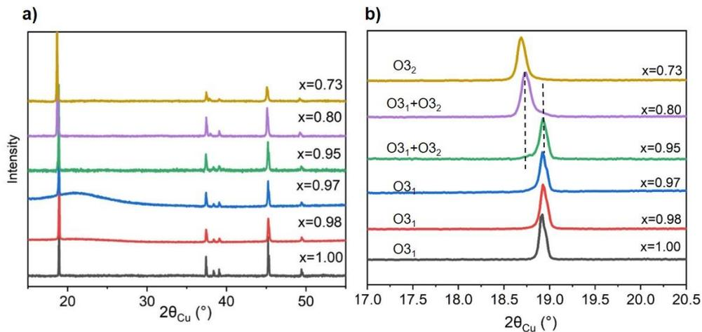
Figure A. 26. a) X-ray diffraction patterns of the electrochemically deintercalated  $\text{Li}_x\text{Co}_{0.96}\text{Al}_{0.04}\text{O}_2$  materials prepared with targeted Li compositions by controlling the Li content, in the low potential region  $V < 4V$  vs  $\text{Li}^+/\text{Li}$  with b) the detail in the (003) line.
