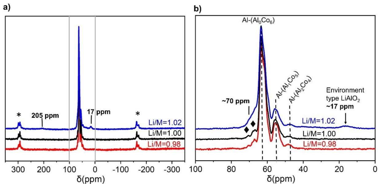
Figure A. 8. (a)  $^{27}\text{Al}$  and MAS NMR spectra of 2% Al doped  $\text{LiCoO}_2$  samples with various Li/M ratio ( $M = \text{Co} + \text{Al}$ ). A zoom in the central transitions is given in (b) (\*: spinning sidebands, ◆: satellite transitions at 69 and 73 ppm)
