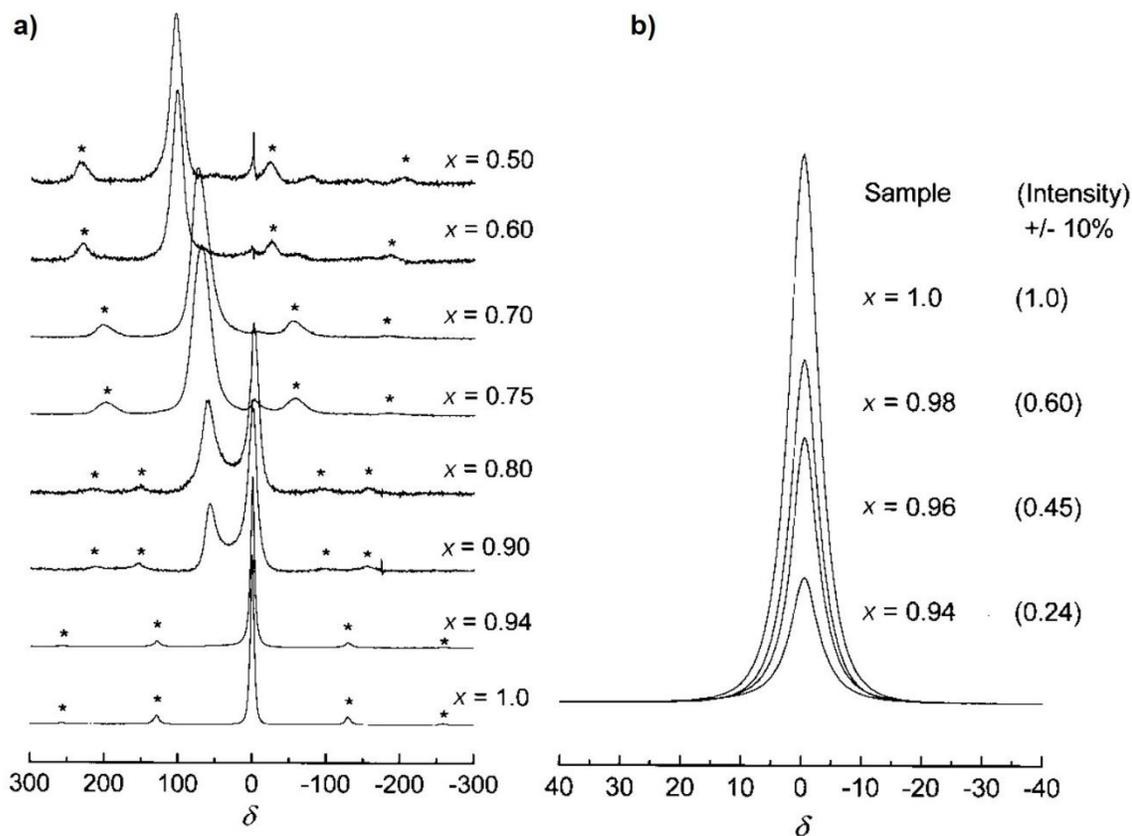
Figure 17. <sup>7</sup>Li MAS NMR spectra for the various Li<sub>x</sub>CoO<sub>2</sub> deintercalated phases (\*=spinning sidebands) from Ménétrier et al.<sup>14</sup>
