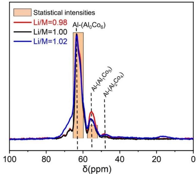
Figure A. 10.  $^{27}\text{Al}$  MAS NMR spectra recorded at 130.33 MHz using a 30 kHz spinning frequency of the 2% Al doped  $\text{LiCoO}_2$  samples in comparison with the theoretical intensity distribution of the different Al environments versus Co, expected for a 2% Al-doped sample.
