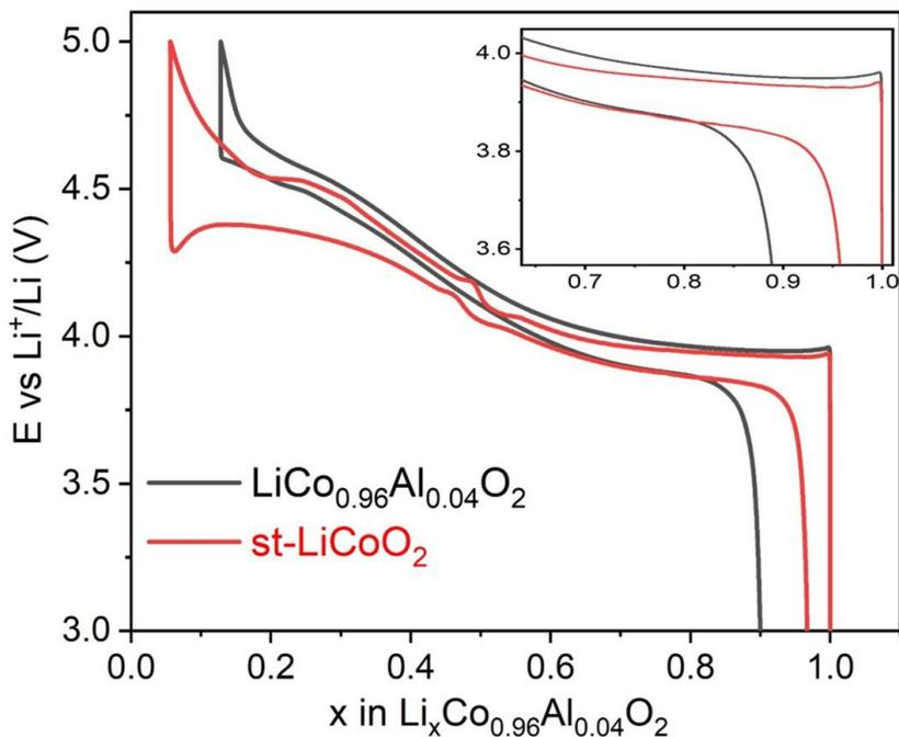
Figure A. 20. The first charge–discharge curves in the 3–5 V voltage range vs. Li<sup>+</sup>/Li of Li<sub>x</sub>Co<sub>0.96</sub>Al<sub>0.04</sub>O<sub>2</sub> and Li<sub>x</sub>CoO<sub>2</sub> samples (C/20 cycling rate).
