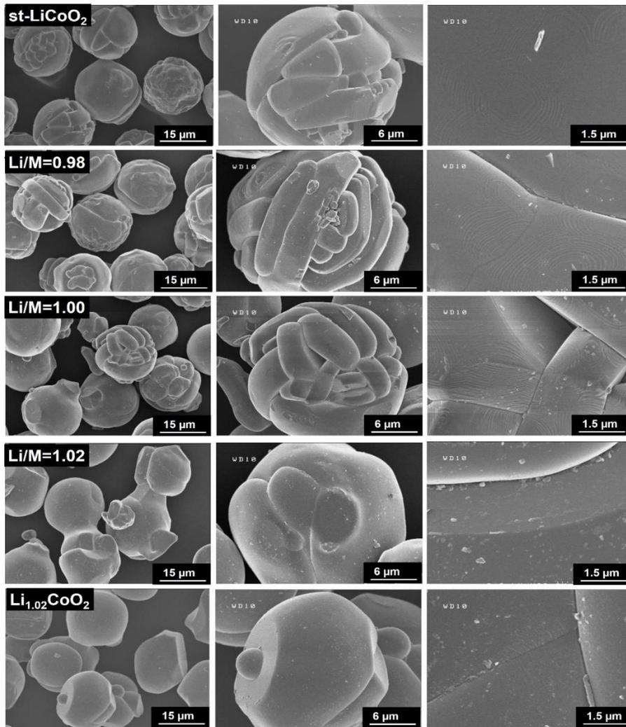
Figure A. 2. SEM micrographs of 2% Al doped  $\text{LiCoO}_2$  samples with various  $\text{Li/M}$  ratio ( $M = \text{Co} + \text{Al}$ ), compared to  $\text{st-LiCoO}_2$ .
