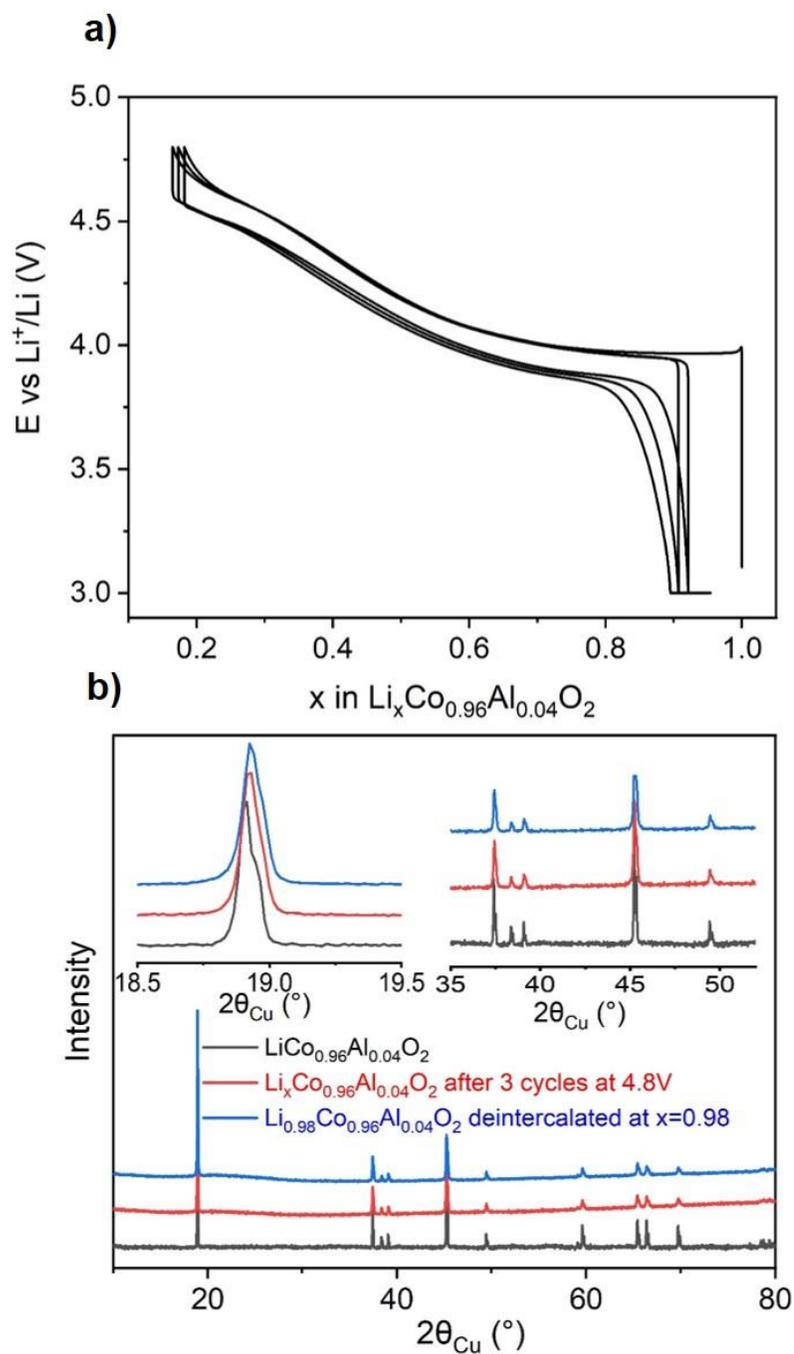
Figure A. 31. a) 3 cycles of galvanostatic charge / discharge (3V-4.8V) of an Li //  $\text{Li}_x\text{Co}_{0.96}\text{Al}_{0.04}\text{O}_2$  and stopped in potential at 3V cell with a rate of C/20. b) X-ray diffractogramme of  $\text{Li}_x\text{Co}_{0.96}\text{Al}_{0.04}\text{O}_2$  cycled compared to the pristine and the deintercalated  $\text{Li}_{0.98}\text{Co}_{0.96}\text{Al}_{0.04}\text{O}_2$ .
