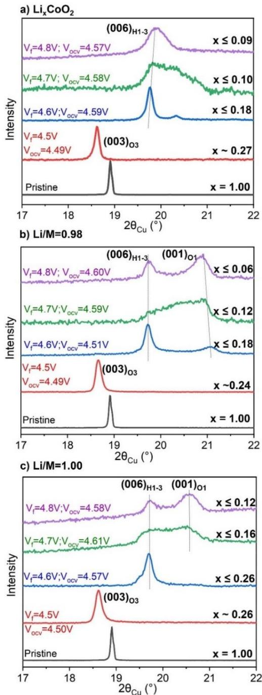
Figure B. 18. Detail in the (001) line from XRD for a) *st*- $\text{LiCoO}_2$ , b)  $\text{Li}/\text{M}=0.98$  and c)  $\text{Li}/\text{M}=1.00$  ( $V_{\text{ocv}}$  corresponds to the voltage measured at the end of relaxation before disassembling the cell and  $V_f=V_{\text{floating}}$ ).
