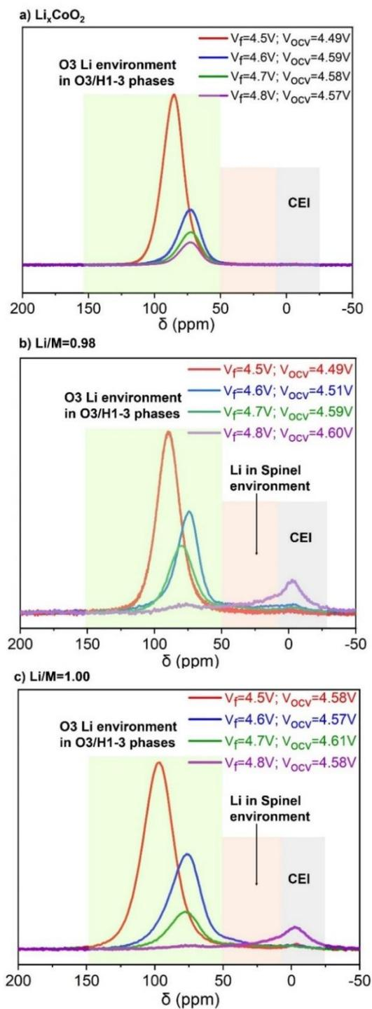
Figure B. 19. Ex-situ  $^7\text{Li}$  MAS NMR spectra for 2% Mg doped  $\text{LiCoO}_2$  materials (Hahn echo,  $B_0 = 7.05\text{T}$ ,  $V_{ocv}$  corresponds to the voltage measured at the end of relaxation before disassembling the cell and  $V_f=V_{floating}$ ).
