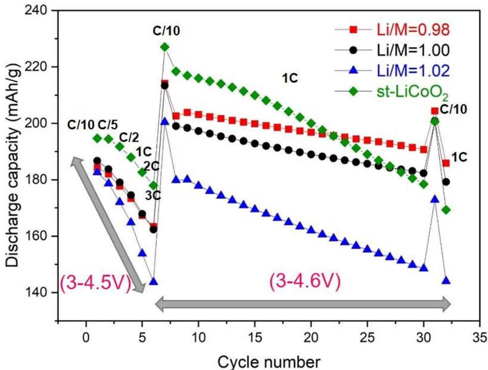
Figure A. 15. Cycling performances of *st*-LiCoO<sub>2</sub> compared to Al doped LiCoO<sub>2</sub> with various *Li/M* ratios using different *C* rates.
