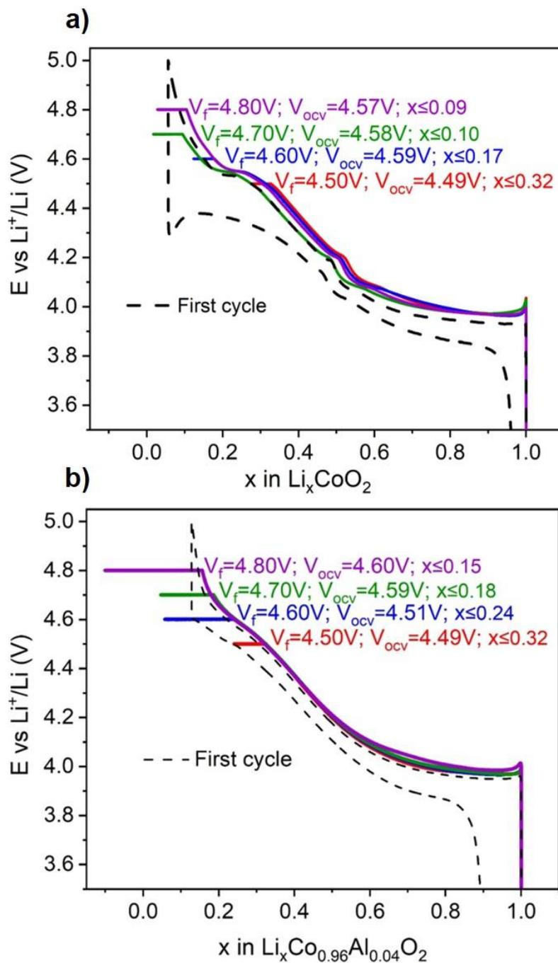
Figure A. 29. Galvanostatic charge of Li//LiCo<sub>0.96</sub>Al<sub>0.04</sub>O<sub>2</sub> cells stopped at different voltage from 4.5V to 4.8 V compared to a first cycle curve ( $V_f = V_{floating}$  and  $V_{ocv}$  corresponds to the voltage measured before disassembling the cell).
