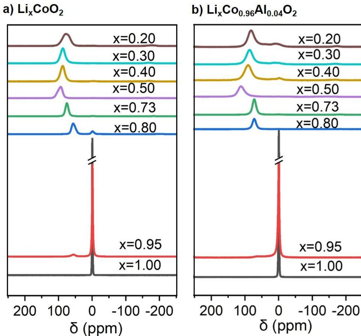
Figure A. 25. Ex-situ <sup>7</sup>Li MAS NMR spectra for a) Li<sub>x</sub>CoO<sub>2</sub> and b) Li<sub>x</sub>Co<sub>0.96</sub>Al<sub>0.04</sub>O<sub>2</sub> (rotor-synchronized Hahn echo sequence,  $\nu_R = 30$  kHz). Arbitrary intensities are used here to better visualize the shifts.
