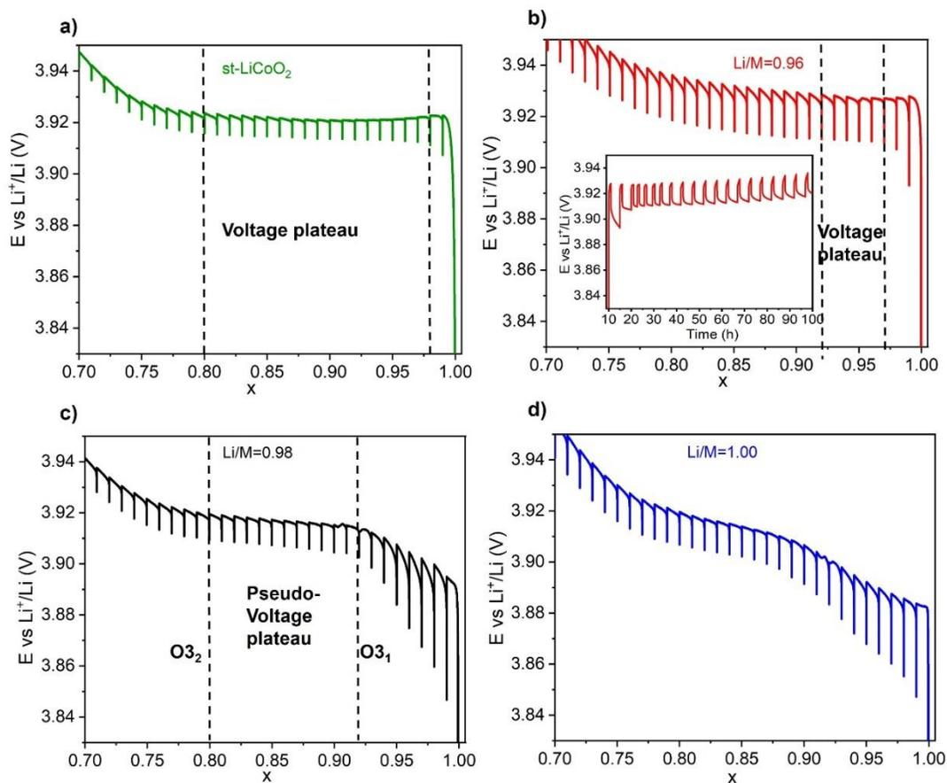
Figure B. 15. First GITT charge of a Li standard a) *st*-LiCoO<sub>2</sub> compared to Mg doped LiCoO<sub>2</sub> with b) Li/M=0.96, insert the corresponding curve as a function of time c) Li/M=0.98 and d) Li/M=1.00 cells 300 h (1h charge using C/100 rate and 4h relaxation).
