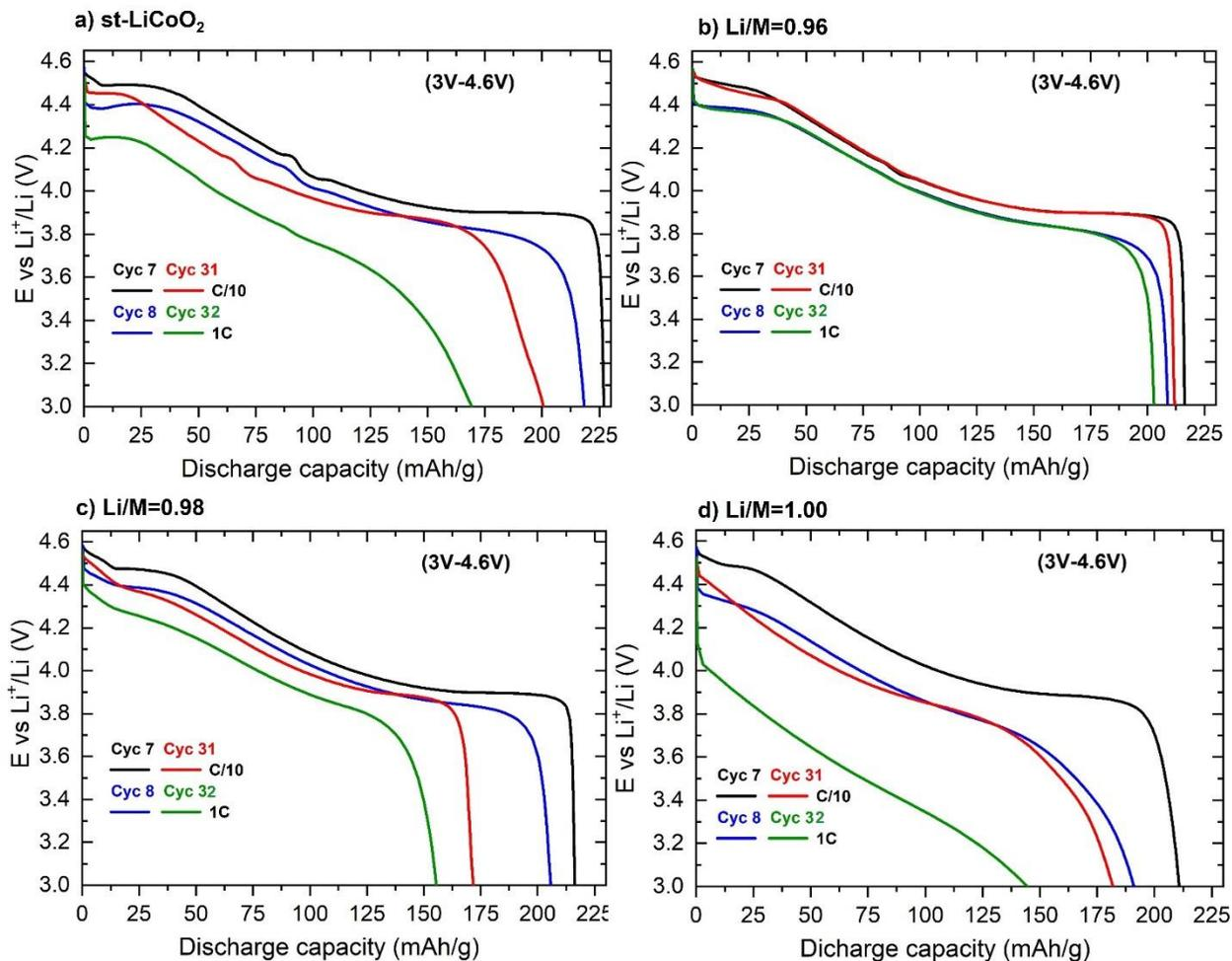
Figure B. 13. Discharge profiles (3V-4.6V) of Li//LiMO<sub>2</sub> cells observed for the 7, 8, 31 and 32<sup>th</sup> cycles of a) st-LiCoO<sub>2</sub> compared to Mg doped LiCoO<sub>2</sub> with various Li/M ratios using C/10 and 1C rates.
