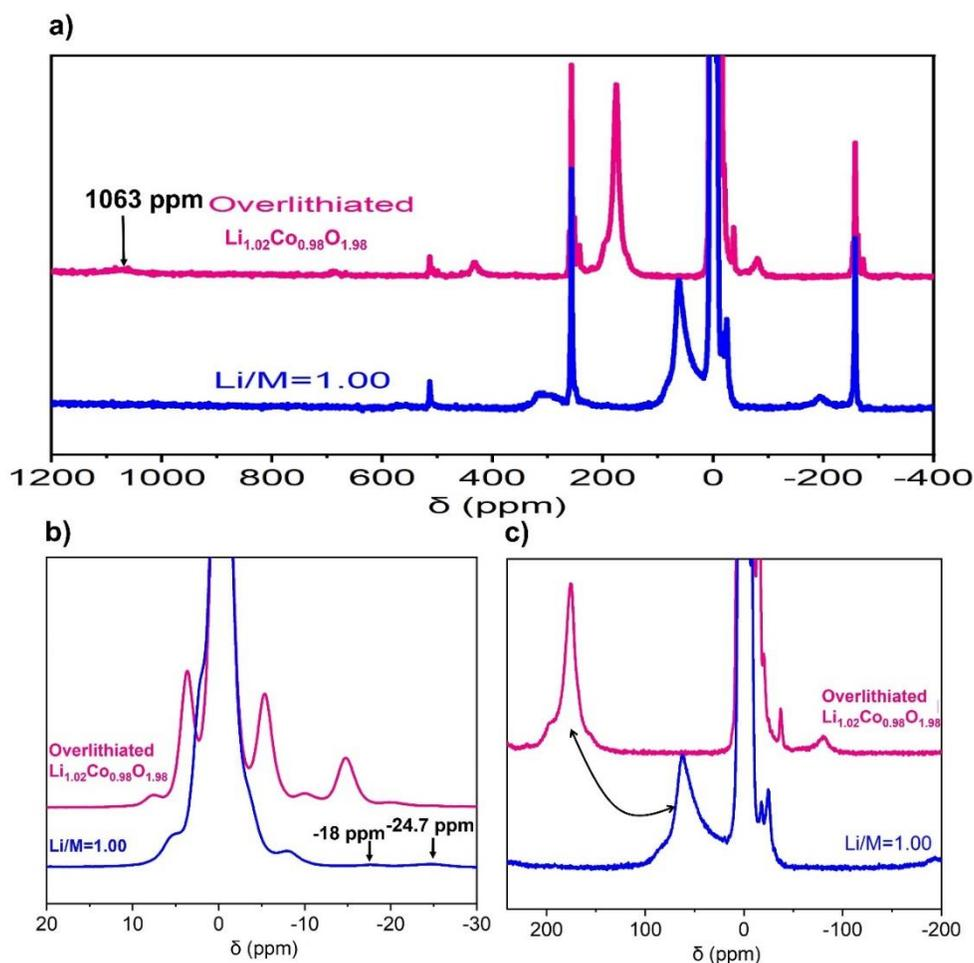
Figure B. 6. (a)  ${}^7\text{Li}$  MAS NMR spectra of  $\text{LiCo}_{0.98}\text{Mg}_{0.02}\text{O}_2$  compared with the overlithiated  $\text{Li}_{1.02}\text{Co}_{0.98}\text{O}_{1.98}$  sample (Hahn echo,  $B_0 = 7.05\text{T}$  \*: spinning sidebands), with a zoom in (b)  $20\text{ ppm} \leq \delta \leq -30\text{ ppm}$  (c) and  $-200\text{ ppm} \leq \delta \leq 200\text{ ppm}$  region.
