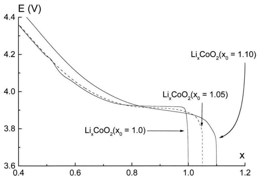
Figure 14. First galvanostatic charge of  $\text{LiCoO}_2$  synthesized with  $\text{Li/Co} = 1.00, 1.05$  or  $1.10$ , from Levasseur et al<sup>54</sup>
