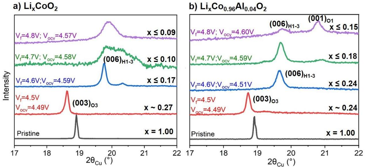
Figure A. 30. Detail in the (00l) line from XRD for a)  $\text{Li}_x\text{CoO}_2$  and b)  $\text{Li}_x\text{Co}_{0.96}\text{Al}_{0.04}\text{O}_2$  ( $V_f=V_{\text{floating}}$  and  $V_{\text{ocv}}$  corresponds to the voltage measured before disassembling the cell).
