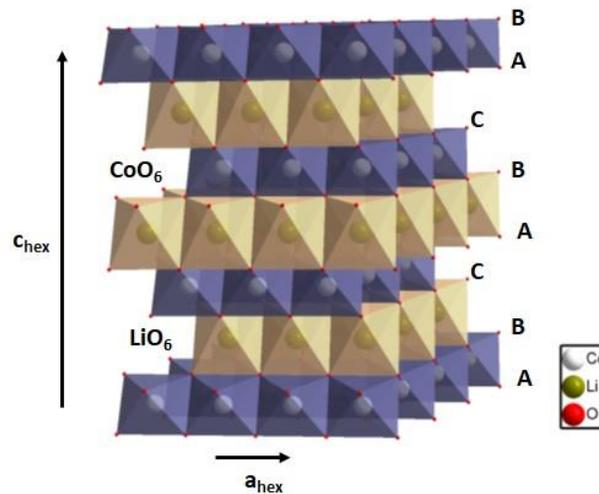
Figure 4. Schematic representation of the structure of  $\text{O3-LiCoO}_2$
