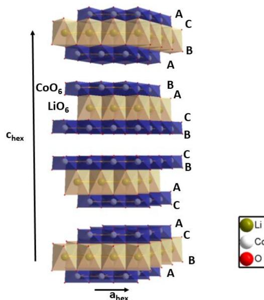
Figure 9. Schematic representation of the H1-3 phase with  $a_{hex}=b_{hex}=2.78 \text{ \AA}$  and  $c_{hex}=25.95 \text{ \AA}$  according to Van der Van et. al.<sup>18,28</sup> Cobalt, lithium, oxygen 1 and oxygen 2 occupied the  $3a (0,0,0)$ ,  $6c (0,0,0.425)$ ,  $6c (0,0,0.277)$  and  $6c (0,0,0.115)$  Wyckoff positions
