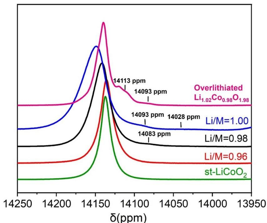
Figure B. 8. <sup>59</sup>Co MAS NMR spectra of 2% Mg doped LiCoO<sub>2</sub> samples with various Li/M stoichiometry compared to stoichiometric and overlithiated Li<sub>1.02</sub>Co<sub>0.98</sub>O<sub>1.98</sub>
