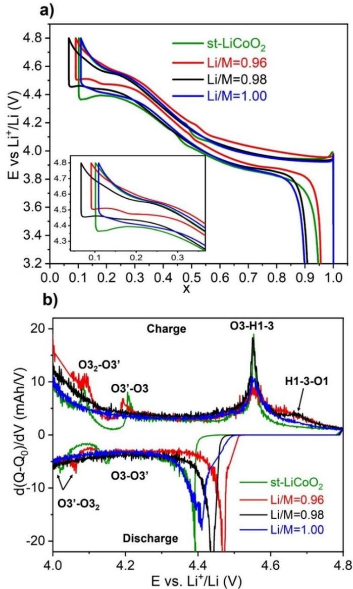
Figure B. 16.(a) First cycle for st-LiCoO<sub>2</sub> compared to Mg doped LiCoO<sub>2</sub> with various Li/M ratios at C/20 up to 4.8 V. Insert: Zoom on the high voltage electrochemical window of the curves plotted. (b) Corresponding  $d(Q-Q_0)/dV$  curves for 4-4.8V window.
