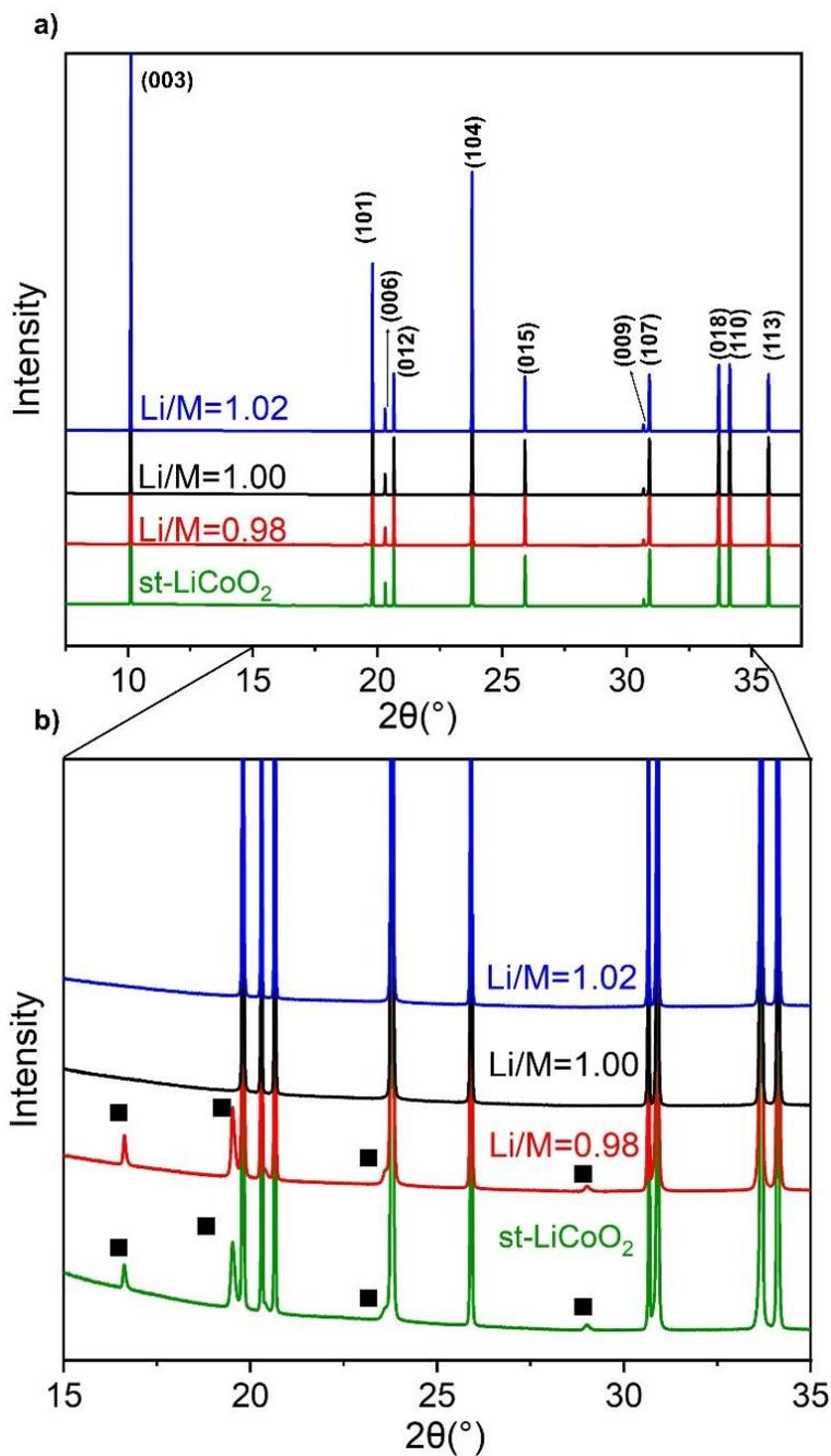
Figure A. 3. S-X-ray powder diffraction patterns for 2% Al doped  $\text{LiCoO}_2$  compared with  $\text{st-LiCoO}_2$ . A zoom in the b)  $15^\circ$  to  $35^\circ$  region (All the patterns were collected with  $\lambda = 0.826 \text{ \AA}$ ,
