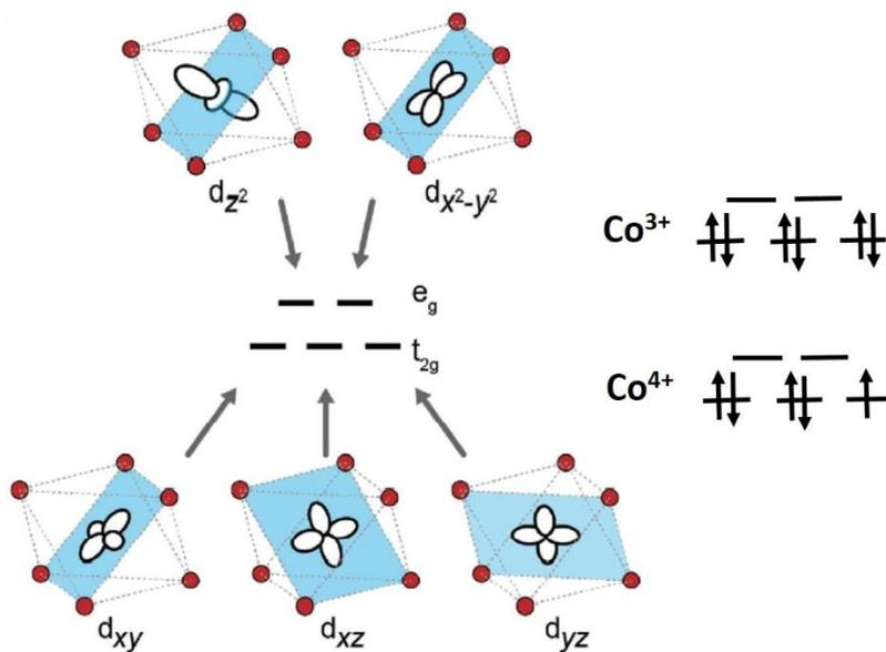
Figure 15. Crystal field splitting of d orbitals in an octahedral environment with the electronic configuration of the Co ions in the octahedral symmetry reproduced from Radin et al.<sup>32</sup>
