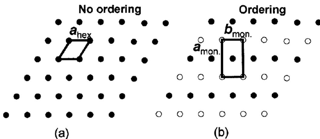
Figure 6. Schematics of (a) lithium ion positions in  $\text{LiCoO}_2$  or randomly distributed lithium and vacancy positions in  $\text{Li}_x\text{CoO}_2$  and (b) ordered lithium and vacancy positions in  $\text{Li}_x\text{CoO}_2$  ( $x = 0.5$ ), where the hexagonal and monoclinic cells are drawn.<sup>18</sup>
