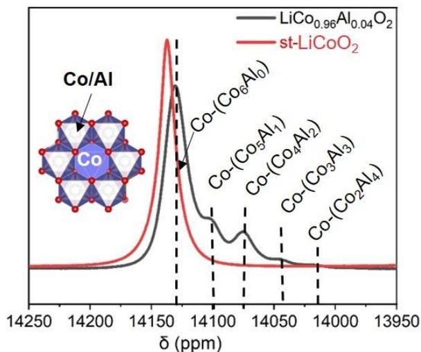
Figure A. 19. a)  $^{27}\text{Al}$  and b)  $^{59}\text{Co}$  MAS NMR of the  $\text{LiCo}_{0.96}\text{Al}_{0.04}\text{O}_2$  compared to  $\text{st-LiCoO}_2$  (◆: satellite transitions).
