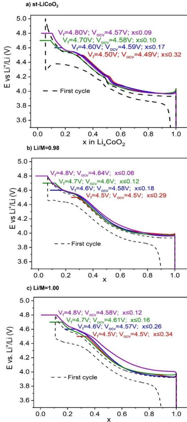
Figure B. 17. Galvanostatic charge of a) st-LiCoO<sub>2</sub>, b) Li/ Li/M=0.98 and c) Li/ Li/M=1.00 cells stopped at different voltage from 4.5 to 4.8 V compared to the first charge-discharge curve ( $V_{ocv}$  corresponds to the voltage measured at the end of relaxation before disassembling the cell and  $V_f=V_{floating}$ ).
