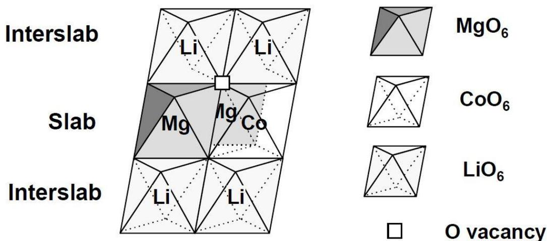
Figure B. 7. schematic representation of the local configuration of the structural defect revealed in the  $\text{Li}_x\text{Co}_{1-y}\text{Mg}_y\text{O}_2$  phases from Levasseur Phd.<sup>15</sup>
