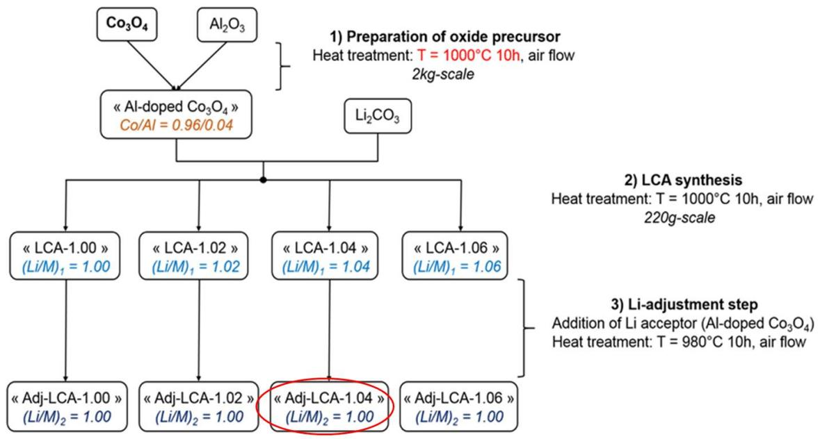
Figure A. 16. Schematic representation of synthetic routes for 4 % Al doped  $\text{LiCoO}_2$  from Duffiet's PhD.<sup>27</sup>
