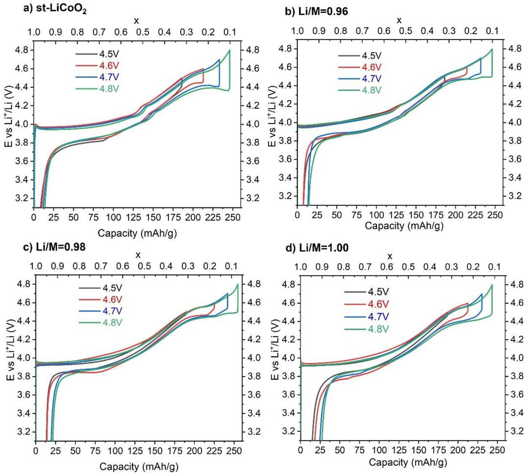
Figure B. 12. First cycle recorded at C/20 and up to various cutoff voltage for a) st-LiCoO<sub>2</sub> compared to Mg doped LiCoO<sub>2</sub> with b) Li/M=0.96, c) Li/M=0.98 and d) Li/M=1.00.
