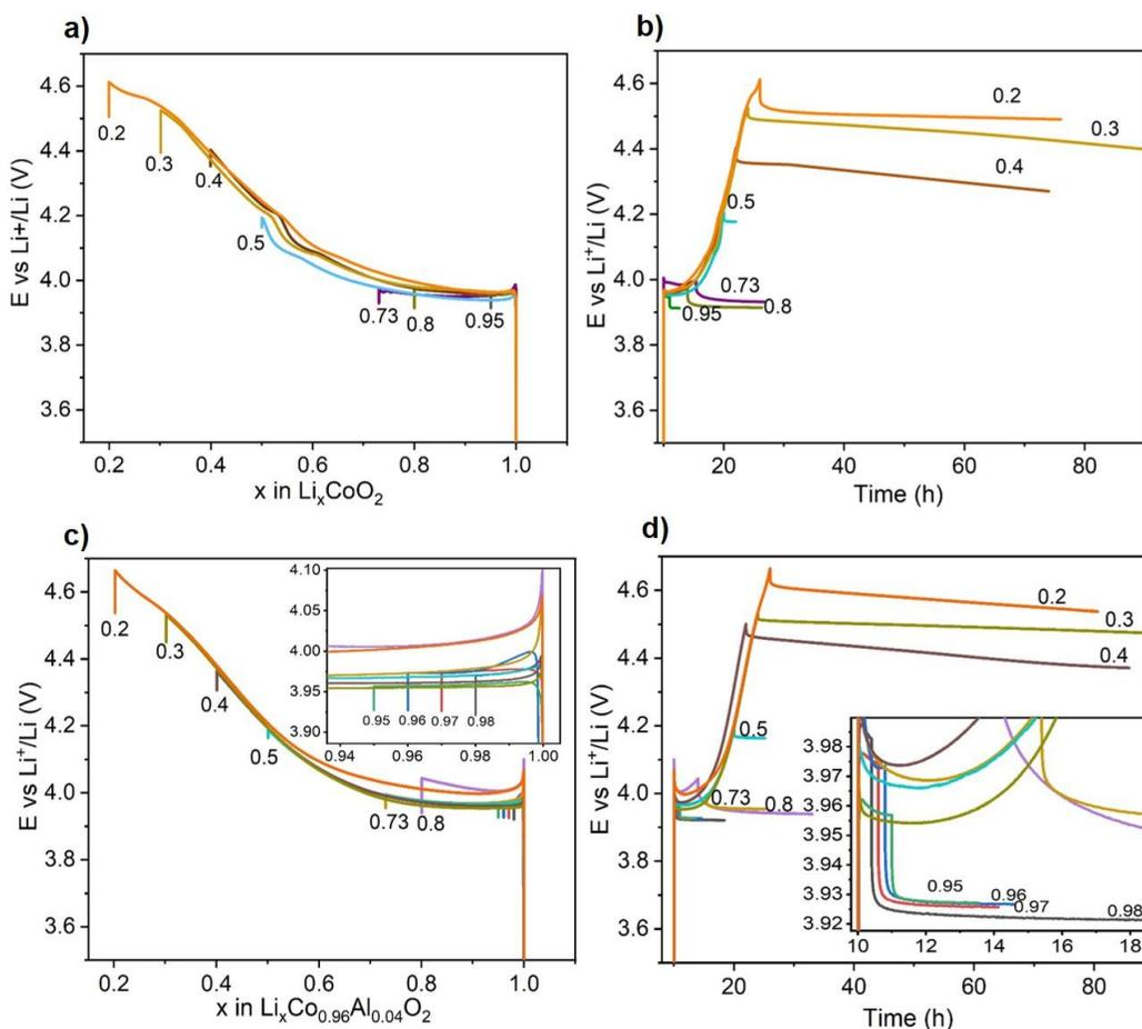
Figure A. 22. Galvanostatic charge of Li/ Li<sub>x</sub>MO<sub>2</sub> cells used to prepare the various a, b) Li<sub>x</sub>CoO<sub>2</sub> and c, d) Li<sub>x</sub>Co<sub>0.96</sub>Al<sub>0.04</sub>O<sub>2</sub> phases (C/20 rate).
