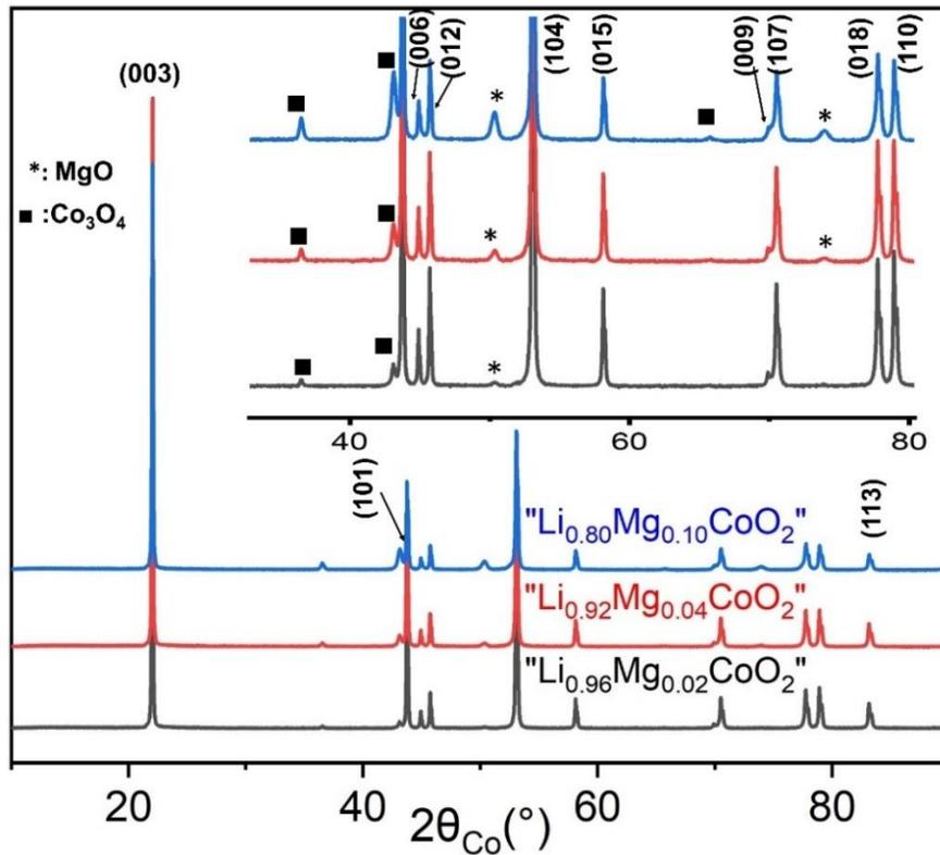
Figure B. 10. X-ray powder diffraction patterns for " $\text{Li}_{1-2y}\text{Mg}_y\text{CoO}_2$ " with  $y = 0.02, 0.04$  and  $0.10$ . The study carried out from the X-ray diffraction is recorded under the following conditions:  $10-120^\circ 2\theta$ , with a step of  $0.02^\circ$ .
