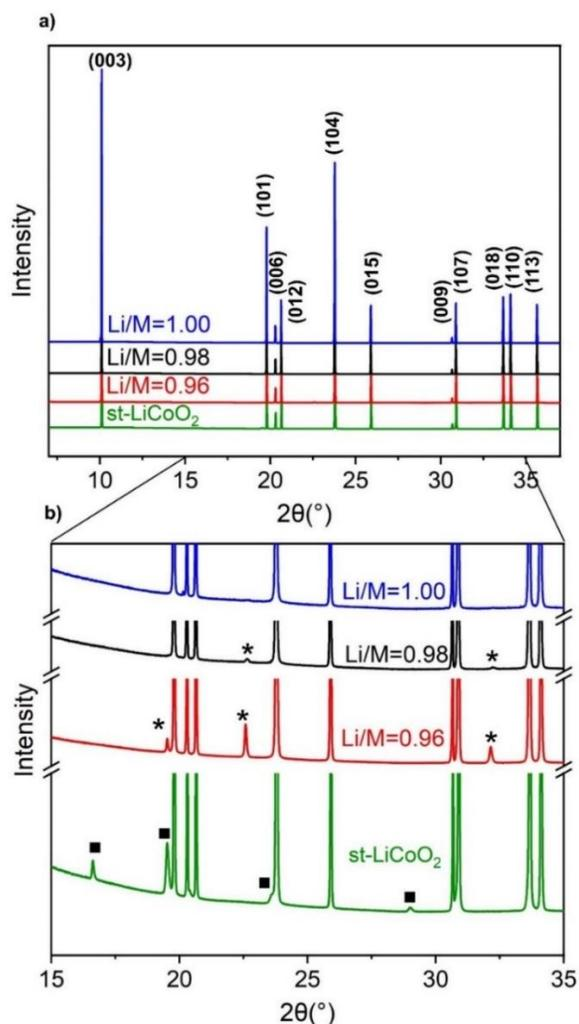
Figure B. 3.a) Synchrotron X-ray powder diffraction patterns for 2% Mg doped  $\text{LiCoO}_2$  compared with stoichiometric  $\text{LiCoO}_2$ . All the patterns were collected with  $\lambda = 0.8260 \text{ \AA}$ . A zoom in the b)  $15^\circ$  to  $35^\circ$  region is given (■:  $\text{Co}_3\text{O}_4$ ; \*:  $\text{MgO}$ ).
