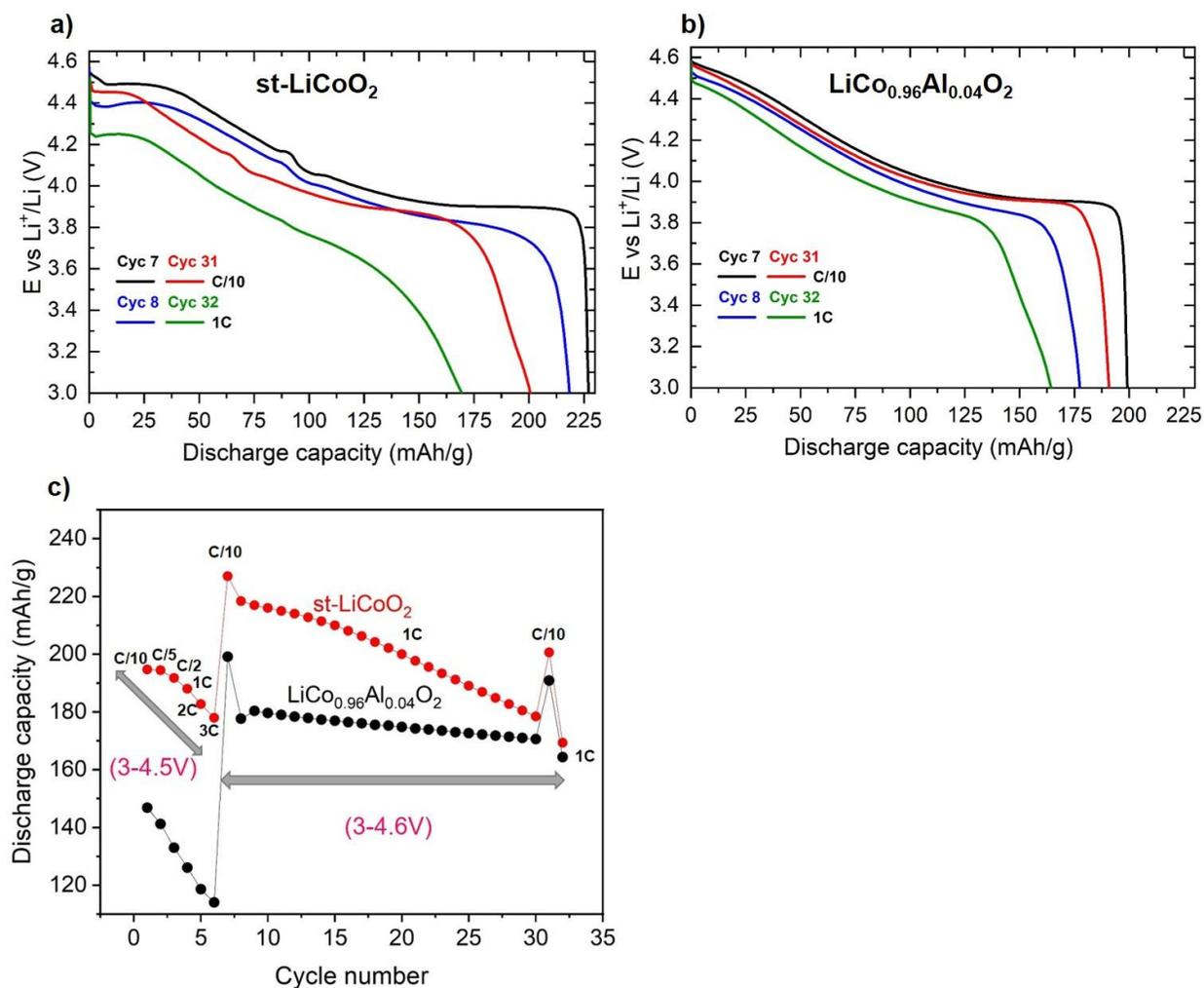
Figure A. 21. Discharge profiles (3V-4.6V) of Li//LiMO<sub>2</sub> (M=Co, Al) cells observed for the 7, 8, 31 and 32<sup>th</sup> cycles of a) *st*-LiCoO<sub>2</sub> and b) LiCo<sub>0.96</sub>Al<sub>0.04</sub>O<sub>2</sub>. c) The discharge capacity versus cycle number of *st*-LiCoO<sub>2</sub> and LiCo<sub>0.96</sub>Al<sub>0.04</sub>O<sub>2</sub> using different C rates.
