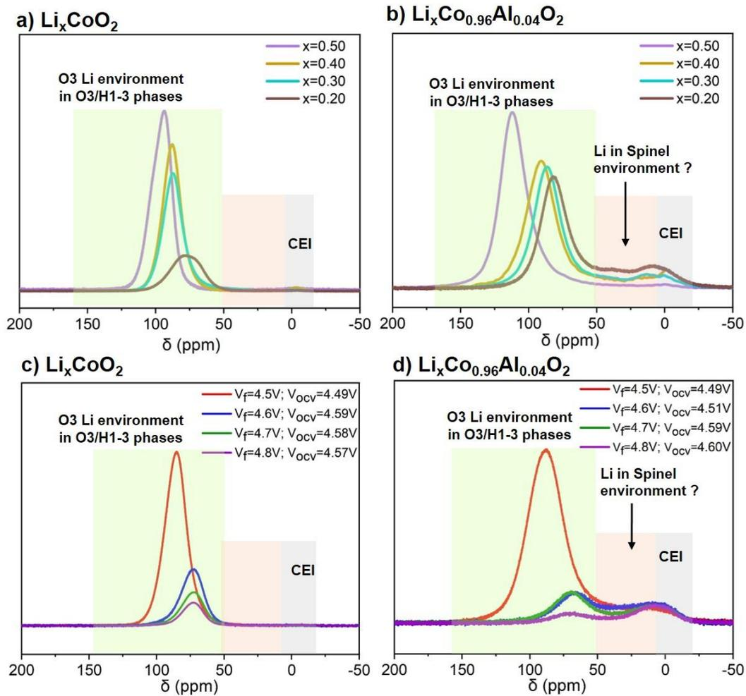
Figure A. 28. Comparison of  $^7\text{Li}$  MAS NMR for highly deintercalated phases of a)  $\text{Li}_x\text{CoO}_2$  and b)  $\text{Li}_x\text{Co}_{0.96}\text{Al}_{0.04}\text{O}_2$  with fixed Li contents of c)  $\text{Li}_x\text{CoO}_2$  and d)  $\text{Li}_x\text{Co}_{0.96}\text{Al}_{0.04}\text{O}_2$  with fixed floating voltages. The ex-situ NMR spectra intensities were normalized with respect to the number of mass of the electrode powder filled in the rotor and number of scans.
