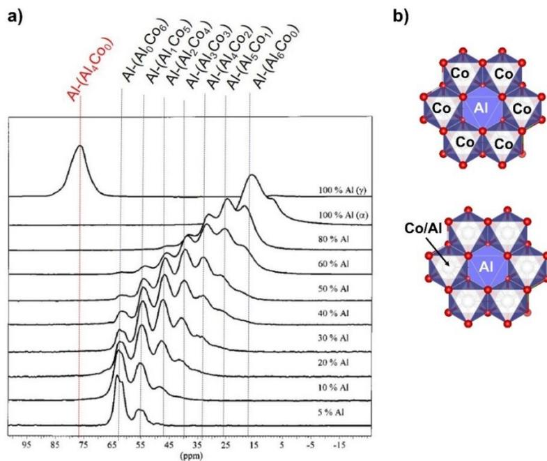
Figure A. 7.  $^{27}\text{Al}$  NMR spectra reported by Gaudin *et al.*<sup>25</sup> with b) a schematic representation of Al environments
