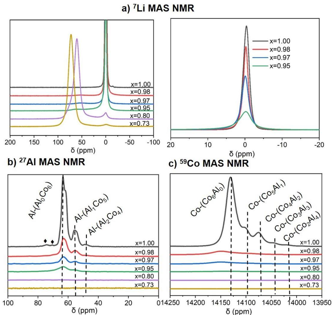
Figure A. 27. Ex-situ a)  $^7\text{Li}$  b)  $^{27}\text{Al}$  and c)  $^{59}\text{Co}$  MAS NMR of the deintercalated  $\text{Li}_x\text{Co}_{0.96}\text{Al}_{0.04}\text{O}_2$  by controlling the Li content in the low voltage region ( $\blacklozenge$ : satellite transitions).
