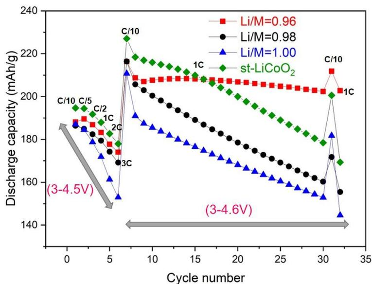
Figure B. 14. Cycling performances of st-LiCoO<sub>2</sub> compared to Mg doped LiCoO<sub>2</sub> with various Li/M ratios using different C rates.
