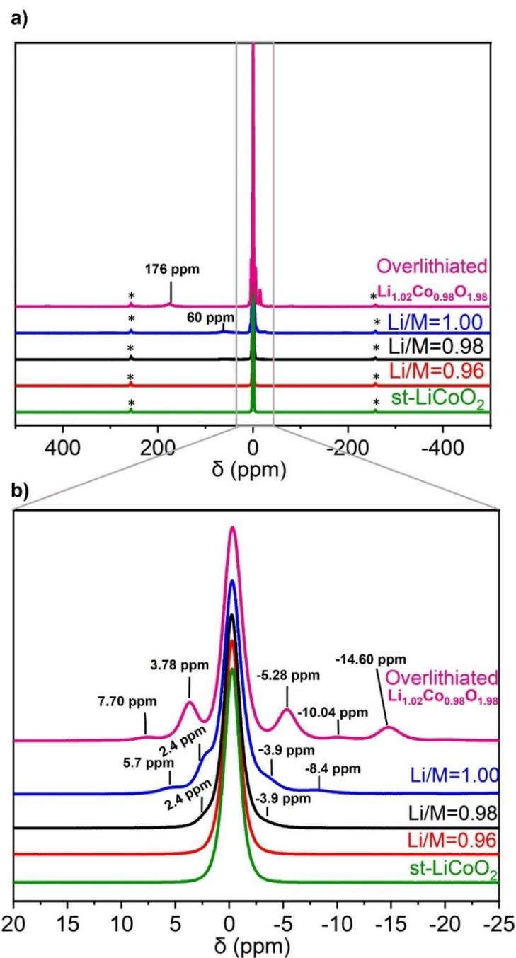
Figure B. 5.(a)  $^7Li$  MAS NMR spectra of 2% Mg doped  $LiCoO_2$  samples with various Li/M stoichiometries (rotor-synchronized Hahn echo sequence,  $\nu_R=30kHz$ ,  $B_0=7.05T$  \*: spinning sidebands) compared to st- $LiCoO_2$  (prepared with Li/Co = 0.98) and overlithiated  $Li_{1.02}Co_{0.98}O_{1.98}$  and (b) zoom in the region ( $-25 ppm \leq \delta \leq 20 ppm$ ).
