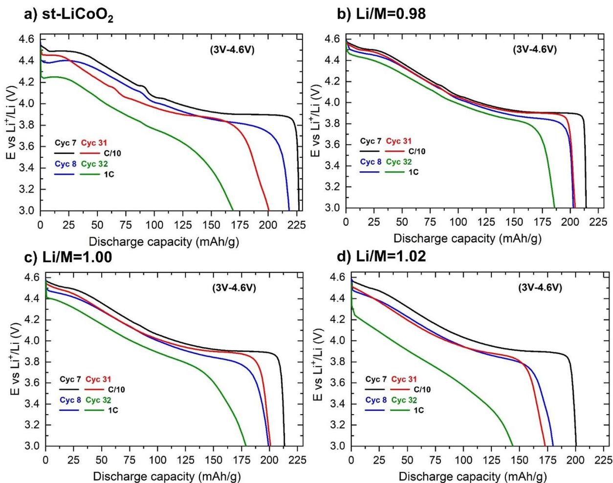
Figure A.14. Discharge profiles (3V-4.6V) of  $\text{Li}/\text{Li}_x\text{Co}_{0.98}\text{Al}_{0.02}\text{O}_2$  cells observed for the 7, 8, 31 and 32<sup>th</sup> cycles using C/10 and 1C rates compared to st-LiCoO<sub>2</sub>.
