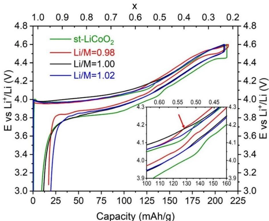
Figure A.13. First cycle for 2% Al doped  $\text{LiCoO}_2$  at C/20 as positive electrode in  $\text{Li}/\text{Li}_x\text{Co}_{0.98}\text{Al}_{0.02}\text{O}_2$  compared to those of  $\text{st-LiCoO}_2$ . A zoom on the monoclinic transition is given in insert.
