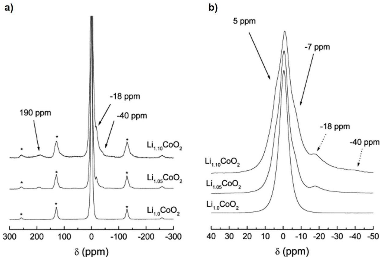
Figure 12.  ${}^7\text{Li}$  MAS NMR spectra for the various  $\text{Li}_x\text{CoO}_2$  phases with a zoom in the central transition given in b ( $x_0 = 1.0, 1.05$  and  $1.10$ ; \*:spinning sidebands).<sup>53</sup>
