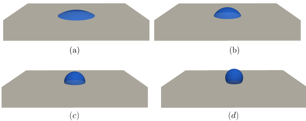
Figure 4.6: The shape of water droplets at equilibrium on a plane. (a) \theta = 30^\circ , (b) \theta = 60^\circ , (c) \theta = 90^\circ , and (d) \theta = 120^\circ .
