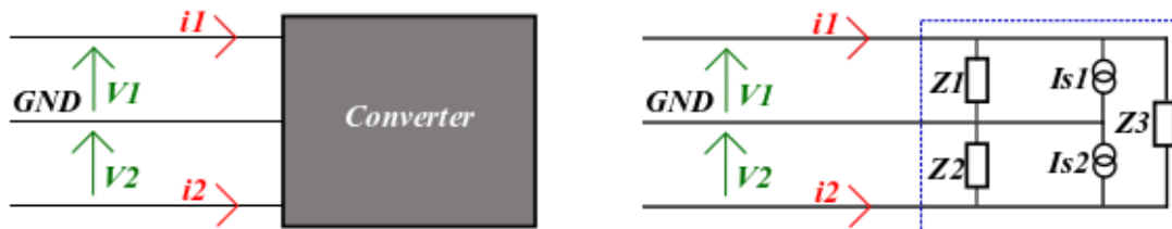
Figure 3.6 – Behavioural EMI modelling with 5 parameters (black box).
