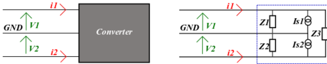
Figure 3.6 – Behavioural EMI modelling with 5 parameters (black box).
