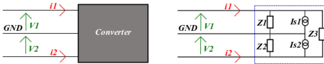
Figure 3.6 – Behavioural EMI modelling with 5 parameters (black box).
