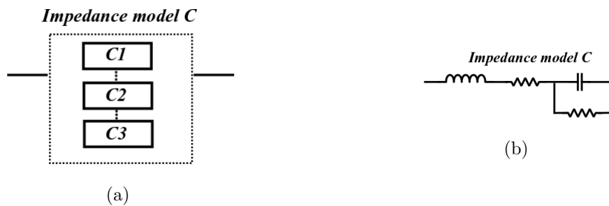
Figure 3.11 – Decoupling capacitors model (a) Capacitor impedance structure (b) equivalent series resistance and inductance model.
