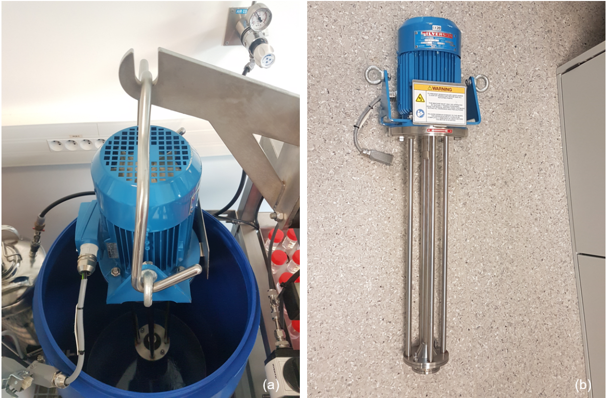
Figure 2.15: Silverson emulsifier with a dispersion head: (a) in the tank, (b) in full
