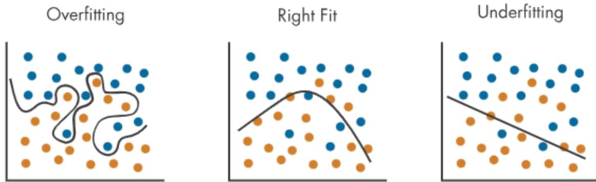
Figure 5: Illustration of overfitting, right fit, and underfitting of a classification model (reproduced from Surajestment (n.d.)).
