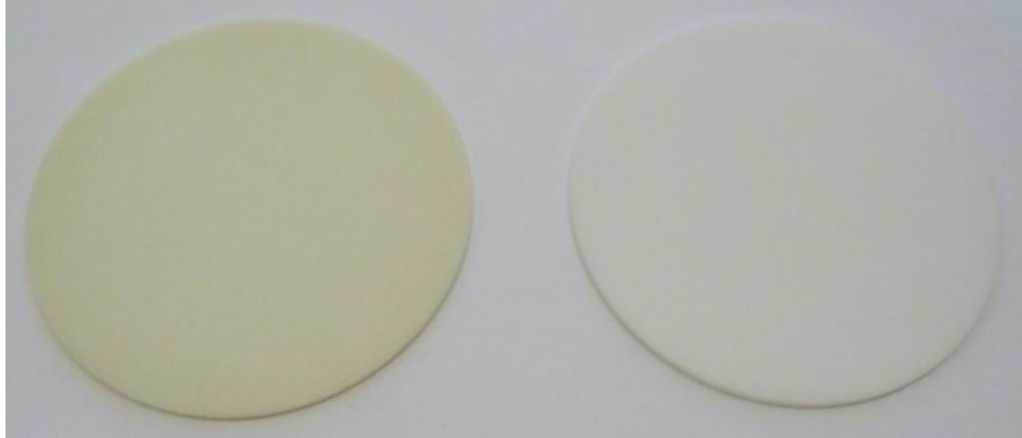
Figure 2.3. \alpha -aluminium oxide disc of supplier A (left) and supplier B (right).
