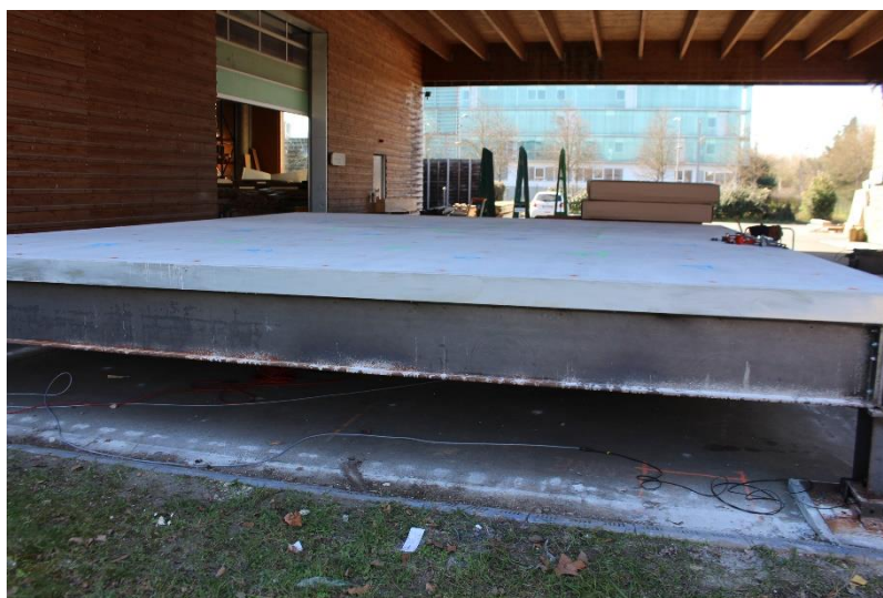
Figure 3.8: Side view of the floor specimen
