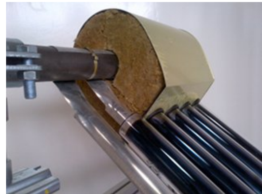
FIGURE 3.10 – SAED , liaison caloduc/tube acier
