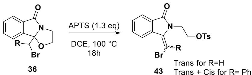
To a solution of compound **36** in dichloroethane, 1.3 eq of APTS was added. The mixture was heated at 100 °C for 18h. The solvent was evaporated. A purification on flash chromatography was performed to get the corresponding compounds **43b-c**.
