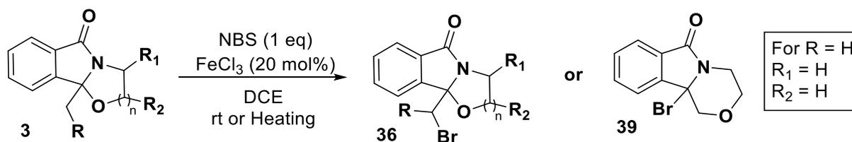
To a solution of oxazolidinone **3** (1 eq) in dichloroethane, NBS (1 eq) and  $\text{FeCl}_3$  (20 mol%) were added. The reaction mixture was heated or stirred at room temperature. After completion of the reaction as shown on TLC, the mixture was washed 3 times with a saturated solution of sodium bicarbonate. Organic layers were dried on  $\text{MgSO}_4$ , and the solvent was evaporated.
