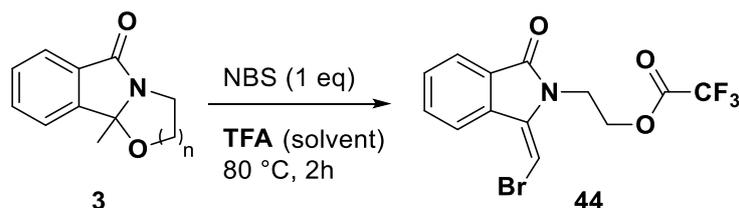
To a mixture of the corresponding compound **3**, NBS (1 eq) was added. The mixture was heated at 80 °C for 2 hours. TFA was evaporated, and a purification on flash chromatography was performed to get the corresponding compound **44**.
