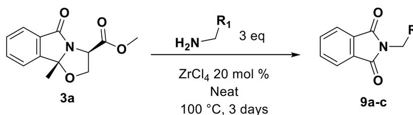
Compound oxazolidinone **3a** (1 eq) and correspondent benzylamine (3 eq) were mixed together, 20 mol%  $\text{ZrCl}_4$  was added and the mixture was heated at 100 °C for 3 days. The mixture was filtered through a pad of celite and purified on flash chromatography to afford compounds **9a-c**.
