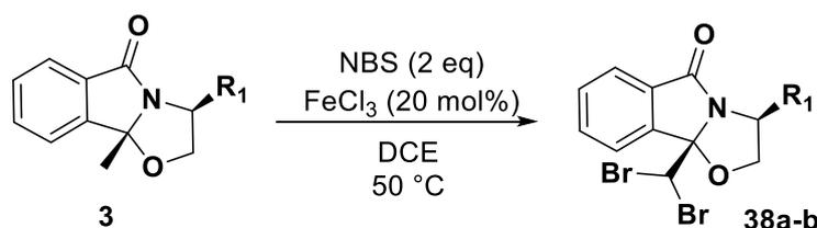
To a solution of oxazolidine **3** (1 eq) in dichloroethane, NBS (2 eq) and  $\text{FeCl}_3$  (20 mol%) were added. The reaction mixture was heated at 50 °C for 18h. The mixture was washed 3 times with a saturated solution of sodium bicarbonate. Organic layers were dried on  $\text{MgSO}_4$ , and the solvent was evaporated. A purification on flash chromatography was performed to get the corresponding *N,O*-acetals **38a-b** dibrominated.
