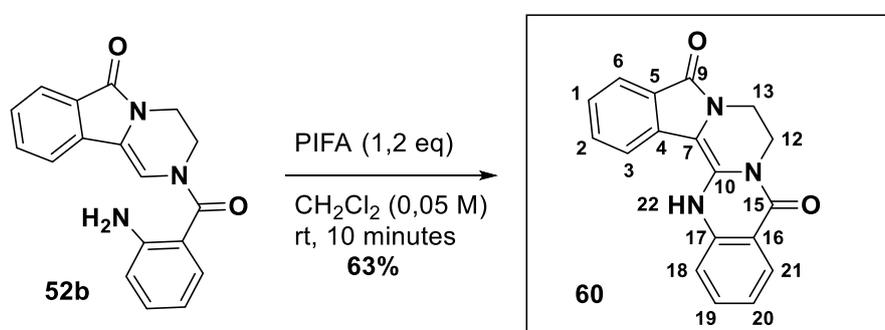
To a solution of piperazine **52b** in dichloromethane (0.05M), 1.2 eq of Iodosobenzene bis(trifluoroacetate) (PIFA) were added. The reaction was stirred at room temperature for 10 minutes. The mixture was filtered through celite and purified on flash chromatography to get compound **60** as a white solid.
