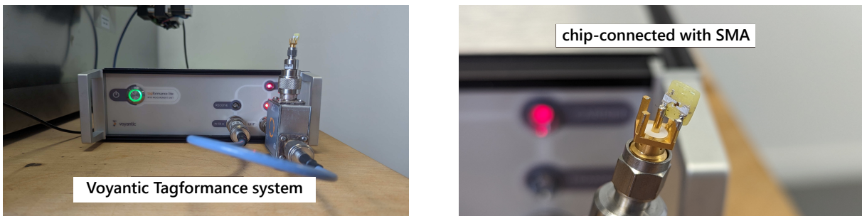
Figure 2.2: Experimental setup to measure the threshold of the chip, connected with SMA.
