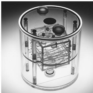
FIGURE 2.15 – Fantôme Magphan SMR 170 (The Phantom Laboratory)
