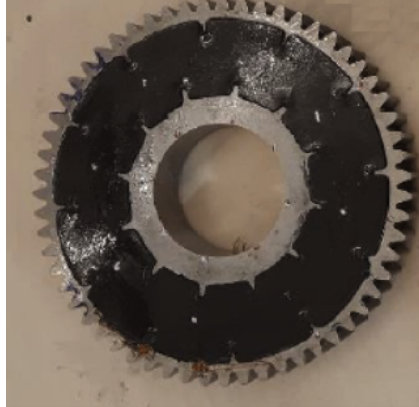
Figure 1.12: Material lightweight gear: CFRP configuration
