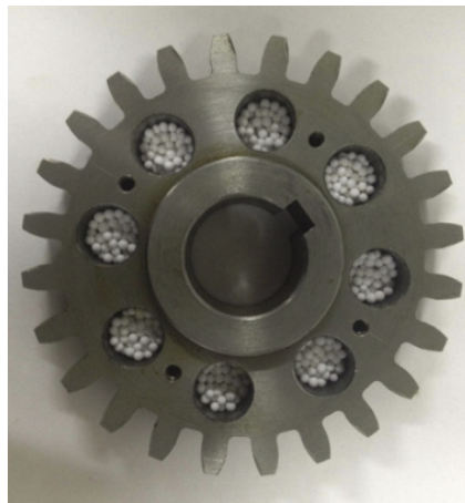
Figure 1.14: Geometrical and Material lightweight gear: Damping powder-filled configuration
