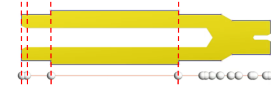
Figure 3.1: Visual representation of a non-uniform shaft and its corresponding FE Timoshenko beam model. Each element corresponds to a geometrically simple region.
