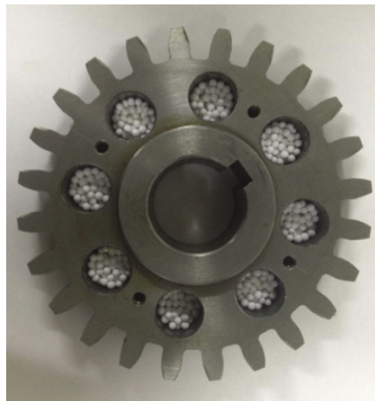
Figure 1.14: Geometrical and Material lightweight gear: Damping powder-filled configuration
