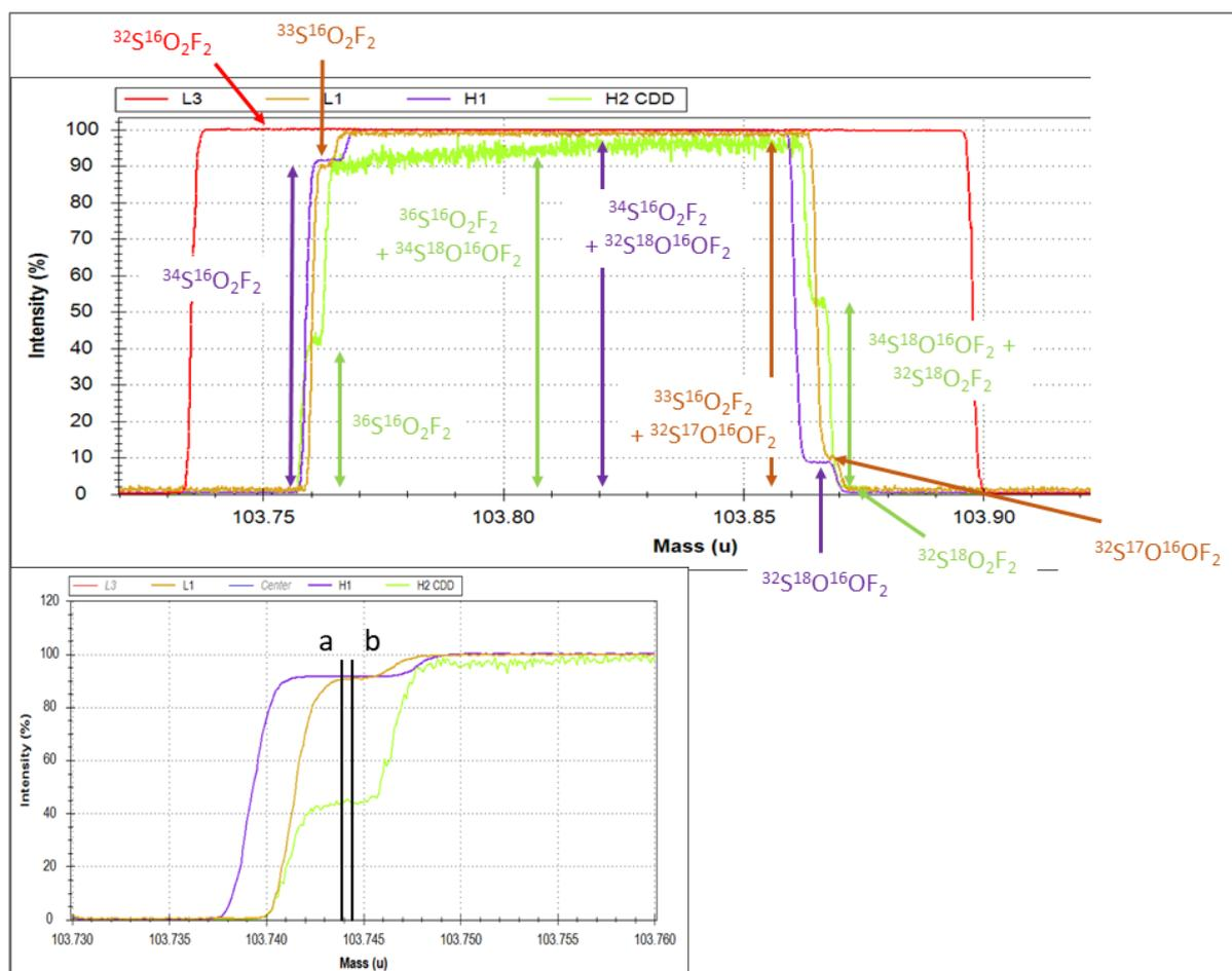
Figure 3.8: Mass-scan on the Ultra-HR-IRMS for analysis of the four S isotopes in  $\text{SO}_2\text{F}_2$ . Top panel: the peak shapes recorded by the four cups are described according to the different  $\text{SO}_2\text{F}_2$  isotopologue they receive. Bottom panel: zoom on the left peak shoulder where the four S-masses are measured at the same time. Each analysis successively measures the “number of counts” on ‘a’ and ‘b’ positions (see text).
