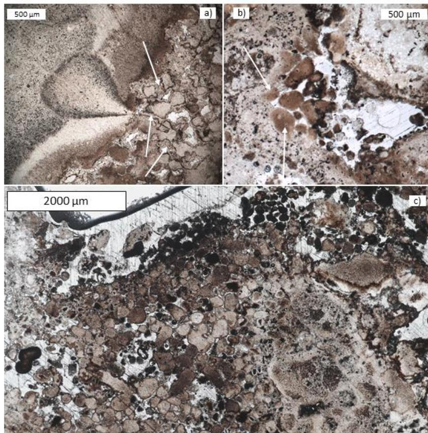
Figure 9.6: Photographs of agglutinating hydromagnesian peloids at the edge of white microbialites in Alchichica, seen under plane-polarized light. a) View of AL-R-1 with evidence of past fluid circulation and cementation around hydromagnesite grains (white arrows). b) View of AL-R-5 with incorporation of hydromagnesian peloids within the microbialites surface (white arrows). c) Similar processes seen in AL-R-3.
