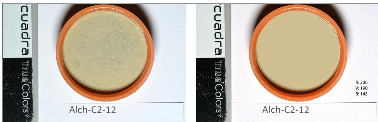
Figure 3.5: Photographs of the sediment preparation for sediment color characterization before (left) and after (right) correction with the black and white color scale. On the right, the disk in the middle of the lid represents the sediment average color with RVB values on the right.
