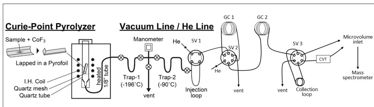
Figure 3.7: Scheme of the SF<sub>6</sub> purification line, modified after Ueno *et al.* (2015). 'GC' stands for gas chromatography; 'SV' for switching valve and 'CVT' for continuously variable transmission and refers to a manometer measuring both high and low pressures.
