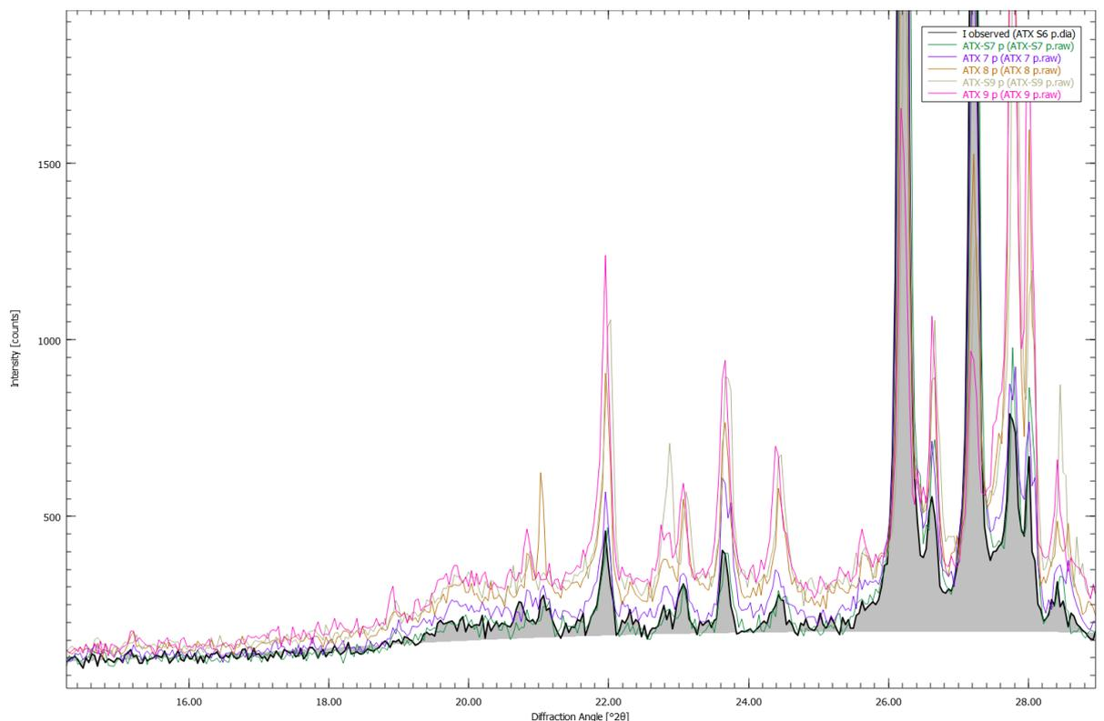
Figure 6.20: Zoom in diffractograms of sediment from Lake Atexcac (10-22 cm). The abscissa axis represents the  $2\theta$  angle of diffraction and the ordinate axis the number of counts. There is a progressive re-appearance of Mg-silicates (at  $\sim 20^\circ$ ) starting from ATX-7 in purple (16-18 cm in depth) to ATX-9 in dark green (18-20 cm in depth), after which the corresponding bump remains. On the left, where there are no peaks the background signal is similar for all samples.
