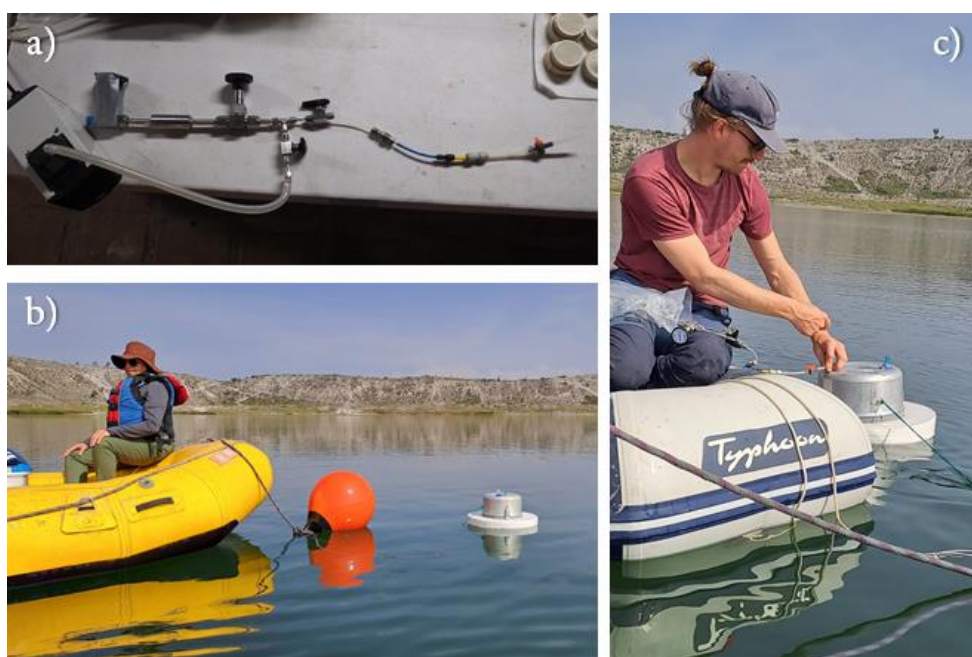
Figure 3.4: pictures of the gas collection set-up on the field. a) pumping of the plastic tube part on the right side, before sampling. The stainless steel tube on the left part was pre-vacuumed in the laboratory in France. b) placement of the gas accumulation chamber on La Preciosa's surface with R. Tavera. c) collection of the gases after two days of accumulation by replacing the plugs on the lid and connecting the tubing system to the chamber instead.
