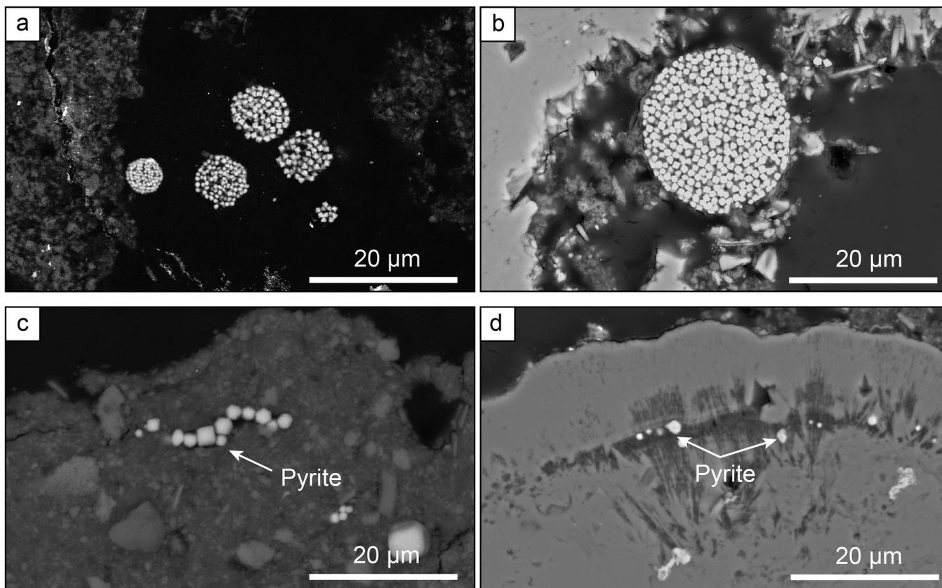
**Figure 1** Secondary Electron microscopy pictures of (a, b) framboidal pyrites and (c, d) micropyrates from (a, c) Cayo Coco Lagoon and (b, d) Atexcac. Framboidal pyrites are located at the surface of the mineralised microbialite (in dark) while micropyrates are entombed within aragonite (in light grey) or Mg rich silicate (dark grey).
