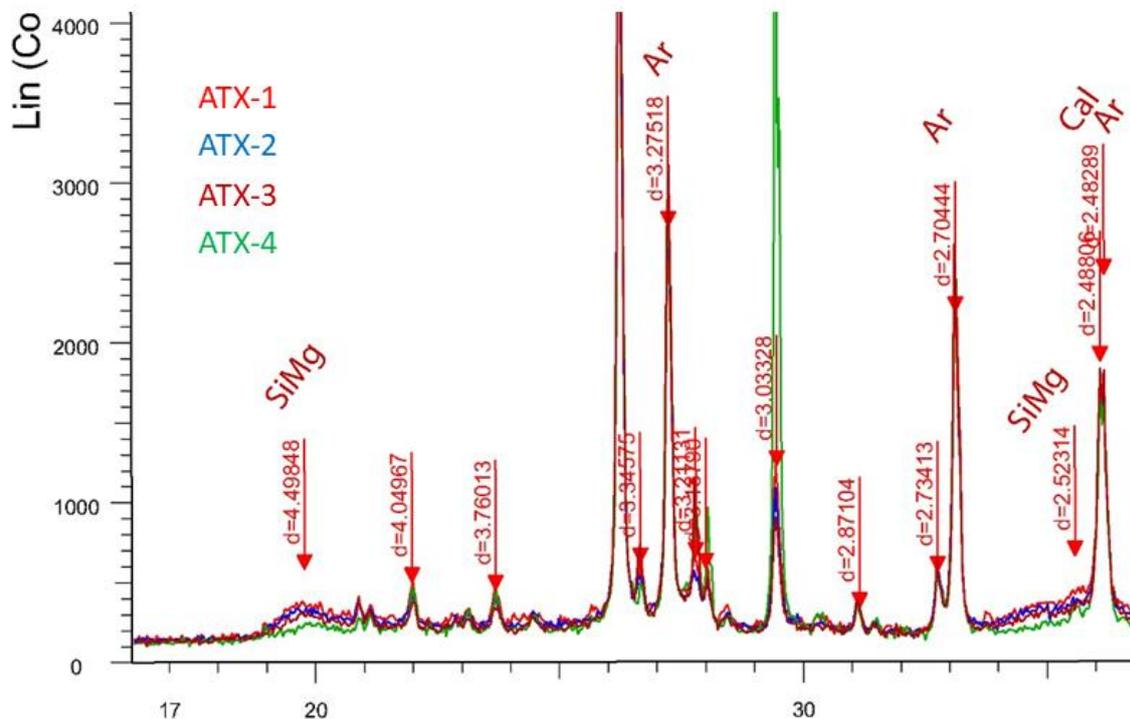
Figure 6.19: Zoom in diffractograms of sediment powders from Lake Atexcac (0-9 cm). The abscissa axis represents the  $2\theta$  angle of diffraction and the ordinate axis the number of counts. ‘SiMg’, ‘Ar’ and ‘Cal’ refer to authigenic Mg-silicate phases (see text), aragonite and calcite, respectively. There is a progressive disappearance of Mg-silicates between ATX-1 in light red (0-1 cm in depth) and ATX-4 in green (7-9 cm in depth).
