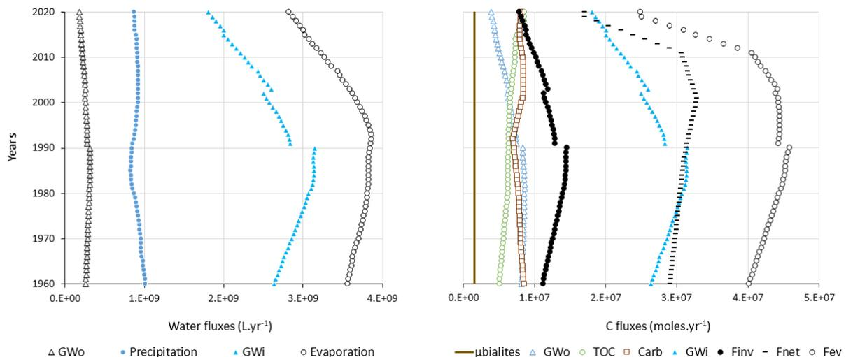
Figure 5.4: water and C fluxes in scenarios 1. In scenarios 2 and 3, a flux of  $30 \cdot 10^6 \text{ mol.yr}^{-1}$  of respired- or volcanic- $\text{CO}_2$  is added. It changes the  $^{14}\text{C}$  balance of the lake such that calculated  $F_{\text{ev}}$  and  $F_{\text{inv}}$  are slightly different as well.
