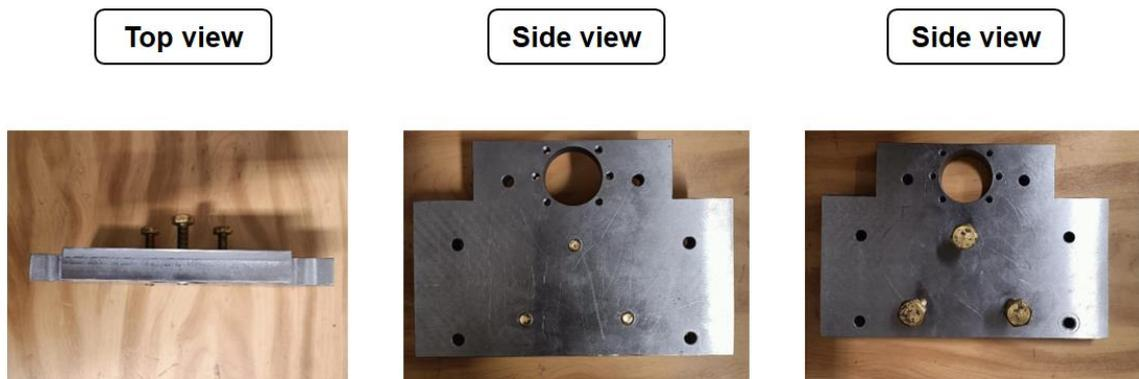
*Figure 23: The magnetic support piece composed of magnetic inox material and have three nonmagnetic screws for collecting the first magnet.*
