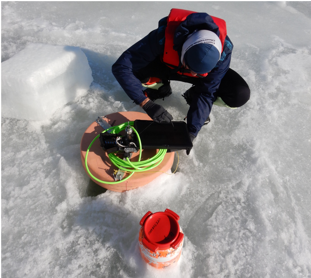
Figure 2.5 – Example of one wave buoy (bottom) and one ADCP (center) deployed on the same floe in the pack ice region on day 2020-02-25, while I am programming the ADCP.
