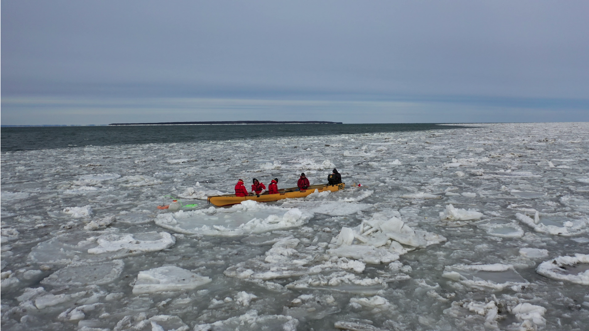
Figure 2.2 – Picture taken by a UAV facing North of the ice canoe in operation and its five-member crew during the 2020-02-13 deployment off the BdHH, with Bic Island visible in the back. The pink, red and green objects on the ice floe just to the left of the canoe are respectively the buoy of S497, a SKIB buoy, and the digital cable connecting S497 to a computer to start the data acquisition.
