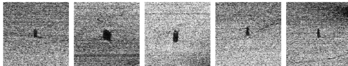
Figure 2.9: Image credits: [70]. Different underwater rocks detected by a side-scan sonar. We can notice the difficulty in distinguishing one feature from the other.
