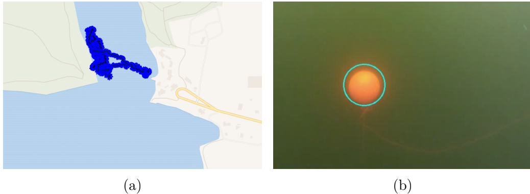
Figure 7.14: (a): Display of the area already explored on the HMI that would guide the planning of new missions when searching for the submerged buoy; (b): Detection of the orange buoy by the underwater camera.
