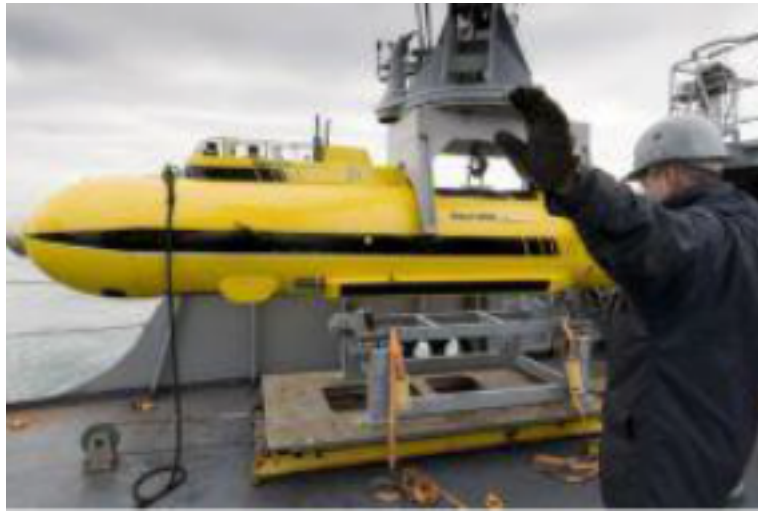
Figure 1.6: Image credits: DGA/GESMA. Deployment of the AUV Daurade in the roadstead of Brest from a ship.
