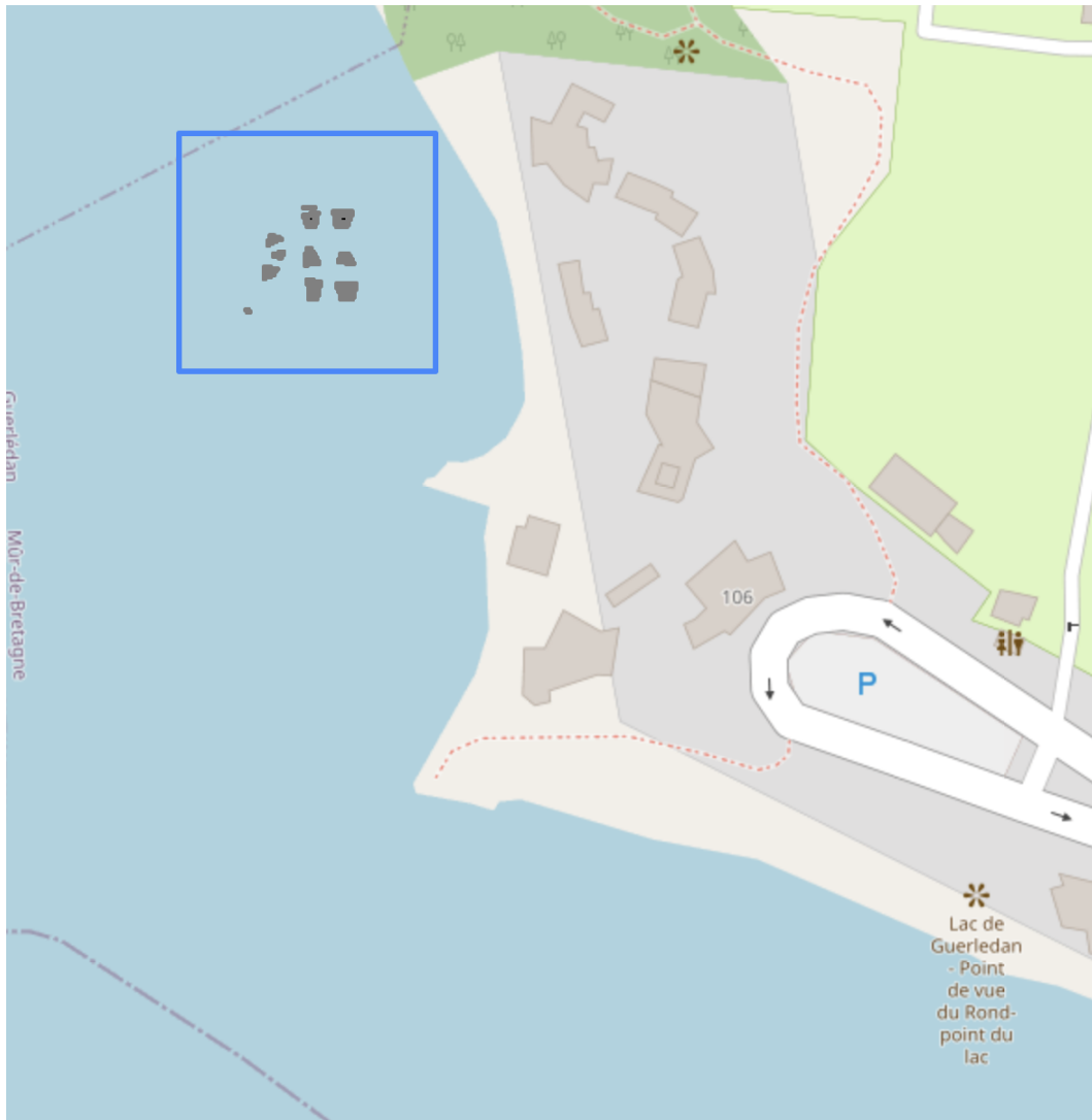
Figure 7.21: Georeferenced representation of the area explored four times on the Guerledan map. The initial knowledge about the positioning of the yellow brick was that it was inside the area surrounded by the blue rectangle. Using the coverage measure estimation this area is contracted to the areas represented in grey on the lake.
