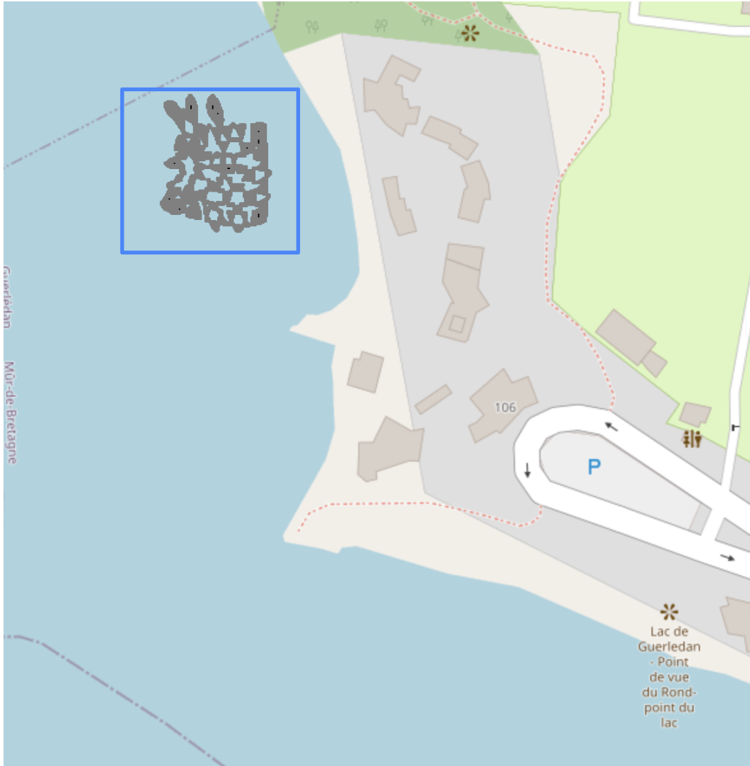
Figure 7.20: Georeferenced representation of the area explored twice on the Guerlédan map. The initial knowledge about the positioning of the red brick was that it was inside the area surrounded by the blue rectangle. Using the coverage measure estimation this area is contracted to the areas represented in grey on the lake.
