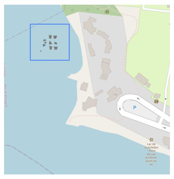
Figure 7.21: Georeferenced representation of the area explored four times on the Guerlédan map. The initial knowledge about the positioning of the yellow brick was that it was inside the area surrounded by the blue rectangle. Using the coverage measure estimation this area is contracted to the areas represented in grey on the lake.
