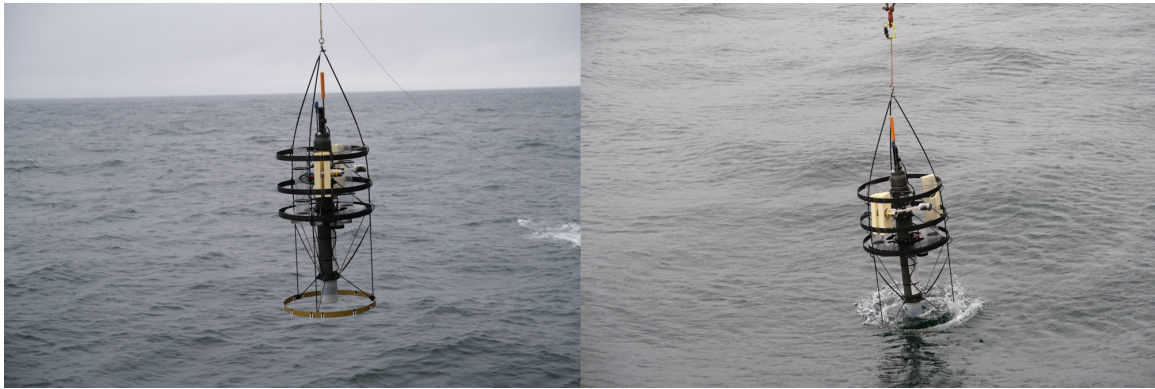
Figure 4.13: Deployment of the Twilight Zone Explorer float during the APERO cruise.
