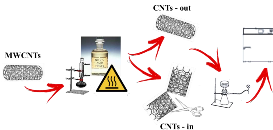
Figure 1. Scheme of pretreatment of CNTs.
