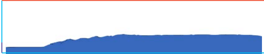
Figure 4.27: Numerical setup of the hydraulic jump. Off plane boundaries are symmetries, on the bottom left-hand side is the inlet, red denotes a pressure outlet and light blue a wall.
