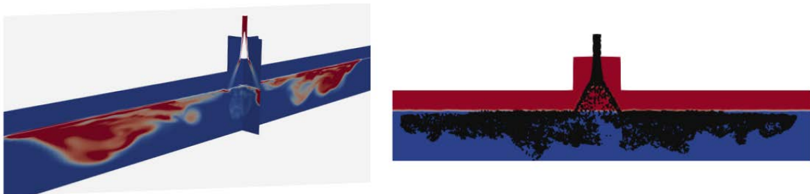
Figure 1.10: Differences in modelling between multifluid (left) and multifluid-Lagrangian tracking (right) methods for liquid-gas-solid flows. Cases presented in chapter 5.
