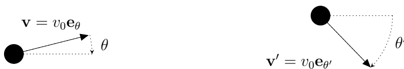
Figure 3.1.: A particle with orientation \theta travels ballistically with a velocity \mathbf{v} = v_0 \mathbf{e}_\theta = v_0 (\cos \theta, \sin \theta) . It undergoes a tumbling event at a rate \lambda . As the particle tumbles, its orientation is updated to \theta' = \theta + \theta_{\text{jump}} where \theta_{\text{jump}} is drawn in [-\pi, \pi) according to the distribution P_t .
