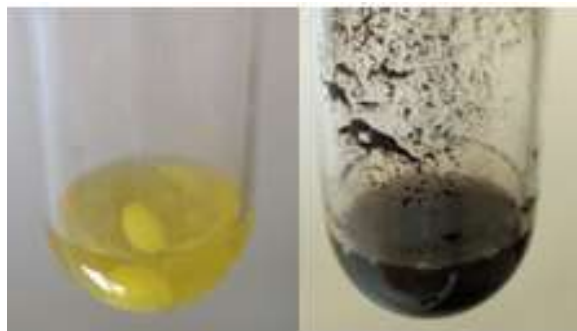
Figure 1: Colour change in a typical synthesis of RuNi/PVP NPs at RT; left, before the hydrogenation reaction, and right, after the reaction.
