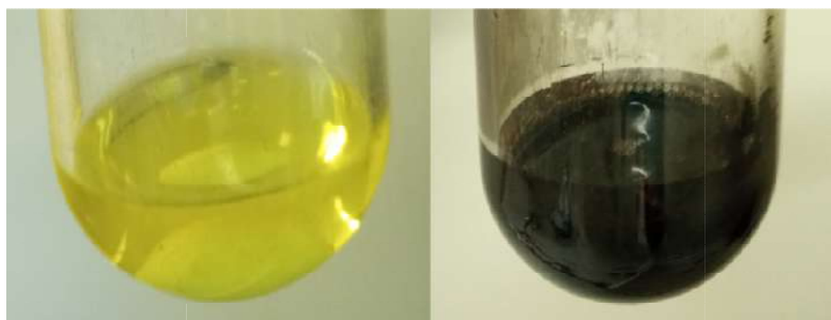
Figure 35: Colour change observed in a typical synthesis of RuNi/AdCOOH NPs at 85 °C; left, before the hydrogenation reaction, and right, after the reaction.
