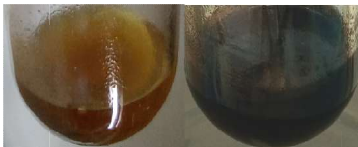
Figure 39: Colour change observed in a typical synthesis of RuCu/PVP NPs at 100 °C; left, before the hydrogenation reaction, and right, after the reaction.
