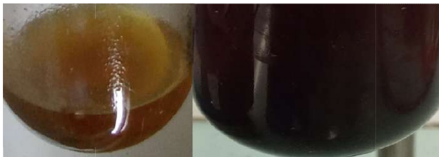
Figure 52: Colour change in a typical synthesis of Cu/HDA NPs at 80 °C, 100 °C or 120 °C; left, before the hydrogenation reaction, and right, after the reaction.
