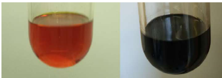
Figure 21: Colour change in a typical synthesis of RuNi/PPh 2 Py NPs at 85 °C; left, before the hydrogenation reaction, and right, after the reaction.
