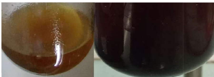
Figure 52: Colour change in a typical synthesis of Cu/HDA NPs at 80 °C, 100 °C or 120 °C; left, before the hydrogenation reaction, and right, after the reaction.
