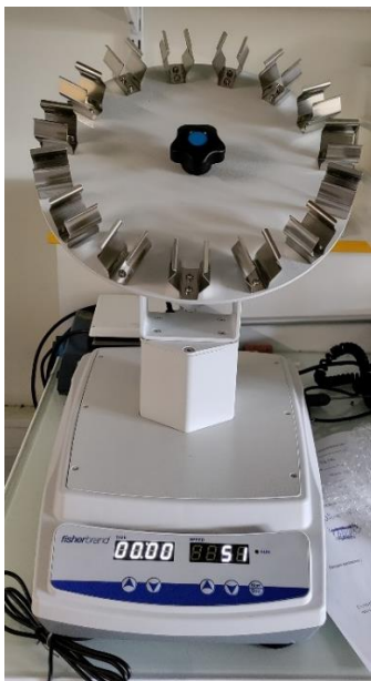
Figure 4.3 Rotating instrument used to stirrer the [\text{Ni}(\text{COD})_2]/\text{THF}/\text{FIL} reaction mixtures.
