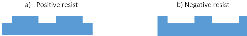
Figure 112. Sketch of the sample after etching. a) In the case of positive resist. b) In the case of negative resist.
