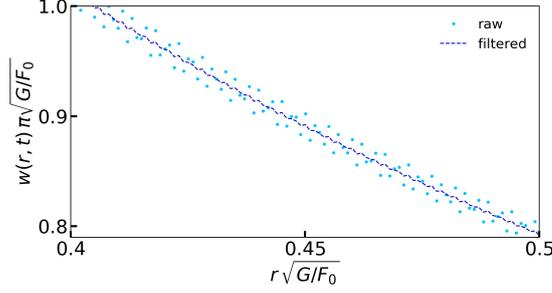
FIG. C.1. **Effect of a Savitsky-Golay filter of order 3.** A Savitsky-Golay filter of order 3 is applied on a 9-points wide sliding window, for a total of 200 000 points.
