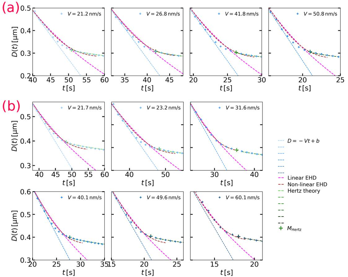
FIG. B.1. **Zoom around the inflection point in distance-time representation.** Distance  $D$  between the two glass interfaces as a function of time, zoomed around the inflection point, for each of the ten approach curves shown in the Chapter 5. (a): First data set, made of four curves. (b): Second data set, made of six curves.
