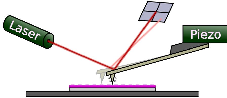
FIG. 2.3. **Schematic of an AFM.** A sharp tip is held by a cantilever, which is supported by a chip. A piezo element moves vertically the chip, whose position is noted  $z_{\text{piezo}}$ . A laser beam is sent on the top face, at the edge of the cantilever. The reflection of the laser is monitored by a photodiode. From the shifted signal of the photodiode, the deflection of the cantilever  $Z_{\text{canti}}$  is extracted.
