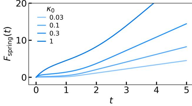
FIG. 5.10. **Theoretical force when only a spring is considered.** Dimensionless theoretical force  $F_{\text{spring}}$  as a function of dimensionless time  $t$ , computed from Eq. (5.57), for different values of the ratio between viscous stresses and spring elasticity  $\kappa_0$ , as indicated in the legend, and for  $\delta(0) = 0$ .
