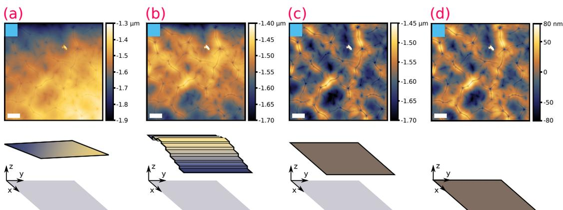
FIG. A.1. **Treatment of raw AFM images.** Image at different steps of treatment and schematic of the defect to correct. (a): Raw image obtained after a topography measurement. (b): After correction of the planar tilt. (c): After correction of the gap between successive lines. (d): After subtracting the mean plane.
