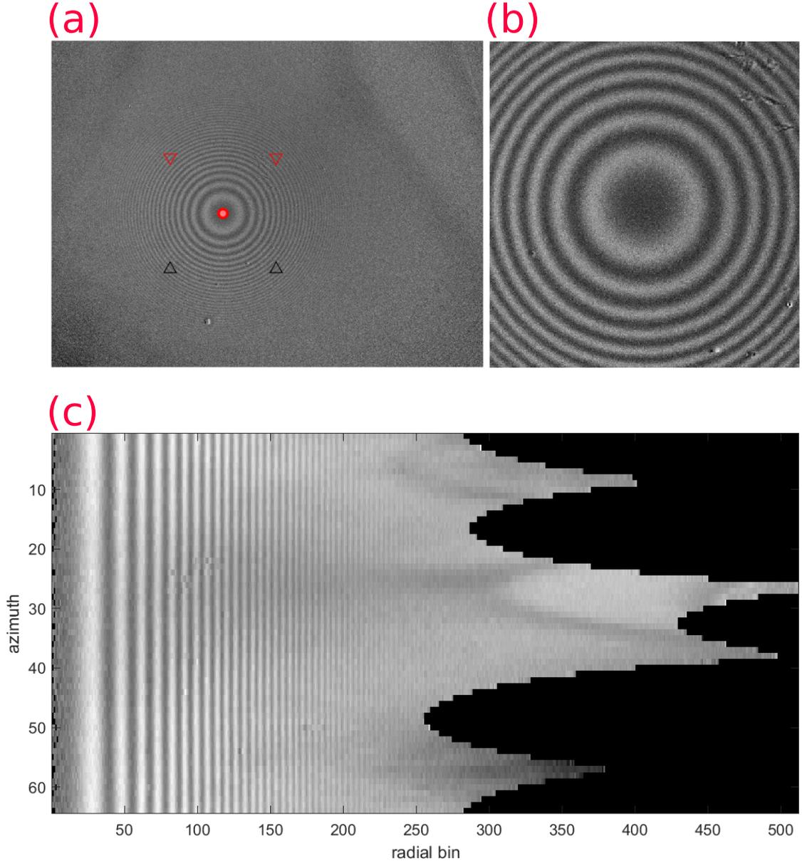
FIG. A.7. **Numerical search for the center of the Newton's rings.** (a): Large plan of an interference image, after division by the background image. (b): Zoom on the center of the rings. (c): Conversion of the image into polar coordinates. The light intensity is plotted as a function of the radial coordinate  $r$  (horizontal axis) and the azimuths  $\theta$  (vertical axis).
