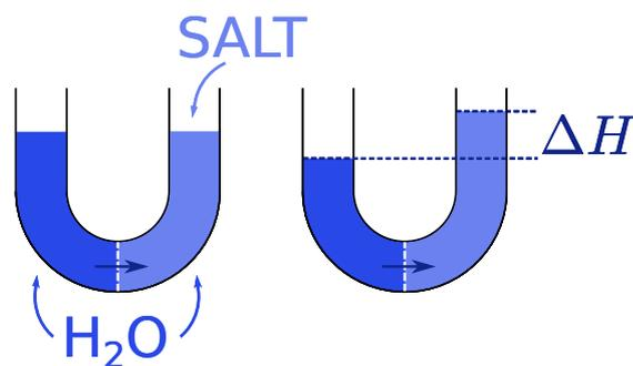
FIG. 1.3. **Intuitive definition of the osmotic pressure.** A U-pipe is filled with water. Salt is added on the right side. A semi-permeable membrane placed in the middle allows water to flow but prevents salt to pass through. A water flow from left to right dilutes the salt, and results in a difference of height  $\Delta H$  between the two sides.
