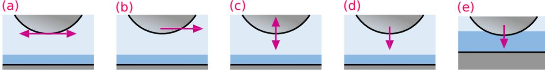
FIG. 1.8. **Different configurations for soft-lubrication investigation in the sphere-plane geometry.** The sphere motion is (a): oscillatory and parallel to the soft-coating plane, (b): steady and parallel to the plane, (c): oscillatory and perpendicular to the plane, (d): steady and perpendicular to the plane, also called approach mode. (e): After the approach mode, the sphere is eventually in solid contact with the soft coating and indents it.
