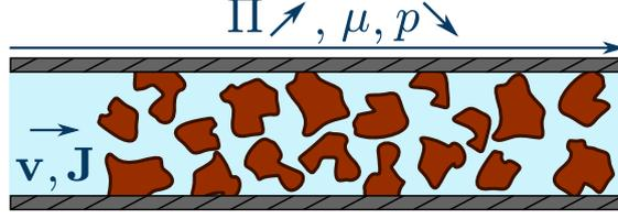
FIG. 1.4. **Darcy flow through a porous medium.** A solvent flows through a porous medium at a velocity  $\mathbf{v}$ , or similarly with a molecular flux  $\mathbf{J}$ , following the decreasing mechanical pressures  $p$  or chemical potentials  $\mu$ , or the increasing osmotic pressures  $\Pi$ .
