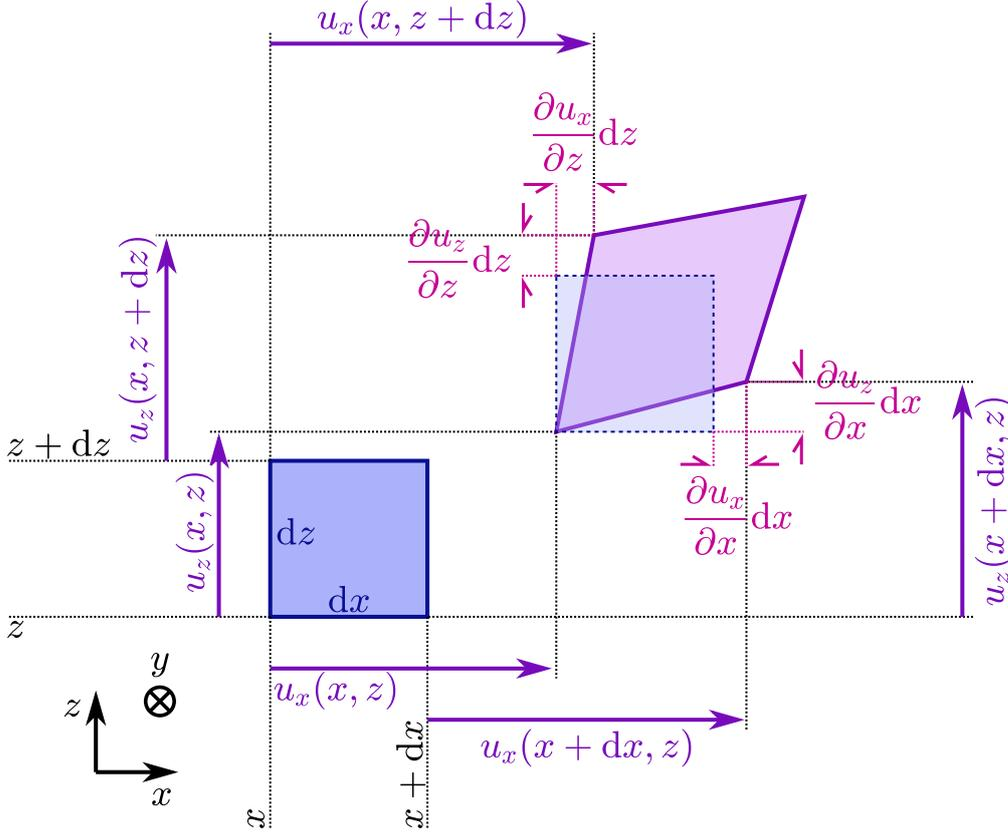
FIG. 1.6. **Two-dimensional displacement of an infinitesimal surface element upon deformation.** Originally located at a position  $(x, z)$ , an infinitesimal surface element  $dx dz$  is displaced by  $\mathbf{u}$  upon a deformation. The strain tensor  $\epsilon$  is computed using the partial derivatives of the displacement field  $\mathbf{u}$ , using Eq. (1.38).
