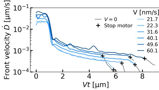
FIG. A.8. **Front velocity of the spherical probe in SFA.** From the data of Fig. 5.6(b), the time-derivative of the distance  $D$  between the two glass interfaces is computed and plotted as a function of  $Vt$ , the traveling distance imposed at the back of the spring.
