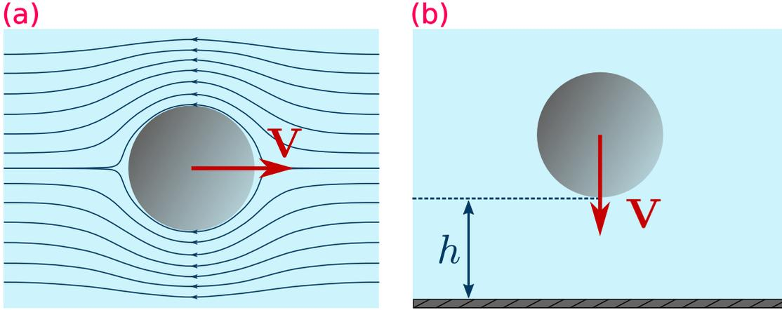
FIG. 1.2. **A spherical particle submitted to Stokes drag.** (a): A particle of radius  $R$  is moving at a velocity  $\mathbf{V}$  in a viscous fluid. The stream lines are drawn. (b): A particle of radius  $R$  is moving at a velocity  $\mathbf{V}$  towards a rigid boundary. The distance to the wall is denoted  $h$ .
