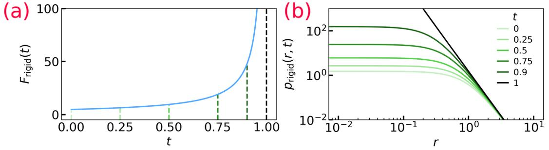
FIG. 5.9. **Theoretical force and pressure field in the rigid case.** (a): Dimensionless theoretical force  $F_{\text{rigid}}$  as a function of dimensionless time  $t$ , computed from Eq. (5.48). The green dashed lines indicate the times  $t$  at which the pressure is plotted in (b). (b): Dimensionless theoretical pressure field  $p_{\text{rigid}}(r, t)$ , computed from Eq. (5.47), for different dimensionless times  $t$ , signaled in (a) by green dashed lines.
