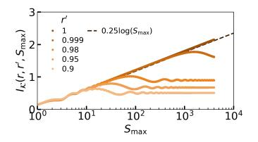
FIG. 5.11. Convergence of the kernel integral in SFA simulations. Truncated integral  $I_{\mathcal{K}}(r, r', S_{\max})$  of the product  $s\mathcal{G}_{\tau}^{\text{comp}}J_0(sr)J_0(sr')$  as a function of  $S_{\max}$ , as defined in Eq. (5.60), for different r', for r = 1,  $\nu = 0.2$  and  $\tau_0 = 1$ . For r = r', the integral diverges following a logarithmic scaling.
