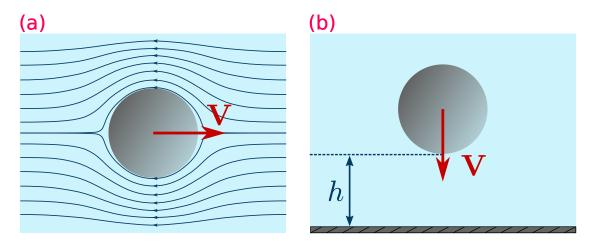
FIG. 1.2. A spherical particle submitted to Stokes drag. (a): A particle of radius R is moving at a velocity V in a viscous fluid. The stream lines are drawn. (b): A particle of radius R is moving at a velocity V towards a rigid boundary. The distance to the wall is denoted h.
