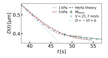
FIG. 5.18. Comparison of numerical simulations with two different Young's Moduli to experimental data. Distance between the two glass surfaces D as a function of time t. The experimental data is compared to numerical simulations based on the non-linear EHD model, for two different values of the Young's modulus indicated in the legend.
