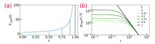
FIG. 5.9. Theoretical force and pressure field in the rigid case. (a): Dimensionless theoretical force  $F_{rigid}$  as a function of dimensionless time t, computed from Eq. (5.48). The green dashed lines indicate the times t at which the pressure is plotted in (b). (b): Dimensionless theoretical pressure field  $p_{rigid}(r,t)$ , computed from Eq. (5.47), for different dimensionless times t, signaled in (a) by green dashed lines.
