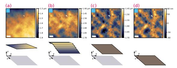
FIG. A.1. **Treatment of raw AFM images.** Image et different steps of treatment and schematic of the defect to correct. (a): Raw image obtained after a topography measurement. (b): After correction of the planar tilt. (c): After correction of the gap between successive lines. (d): After subtracting the mean plane.
