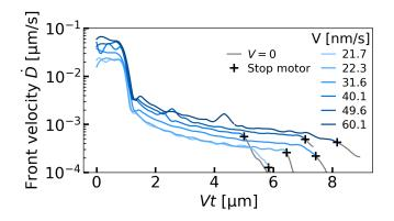
FIG. A.8. Front velocity of the spherical probe in SFA. From the data of Fig. 5.6(b), the time-derivative of the distance D between the two glass interfaces is computed and plotted as a function of Vt, the traveling distance imposed at the back of the spring.
