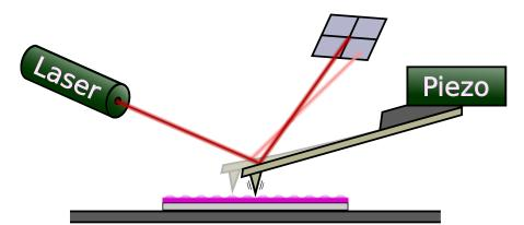
FIG. 2.3. Schematic of an AFM.A sharp tip is held by a cantilever, which is supported by a chip. A piezo element moves vertically the chip, whose position is noted  $z_{piezo}$ . A laser beam is sent on the top face, at the edge of the cantilever. The reflection of the laser is monitored by a photodiode. From the shifted signal of the photodiode, the deflection of the cantilever  $Z_{canti}$  is extracted.
