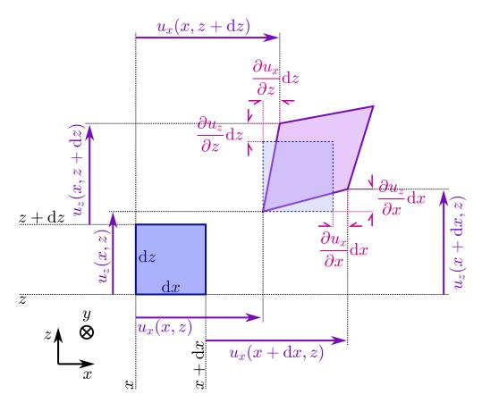
FIG. 1.6. Two-dimensional displacement of an infinitesimal surface element upon deformation. Originally located at a position (x, z), an infinitesimal surface element dxdz is displaced by u upon a deformation. The strain tensor  $\epsilon$  is computed using the partial derivatives of the displacement field u, using Eq. (1.38).
