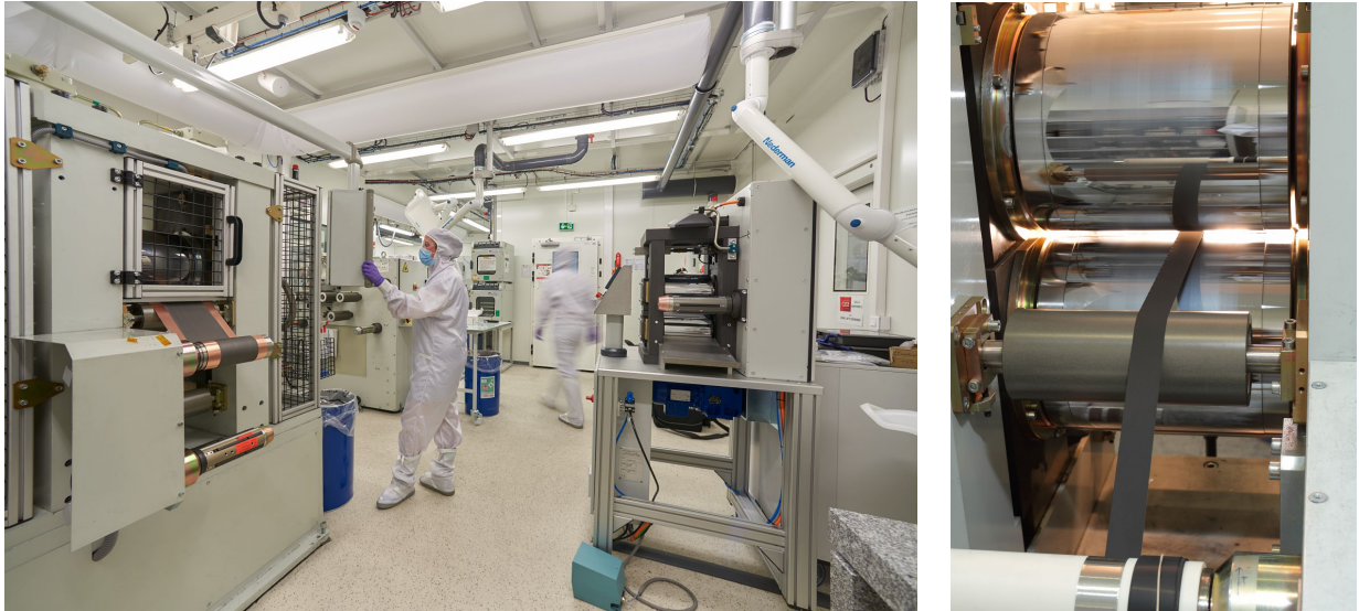
Figure 2: Calendering machines used for the manufacturing of Li-ion battery electrodes (CEA LITEN).
