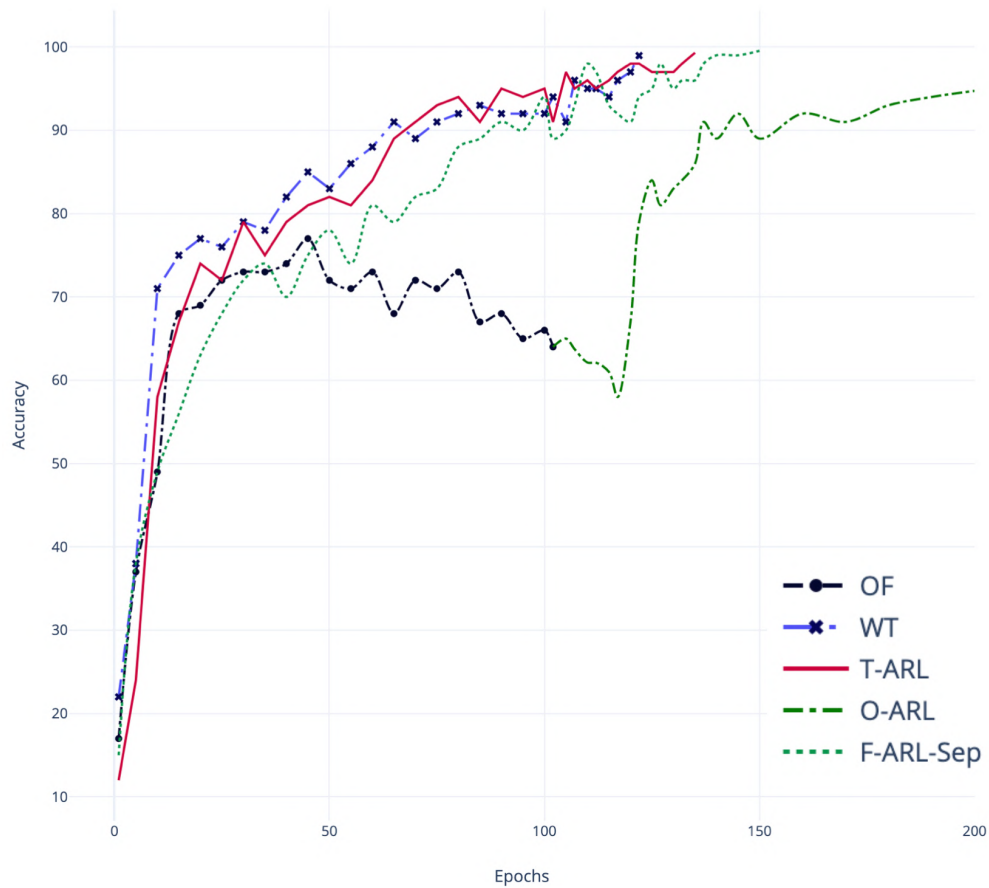
Figure 7.6: Comparison of different models on the task of digit classification on MNIST for the over-fitting scenario. The accuracy results are reported as the average of 5 experiments with the best hyper-parameters. OF is the over-fitted model, which is used by O-ARL as the initial start for solving the over-fitting problem. WT is the well trained model, T-ARL is the model which is trained from the start with ARL, and F-ARL-Sep is the WT model and fine-tuned with both ARL and sep loss 7.4 .
