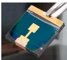
*Figure 3.13: Typical triple cation lead halide perovskite solar cell with glass/FTO/c-TiO<sub>2</sub>/m-TiO<sub>2</sub>/HaP/Spiro-MeOTAD/gold*
