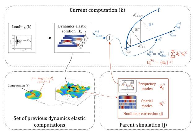
Figure 4.3 • Computation (k) enhanced from a chosen parent-simulation
