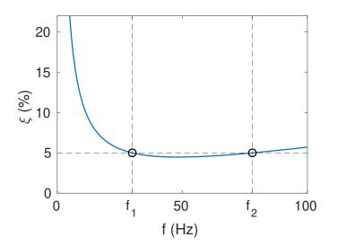
**Figure 3.4** • Evolution of the damping rate as a function of the frequency. A Rayleigh damping matrix is used with a damping rate fixed at 5 % for the first two eigenfrequencies  $f_1 = 30$  Hz and  $f_2 = 78$  Hz.
