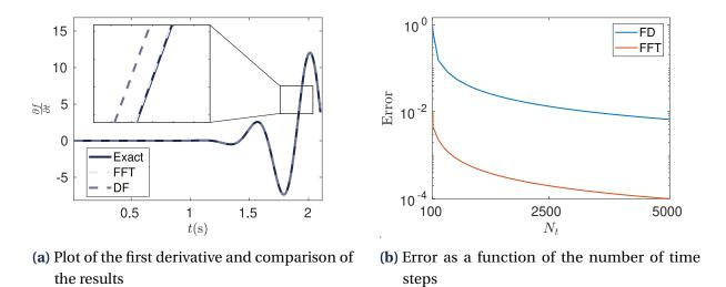
Figure A.2 • Comparison of Fourier and finite difference first order derivation
