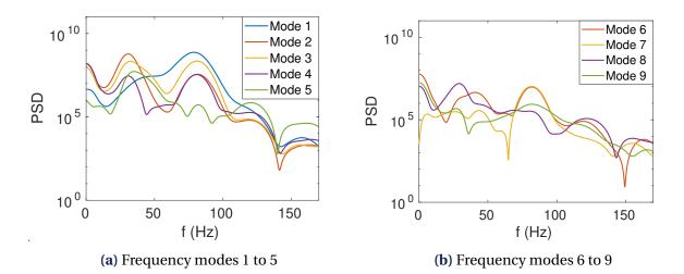
**Figure 3.18** • Power Spectral Density of the nine estimated PGD modes for the beam solicited with load 2 - bi-frequency load with  $f_a = 40$  Hz,  $f_b = 80$  Hz at  $U_d^{\text{max}} = 30$  mm
