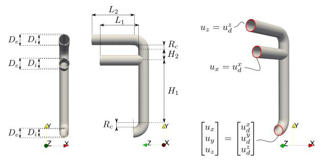
Figure 3.23 • Three-dimensional structure with boundary conditions
