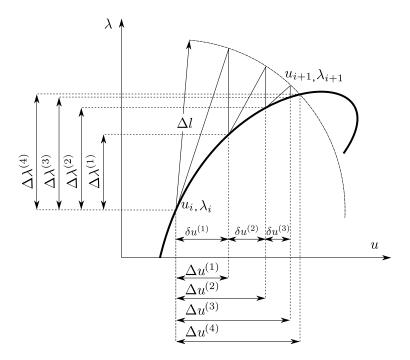
Figure 1.7 • Spherical Riks method, reproduced from [Crisfield, 1983].
