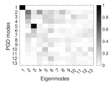
**Figure 3.22** • Modal Assurance Criterion (MAC) matrix comparing the basis of PGD modes with classical LNMs for the beam solicited with load 3 - a complex load
