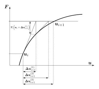
Figure 1.6 • Newton-Raphson scheme applied to mechanics
