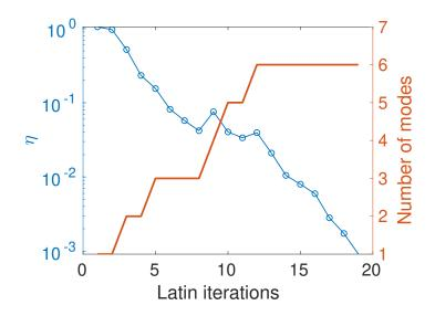
**Figure 3.9** • Convergence of the error indicator and evolution of the number of PGD modes with LATIN iteration for the beam solicited with load 1 - f = 40 Hz and  $U_d^{max} = 100$  mm
