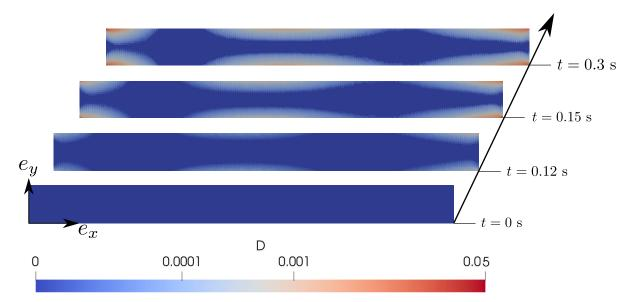
**Figure 3.7** • Evolution of the damage field for the beam solicited with load 1 - f = 40 Hz and  $U_d^{\text{max}} = 100$  mm
