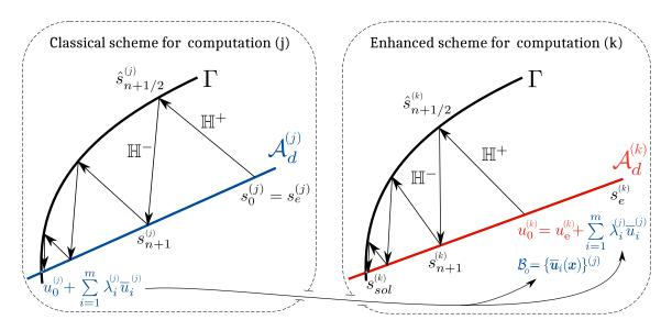
Figure 4.2 • Standard and enhanced non-linear LATIN-PGD schemes
