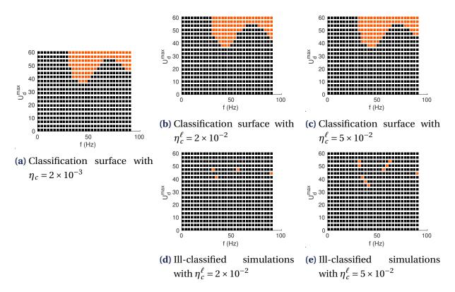
**Figure 5.3** • Influence of the stopping criterion on the classification precision between computations leading to failure (red) and safe results (black).
