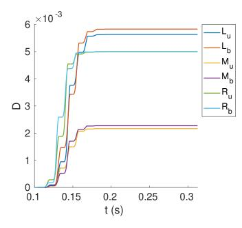
**Figure 3.8** • Damage evolution at different points of the beam (Figure 3.5) solicited with load 1 - f = 40 Hz at  $U_d^{max} = 100$  mm
