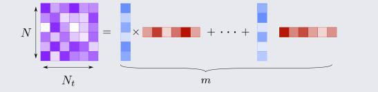
Under a discretised form, the *m*-th order reduced approximation  $\{U_m\}$  of the displacement  $\{U\}$  reads
