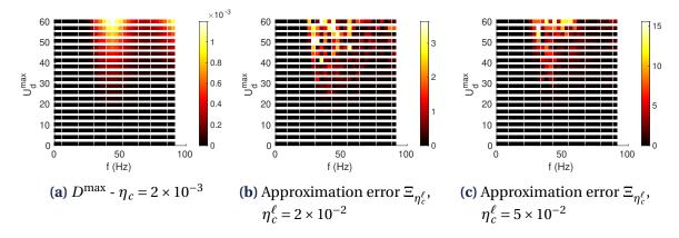
**Figure 5.2** • Approximation error for different values of coarse stopping criterion  $\eta_c^\ell$
