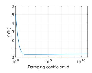
**Figure 3.16** • Evolution of the overlapping error  $\zeta$  for dampened frequency computation with regard to the damping coefficient *d* for the beam solicited with load 1 mono-frequency Gaussian load with f = 40 Hz and  $U_d^{\text{max}} = 100$  mm
