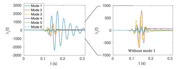
**Figure 3.13** • Six estimated temporal PGD modes for the beam solicited with load 1 - f = 40 Hz and  $U_d^{\text{max}} = 100$  mm
