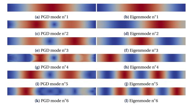
**Figure 3.10** • Magnitude of PGD modes for the beam solicited with load 1 - f = 40 Hz and  $U_d^{\text{max}} = 100$  mm compared to energetically predominant eigenmodes
