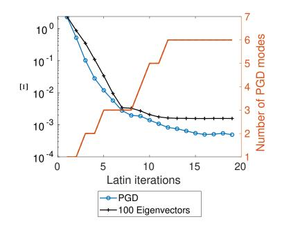
**Figure 3.12** • Evolution of the error with LATIN iteration using an adaptive PGD basis or a fixed basis comprising the first 100 eigenmodes for the beam solicited with load 1 - f = 40 Hz and  $U_d^{\text{max}} = 100$  mm
