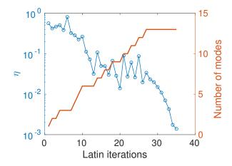
**Figure 3.25** • Evolution of the error indicator and the number of PGD modes for the threedimensional pipe structure solicited with a complex load
