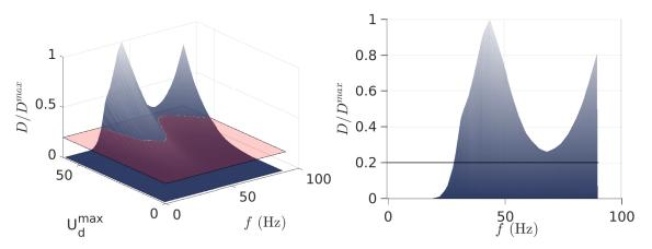
(a) Side view of the response surface showing the (b) Front view of the response surface shownormalised maximum damage in the structure.(b) Front view of the response surface shownormalised maximum damage in the structure.
