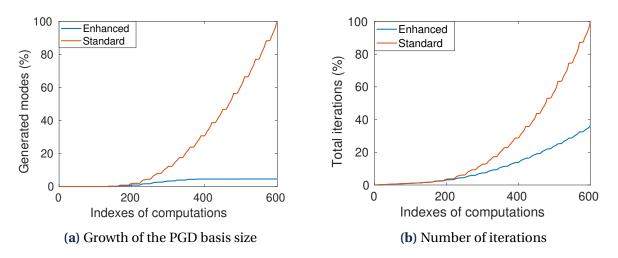
Figure 4.8 • Comparison of the standard method with the enhanced strategy.
