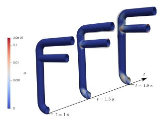
Figure 3.26 • Evolution of the damage field for the pipe solicited with a complex loading
