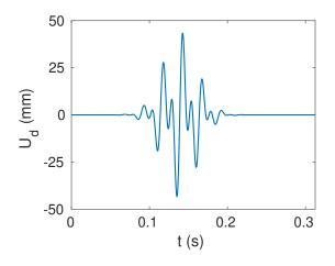
Figure 3.17 • Temporal load 2 - bi-frequency Gaussian case
