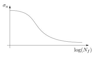
Figure 1.4 • Example of an S-N curve
