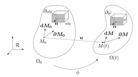
Figure 1.2 • Kinematic transformation of a continuum medium
