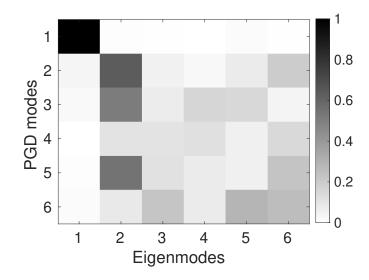
**Figure 3.11** • Modal Assurance Criterion Matrix of the PGD modes and the eigenmodes for the beam solicited with load 1 - f = 40 Hz and  $U_d^{\text{max}} = 100$  mm
