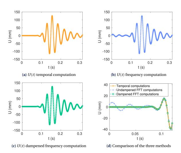
**Figure 3.15** • Numerical effect of the artificial damping: comparison of the temporal, nondampened (showing unwanted artefacts) and dampened frequency computations for the elastic initialisation at point  $P_I$  of the beam solicited with load 1 mono-frequency Gaussian load with f = 40 Hz and  $U_d^{\text{max}} = 100$  mm
