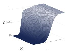
Figure C.1 • Example of a fragility surface
