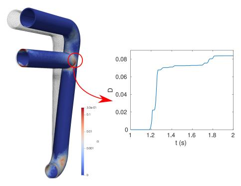
**Figure 3.27** • Damage field in the three-dimensional pipe structure solicited with a complex load at time t = 2 s and damage evolution at the T-junction between the tube and the middle branch over time
