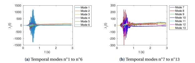
Figure 3.20 • Temporal PGD modes for the beam solicited with load 3 - a complex load
