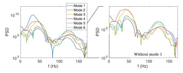
**Figure 3.14** • Power spectral densities (PSD) of the six estimated frequential PGD modes for the beam solicited with load 1 - f = 40 Hz and  $U_d^{\text{max}} = 100$  mm
