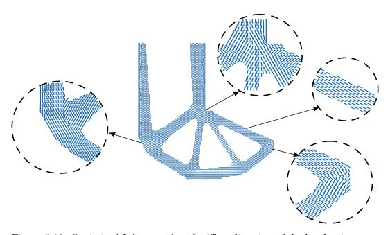
Figure 5.13: Optimized L-beam: plot of stiffest direction of the local anisotropy
