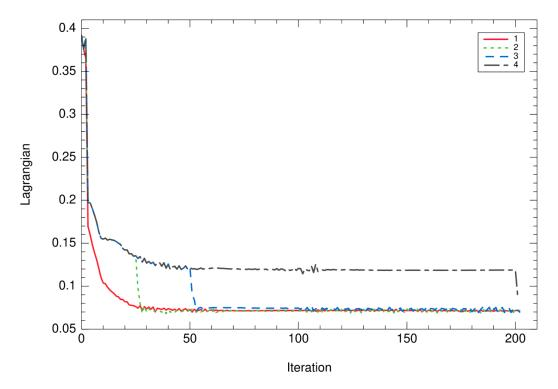
Figure 5.9: Lagrangian evolution for each strategy of the coupled shape and orientation optimization using an optimality criterion for the  $2\mathrm{D}$  cantilever example
