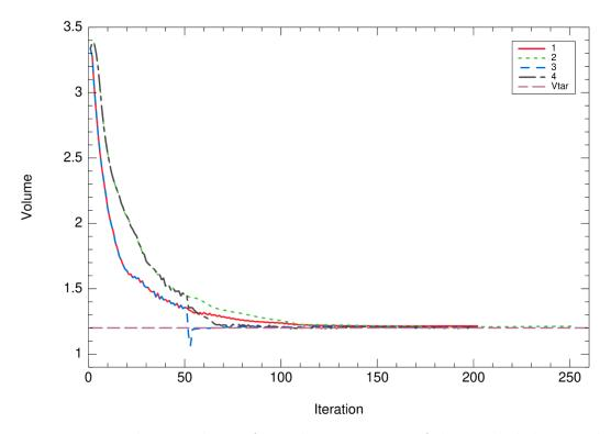
Figure 5.33: Volume evolution for each optimization of the coupled shape and orientation optimization using the gradient descent method for the 2D bridge example  $\frac{1}{2}$
