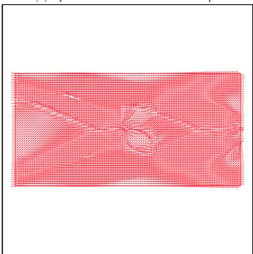
Figure 5.7: Optimized cantilever using strategy 4: optimization of shape then optimization of orientation using the optimality criterion
