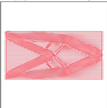
Figure 5.16: Optimized cantilever using strategy 3: simultaneous optimization of shape and orientation using the gradient descent method for  $n \geq 50$
