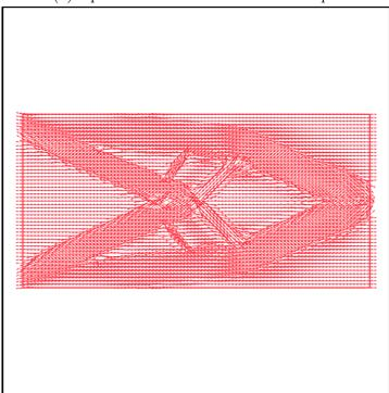
Figure 5.18: Optimized cantilever using strategy 5: optimization of orientation using the gradient descent method after each 50 iterations of shape optimization
