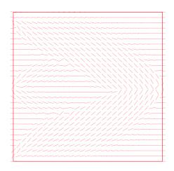
(b) Optimized orientation of a displacement inverter
