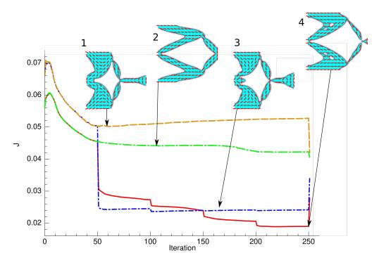
Figure 5.25: Obtained structures and objective functions for the two optimization strategies and the two initializations of the inverter example. Optimization 1: orientation optimized only in the end with  $\alpha_0 = \pi/2$ . Optimization 2: orientation optimized only in the end with  $\alpha_0 = 0$ . Optimization 3: concurrent optimization with  $\alpha_0 = \pi/2$ . Optimization 4: concurrent optimization with  $\alpha_0 = 0$
