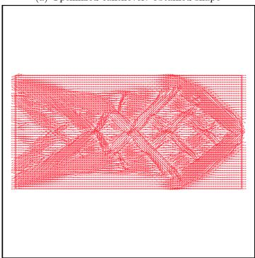
Figure 5.14: Optimized cantilever using strategy 1: simultaneous optimization of shape and orientation using the gradient descent method
