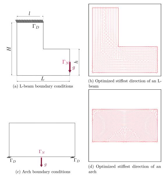
Figure 3.5: L-beam and arch optimal orientations with  $\alpha_0 = 0$
