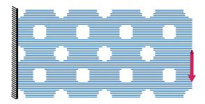
Figure 5.1: Initialization of the cantilever: plot of stiffest direction of the local anisotropy
