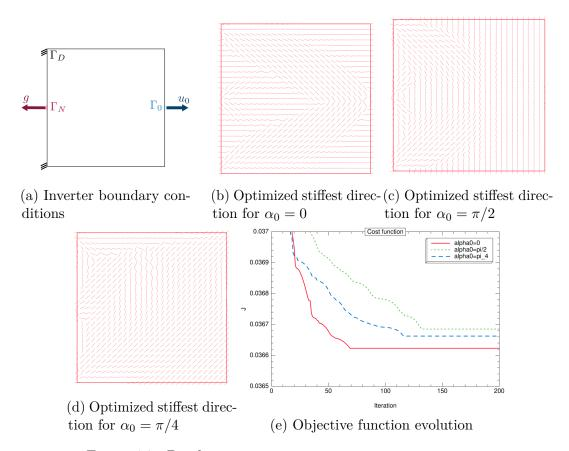
Figure 3.7: Displacement inverter orientation optimization
