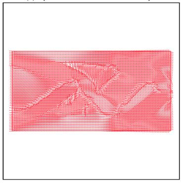
Figure 5.4: Optimized cantilever using strategy 1: simultaneous optimization of shape and orientation using the optimality criterion
