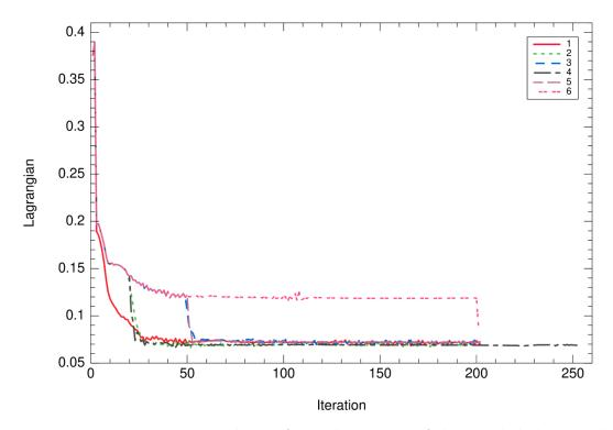
Figure 5.21: Lagrangian evolution for each strategy of the coupled shape and orientation optimization using the gradient descent method for the 2D cantilever example  $\alpha$
