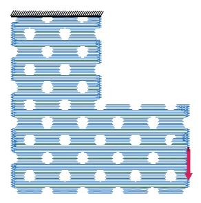
Figure 5.12: Initialization of the L-beam: plot of stiffest direction of the local anisotropy  $\frac{1}{2}$
