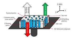
Figure 2.4: Columnar grains formation in SLM (figure from [87])
