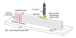
Figure 2.2: Direct energy deposition AM (figure from [66])
