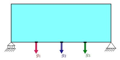
Figure 5.26: 2D bridge loads and boundary conditions
