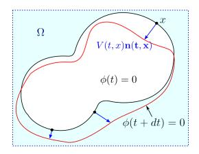
Figure 1.2: Level set function convection
