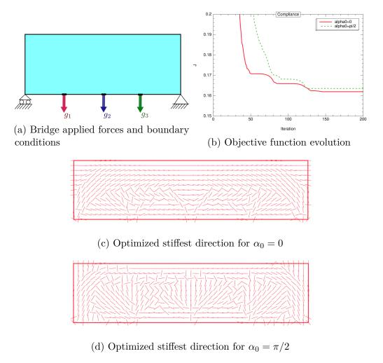
Figure 3.8: Multi-load bridge orientation optimization
