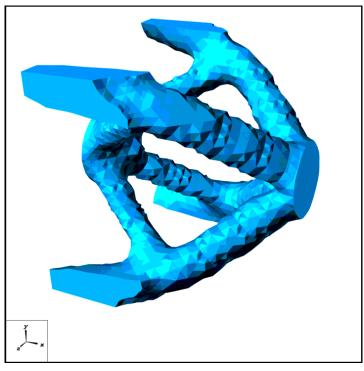
(a) Optimized displacement inverter: obtained shape
