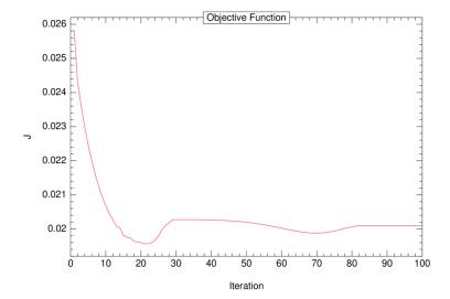
Figure 3.27: Evolution of the compliance in the orientation optimization under a constraint of orientation angle difference to a fixed angle (Example 1)
