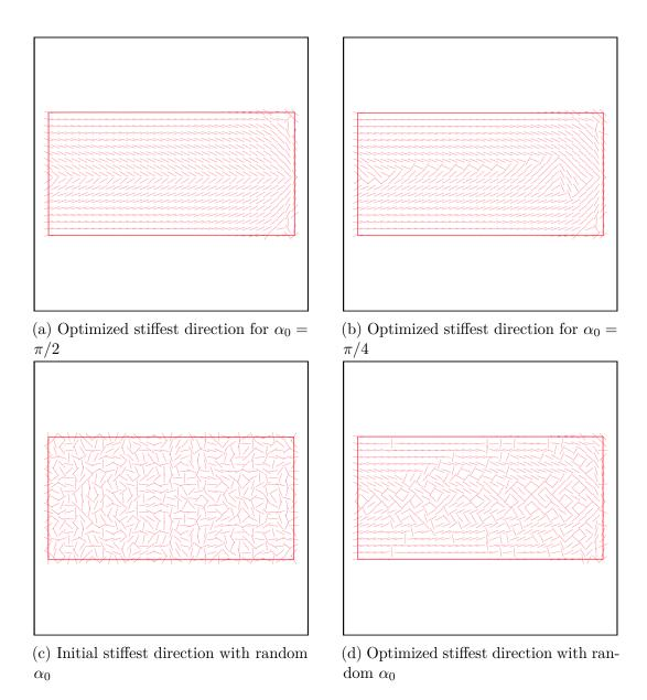
Figure 3.4: Optimization of a cantilever orientation using different initializations of the orientation
