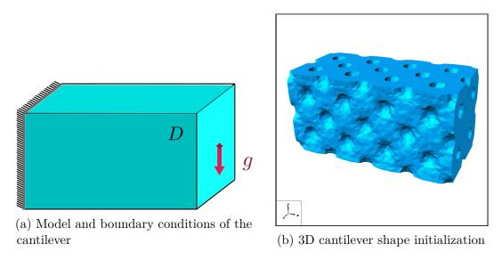
Figure 5.36: 3D cantilever problem model
