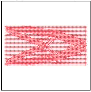
Figure 5.19: Optimized cantilever using strategy 6: optimization of shape then optimization of orientation using the gradient descent method
