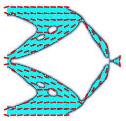
(b) Optimized topology and orientation of a 2D displacement inverter: plot of the stiffest direction of the local anisotropy
