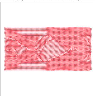
Figure 5.5: Optimized cantilever using strategy 2: simultaneous optimization of shape and orientation using the optimality criterion for  $n \ge 25$
