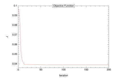
Figure 3.37: Evolution of the compliance in the orientation optimization under a constraint of orientation angle difference to a fixed angle (Example 3)
