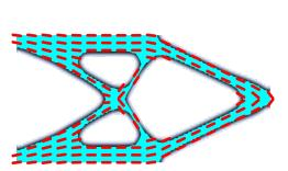
(a) Optimized topology and orientation of a 2D cantilever: plot of the stiffest direction of the local anisotropy
