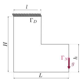
Figure 5.11: 2D L-beam load and boundary condition
