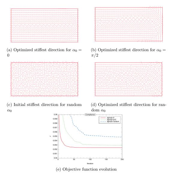
Figure 3.6: Cantilever orientation optimization with a gradient descent
