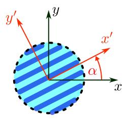
Figure 2.7: Orientation angle  $\alpha$  of the orthotropic material axes of a 2D structure
