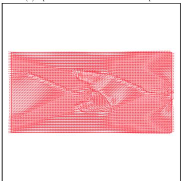
Figure 5.6: Optimized cantilever using strategy 3: optimization of orientation each 50 iterations of shape optimization using the optimality criterion
