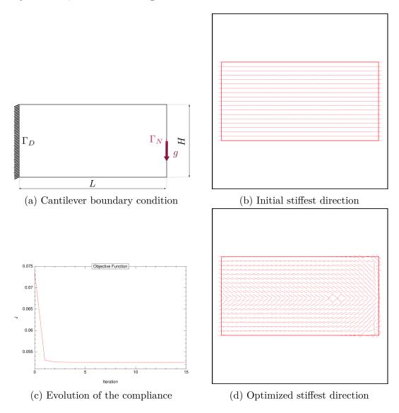
Figure 3.3: Optimization of a cantilever
