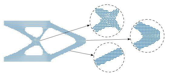
Figure 5.2: Optimized cantilever: plot of stiffest direction of the local anisotropy
