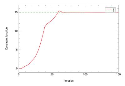
Figure 4.11: Evolution of the constraint function  $C(\alpha)$  in the 3D orientation optimization under a constraint on the angle partial gradient along y
