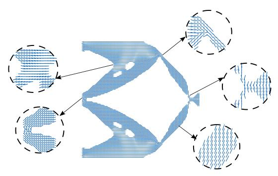
Figure 5.24: Optimized displacement inverter: plot of stiffest direction of the local anisotropy
