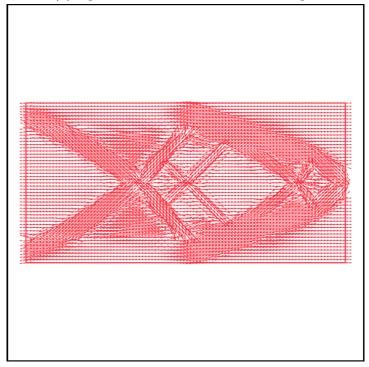
Figure 5.15: Optimized cantilever using strategy 2: simultaneous optimization of shape and orientation using the gradient descent method for  $n \ge 20$
