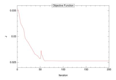
Figure 3.32: Evolution of the compliance in the orientation optimization under a constraint of orientation angle difference to a fixed angle (Example 2)
