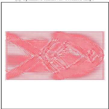
Figure 5.17: Optimized cantilever using strategy 4: optimization of orientation the gradient descent method after each 20 iterations of shape optimization
