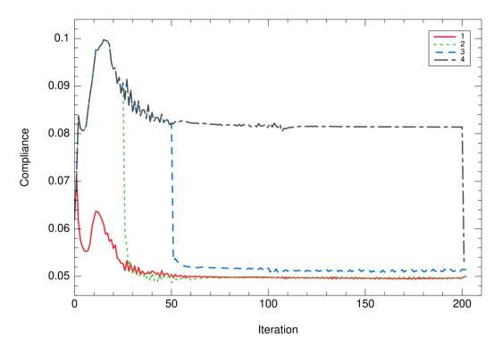
Figure 5.8: Compliance evolution for each strategy of the coupled shape and orientation optimization using an optimality criterion for the  $2\mathrm{D}$  cantilever example
