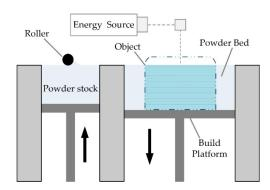
Figure 2.1: Powder bed fusion AM (figure from [24])
