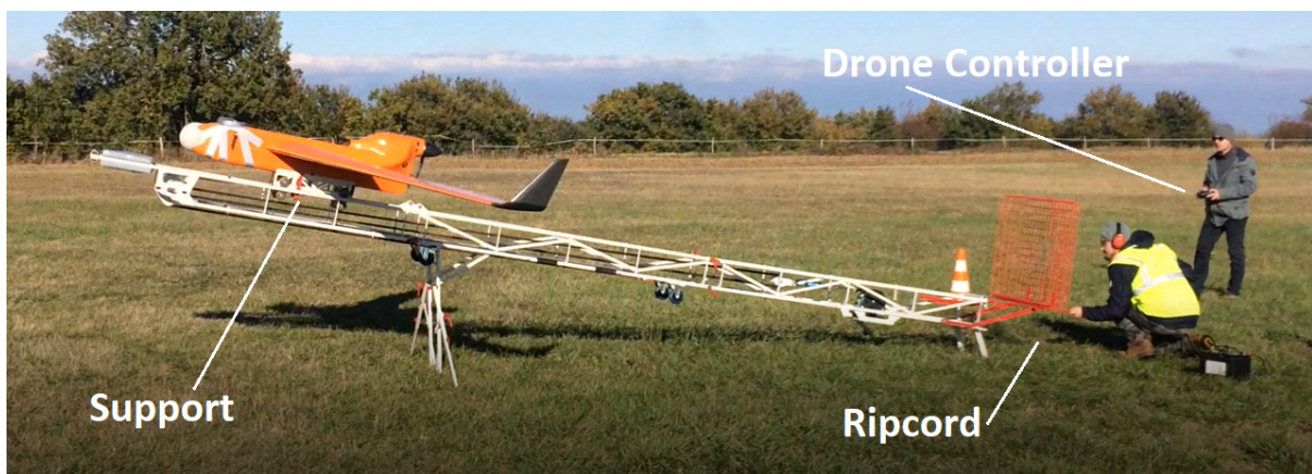
Fig. 2.9 The Boreal Lab drone approaching the end of the slingshot launch platform, moments before taking flight
