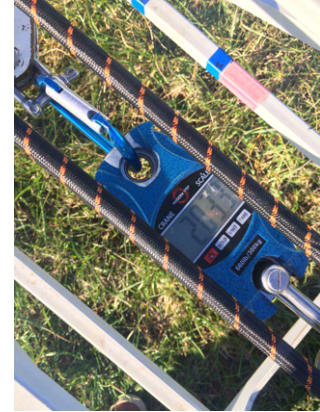
Fig. 2.11 Portable crane scale shows the force on the cord before launch (203.3 kg or 1993.7 N)
