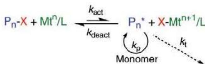
Figure III.6: Global process of ATRP (reproduced from ref.31).
