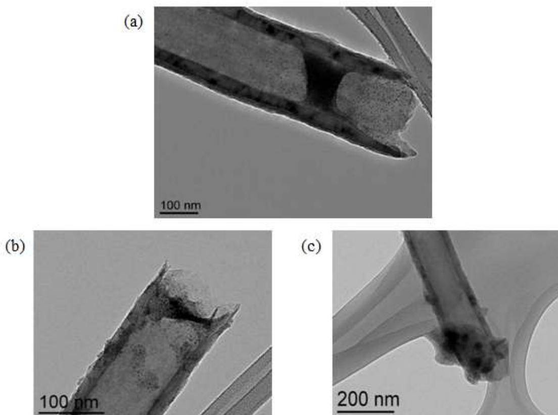
**Figure III.14: TEM images of (a) confinement of the surface-modified Fe NPs in the f-CNT<sub>1</sub> and (b-c) polymerization of isoprene with the f-CNT<sub>1</sub>-confined surface-modified Fe NPs.**
