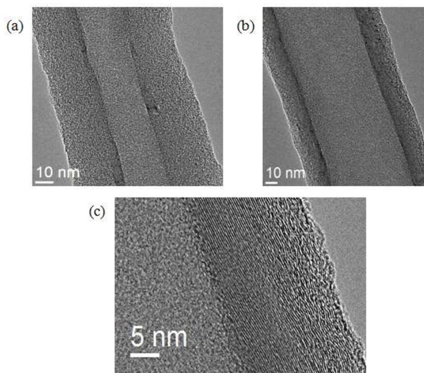
**Figure II.1:** HRTEM images of (a) a CNT<sub>1</sub> with  $d_{\text{inner}} \sim 20\text{-}25$  nm and  $d_{\text{outer}} \sim 75\text{-}80$  nm, and (b) a CNT<sub>1</sub> with  $d_{\text{inner}} \sim 60$  nm and  $d_{\text{outer}} \sim 95\text{-}100$  nm. (c) is magnification of part of the CNT<sub>1</sub> in (b) indicating its graphite layers.
