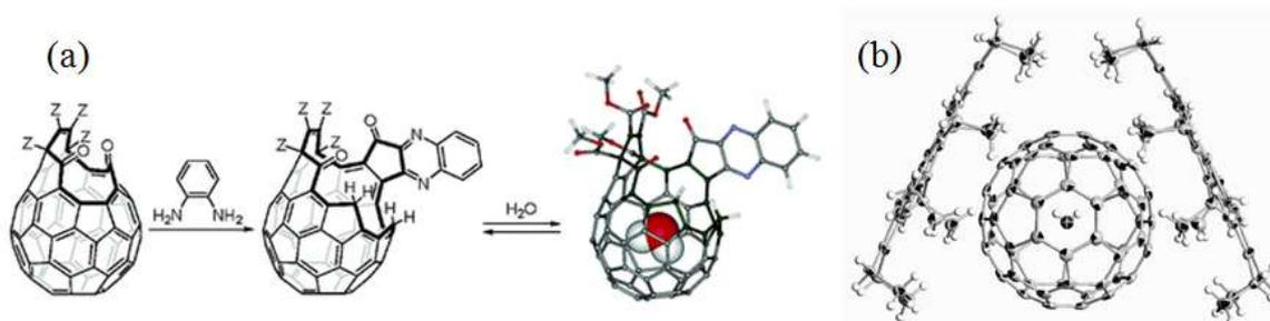
**Figure I.2:** (a) process of confinement of a single water molecule within the open-caged fullerene (Z=CO<sub>2</sub>Me) (20); (b) X-ray structure of the molecular H<sub>2</sub>O@C<sub>60</sub>·(NiOEP)<sub>2</sub> (NiOEP= nickel (II) octaethylporphyrin) at the 50% probability level (reproduced from ref.21).
