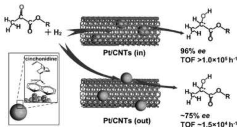
**Figure I.13: Asymmetric hydrogenation of  $\alpha$ -ketoesters on Pt NPs encapsulated within CNTs (Pt/CNTs (in)) and adsorbed onto CNTs (Pt/CNTs (out)) with CD as a chiral modifier (reproduced from ref.57) (TOF= turnover frequency).**
