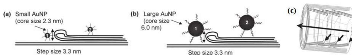
**Figure II.32: Schematic representation of Au NPs of different sizes, (a) smaller and (b) larger, residing at internal step-edges of a GNF; (c) schematic representation of GNF step-edges (reproduced from ref.30).**
