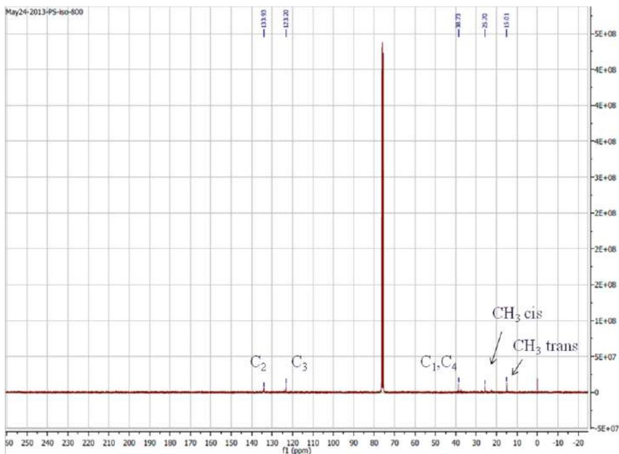
Figure V.2: NMR  $^{13}\text{C}$  of polyisoprene in  $\text{CDCl}_3$ .
