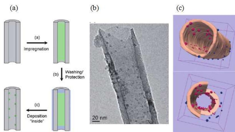
**Figure I.26: (a) Schematic view of a longitudinal cross section of a CNT during the different steps for the selective deposition of NPs inside CNTs; (b) Typical 2D-TEM image of the sample “metal inside”; (c) Modeling of the reconstructed volume: (pink) CNT, (red) Ni NPs inside the tube, (blue) Ni NPs on the external surface (reproduced from ref.173).**
