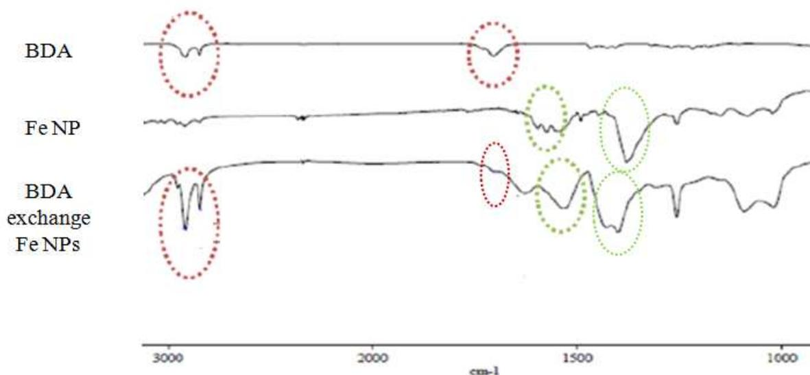
**Figure III.11: IR spectra comparison among BDA, the pre-formed Fe NPs and the BDA modified Fe NPs. C-H stretching vibration (left red cycle); C=O stretching vibration (middle red cycle); modifications for the different carboxylates on the Fe NPs (green cycles).**
