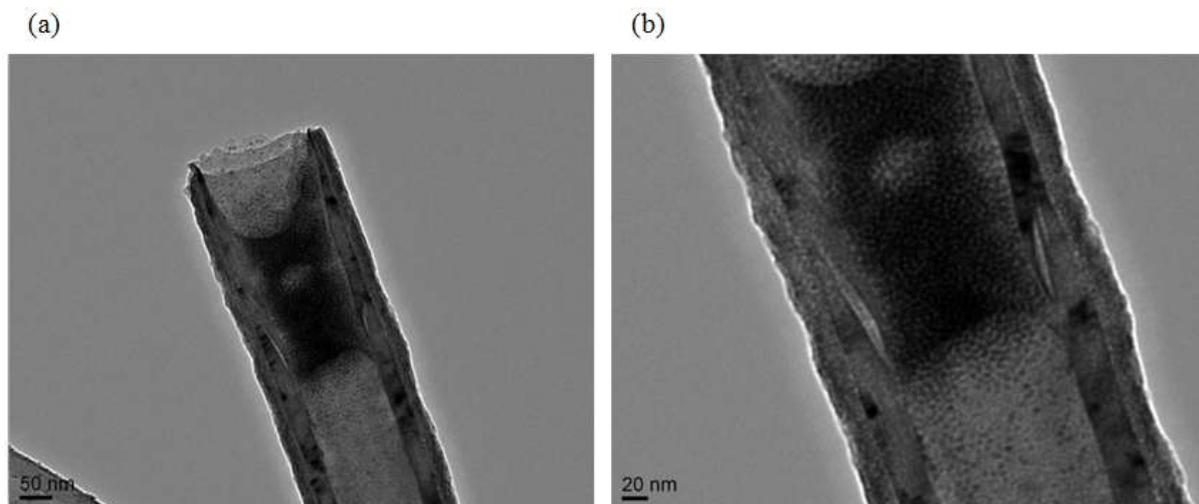
**Figure II.28: Encapsulated Fe NPs within f-CNT<sub>1</sub>.**
