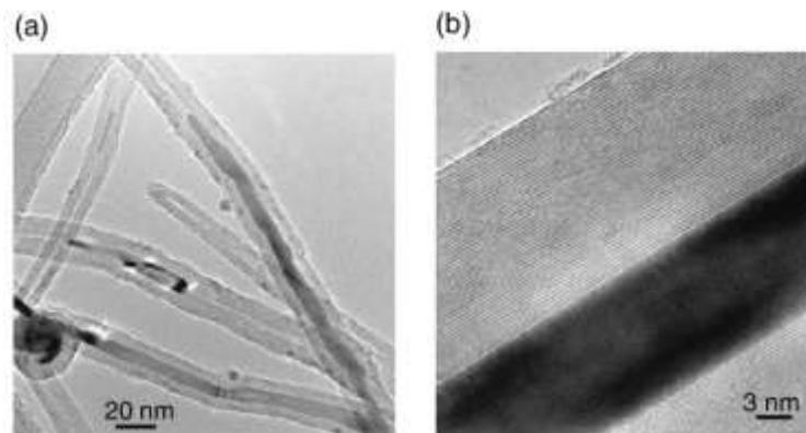
**Figure I.22: (a) TEM image of in situ filled MWCNTs obtained via a CCVD-related process. The filling material is pure  $\alpha$ -Fe (bcc Fe crystals). (b) High resolution of one of the Fe@MWCNTs in (a) (reproduced from ref.143).**
