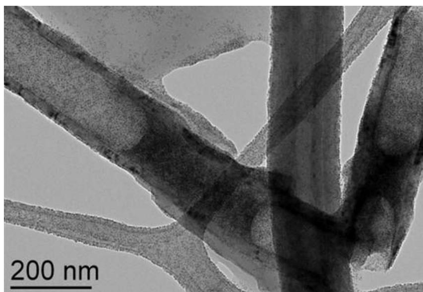
**Figure II.21: TEM image that display the position of the pre-formed Fe NPs and the liquid-gas interfaces near the tip of f-CNT<sub>1</sub>.**
