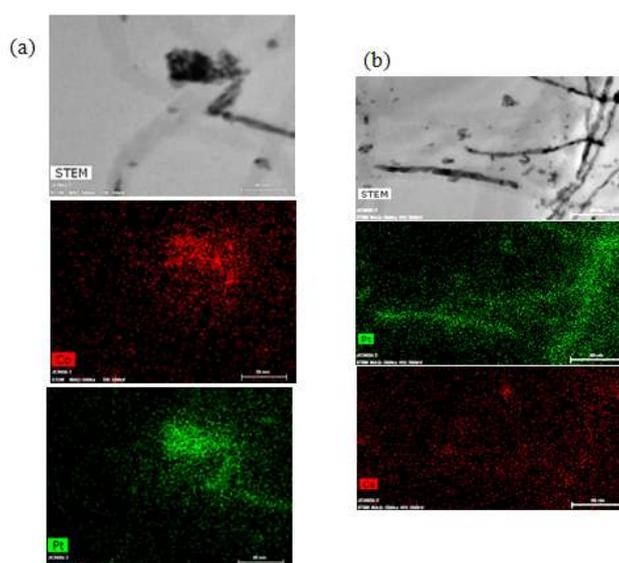
**Figure IV.13: STEM-EDX analysis of HCl washing sample.**
