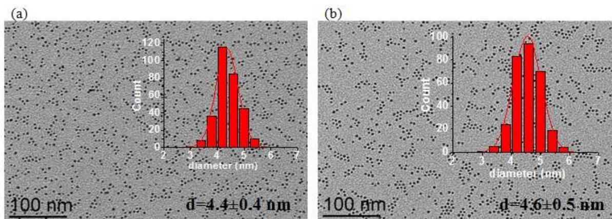
**Figure III.12: TEM images and size distributions of (a) the pre-formed Fe NPs and (b) the initiator-modified Fe NPs.**
