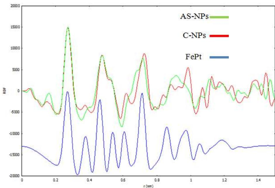
**Figure IV.34: RDF among the AS-NPs (green), C-NPs (red) and FePt bulk (blue).**
