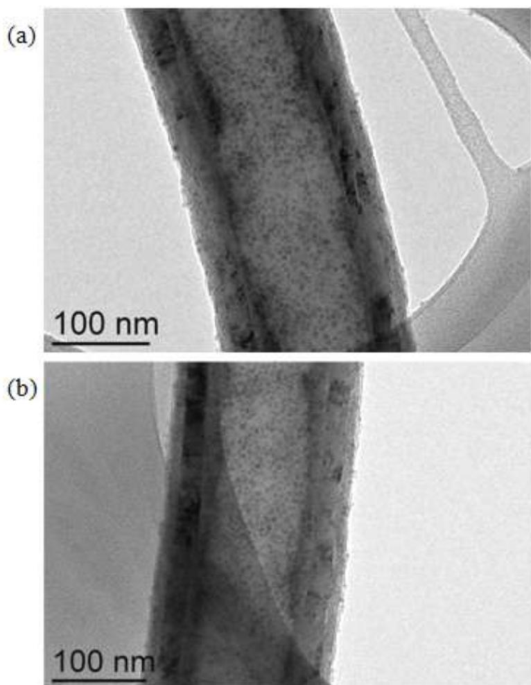
**Figure II.37: TEM images from the grid prepared directly with the solid FeNP@CNT<sub>1</sub>.**
