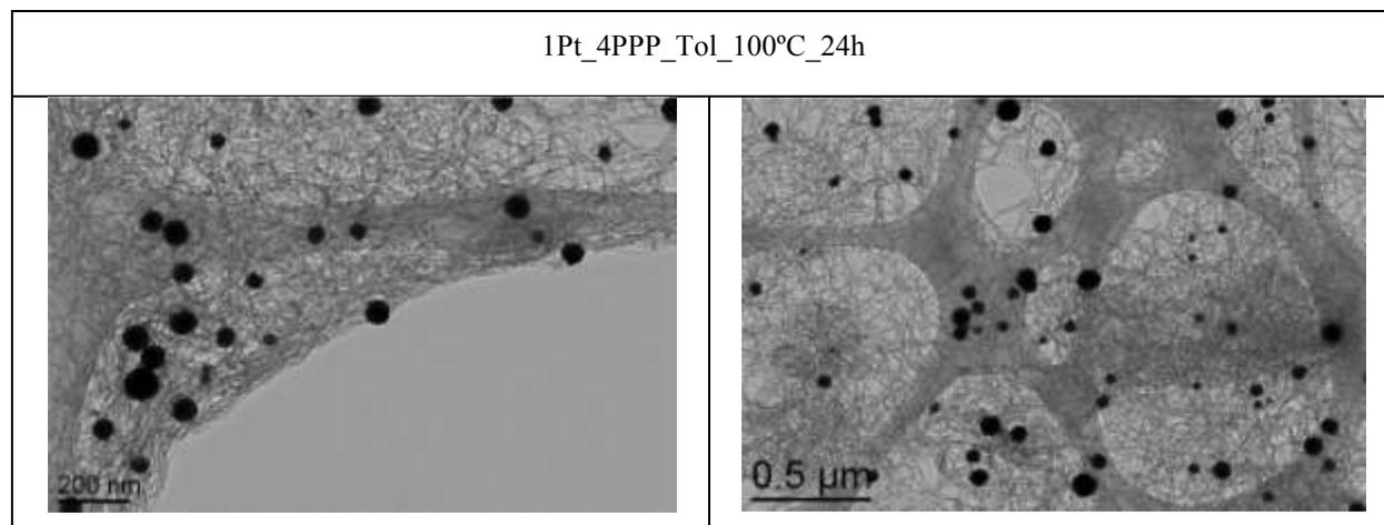
Therefore the addition of 4 equivalents of PPP gives rise to polydispersed NPs (55-100 nm) outside the CNTs while the CNTs remained empty. The NPs are smaller than in the absence of ligands but this experiment apart from the failure of complexes containing only PPP to enter and/or to be reduced into the CNTs, also indicates that PPP alone cannot stabilize small Pt NPs.
