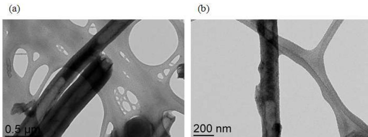
**Figure II.22: TEM micrograph of the interface found in the middle of f-CNT<sub>1</sub>.**
