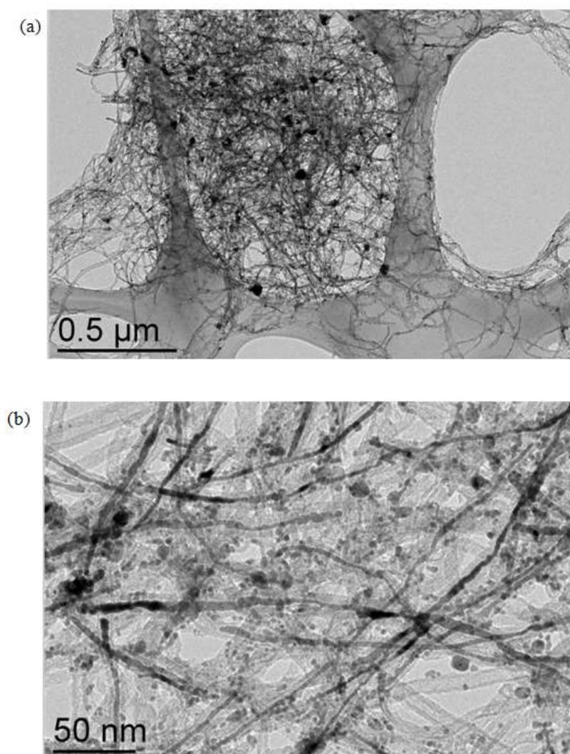
**Figure IV.8: (a-b) TEM images of the CNT-templated Co-Pt NWs and the polydispersed NPs attached on the outer surface of the f-CNT<sub>2</sub>.**
