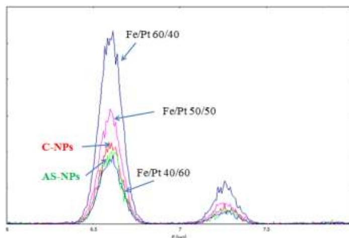
**Figure IV.31: XRF Fe K $\alpha$  and Fe K $\beta$  patterns of the comparison of the C-NPs (red) and AS-NPs (green) with the standard Fe/Pt composition prepared with organometallic complexes. (Amplitudes are normalized on the Pt L pattern).**
