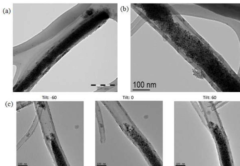
**Figure II.45: TEM images of (a-b) an almost completely filled f-CNT<sub>1</sub> in the condition "Fe\_1BBA:2PPP\_Mes\_150°C\_48h" with fast adding rate; (c) tomography images of a filled f-CNT<sub>1</sub>.**
