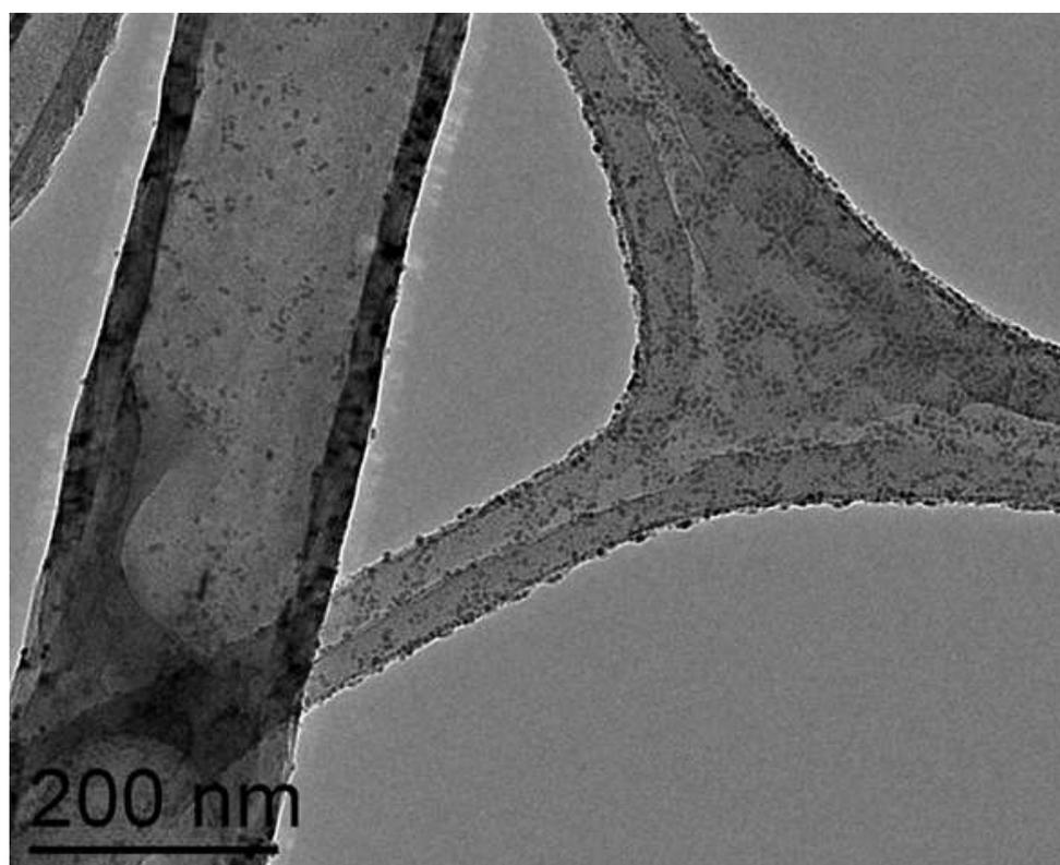
**Figure II.48: TEM image of the synthesis of Co NRs ("Co\_1.2LA\_1.2HDA\_Ani\_150°C\_24h") in the presence of the f-CNT<sub>1</sub>.**
