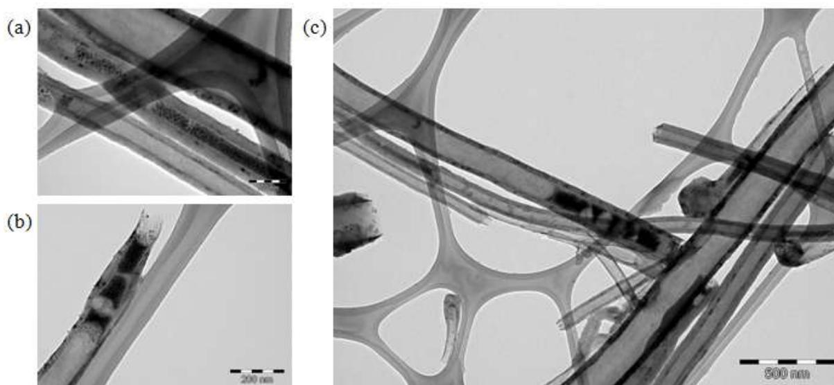
**Figure II.49: TEM images of Co NPs encapsulated within the f-CNT<sub>1</sub> in absence of the stabilizing ligands *via* the *in situ* solution method.**
