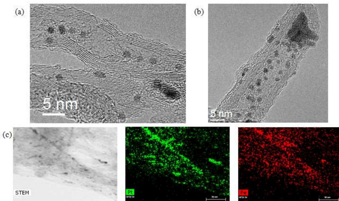
**Figure IV.27: (a-b) HRTEM images and (c) STEM-EDX analysis of the washed sample in "1[Pt(acac)<sub>2</sub>]<sub>1</sub>Fe\_2BBA\_2PPP\_Tol\_100°C\_24h".**
