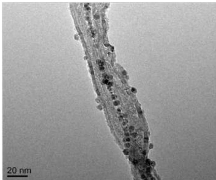
**Figure II.35: TEM image of the f-CNT<sub>2</sub> attached by the Fe NPs on its outer surface.**
