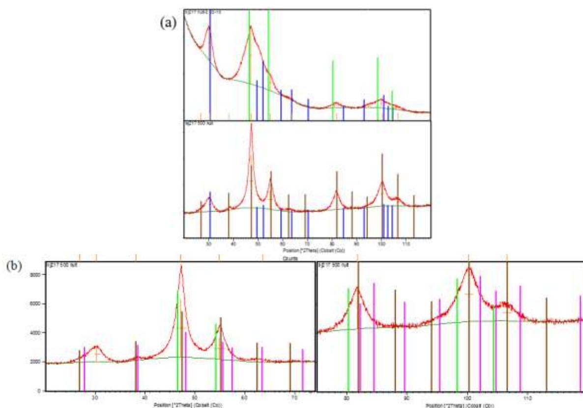
**Figure IV.56: (a) Comparison of XRD patterns between the samples before annealing (top) and after annealing (bottom); (b) magnifications of the bottom diffractogram in (a) (blue line: carbon, green line: Pt; brown line: FePt<sub>3</sub>; pink line: FePt).**
