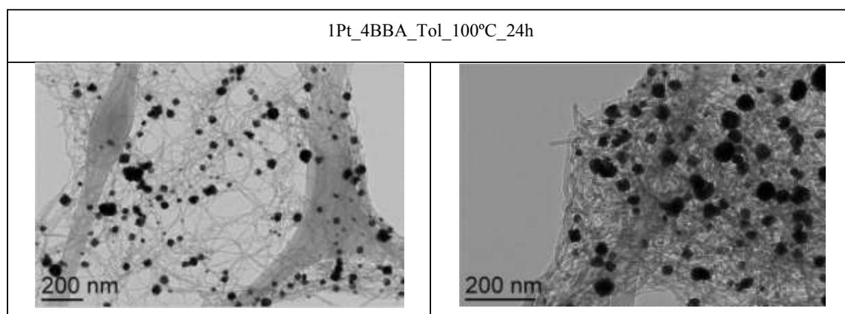
The NPs formed outside the CNTs are more polydispersed (15-100 nm), which indicates that neither BBA is able to stabilize small Pt NPs.
