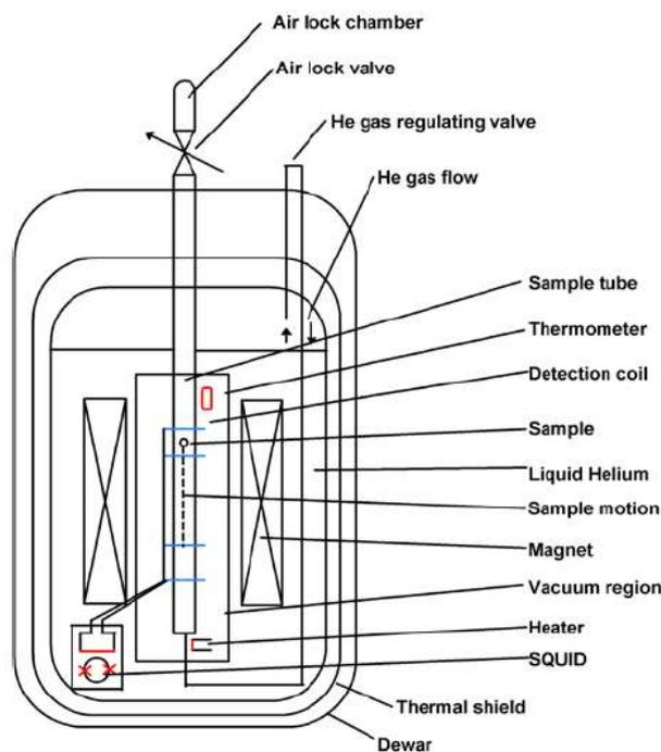
**Figure A.3: Schematic representation of a SQUID magnetometer.**
