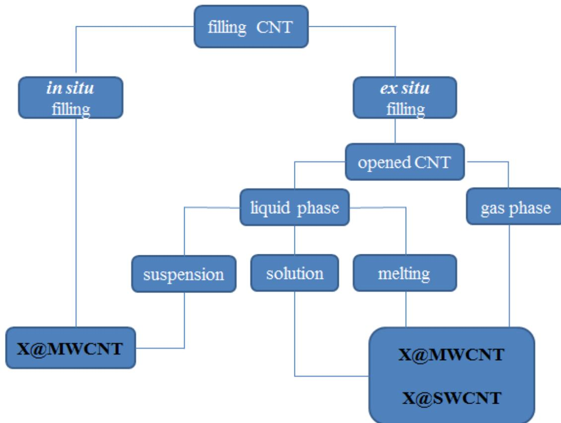
**Figure I.21: Schematic representation of main filling routes for CNT-based hybrid nanomaterials (X represents foreign materials).**
