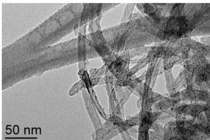
**Figure IV.7:** TEM image of the pre-formed Co-Pt NPs attached on the f-CNT<sub>2</sub>.
