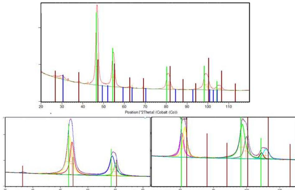
**Figure IV.54: XRD pattern of the polyisoprene-coated Fe-Pt NWs at 600°C for one hour. Blue, green and brown lines correspond respectively to carbon, Pt and ordered FePt<sub>3</sub> phases.**
