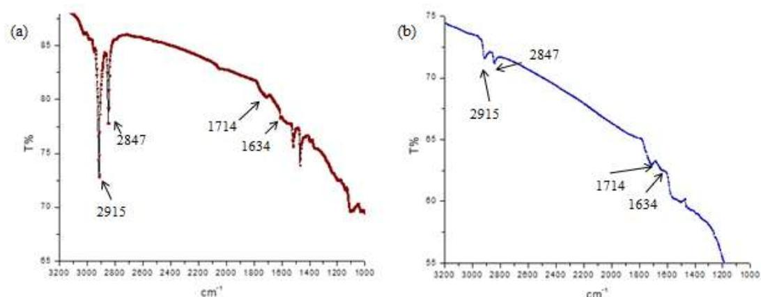
**Figure II.7: IR spectra of (a) the f-CNT<sub>1</sub> and (b) the f-CNT<sub>2</sub>.**
