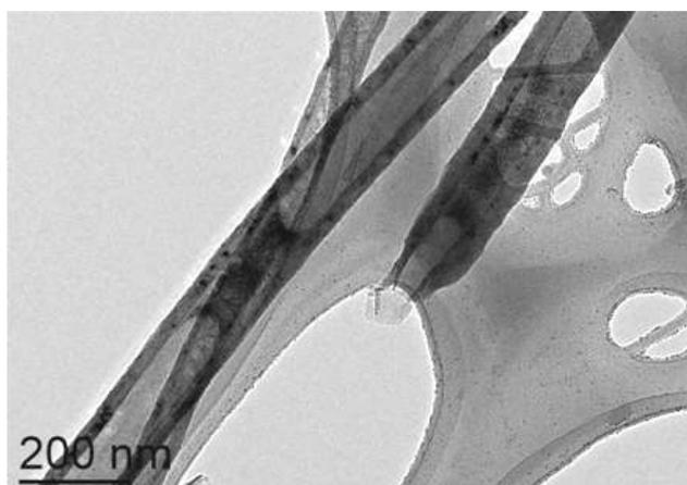
**Figure II.34: TEM image of filled f-CNT<sub>1</sub> with the pre-formed Co NPs ("Co\_1.2BBA\_1.2PPP\_Mes\_150°C\_24h").**
