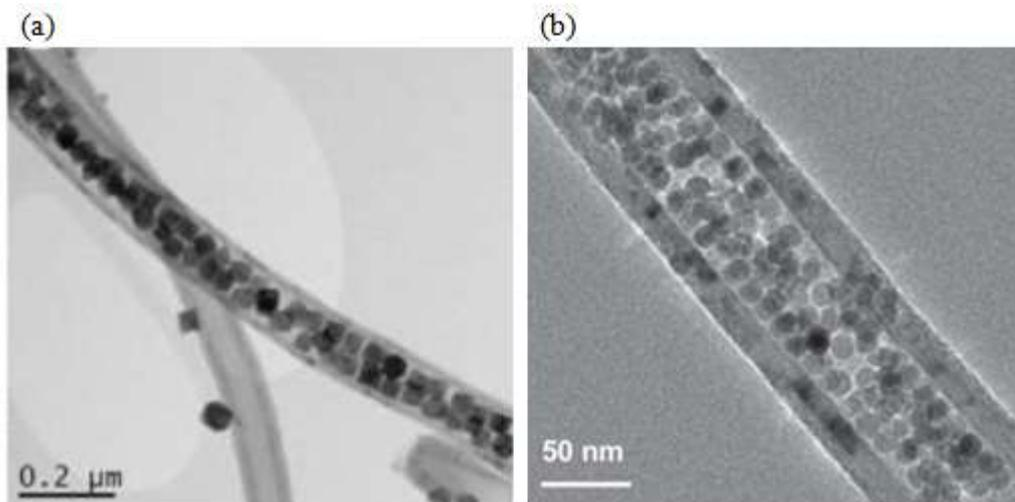
**Figure I.20: TEM images of the MWCNT-encapsulated Co-based NPs (141) and Fe<sub>3-x</sub>O<sub>4</sub> NPs (142) (reproduced from ref. 141 and 142).**
