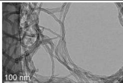
In the presence of 1 BBA and 1 PPP, nothing was observed in the interior of CNTs, however the cobalt particles formed outside are big and ill-shaped.
