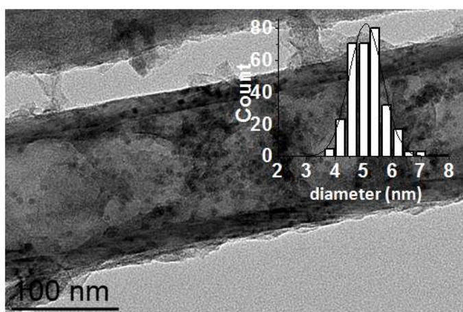
Figure III.20: TEM image of the FeNP@Fe@PI@CNT<sub>1</sub>.
