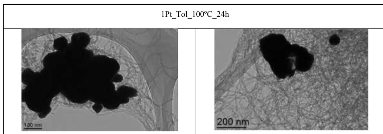
This means that the aromatic ligands are necessary for the introduction of the Pt in the CNTs.
