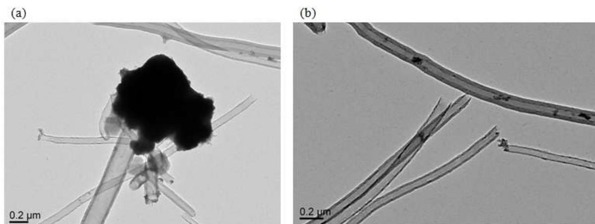
**Figure II.50: TEM images of (a) the massive agglomeration outside the tube and (b) the coalescences of the Co NPs inside the tubes.**
