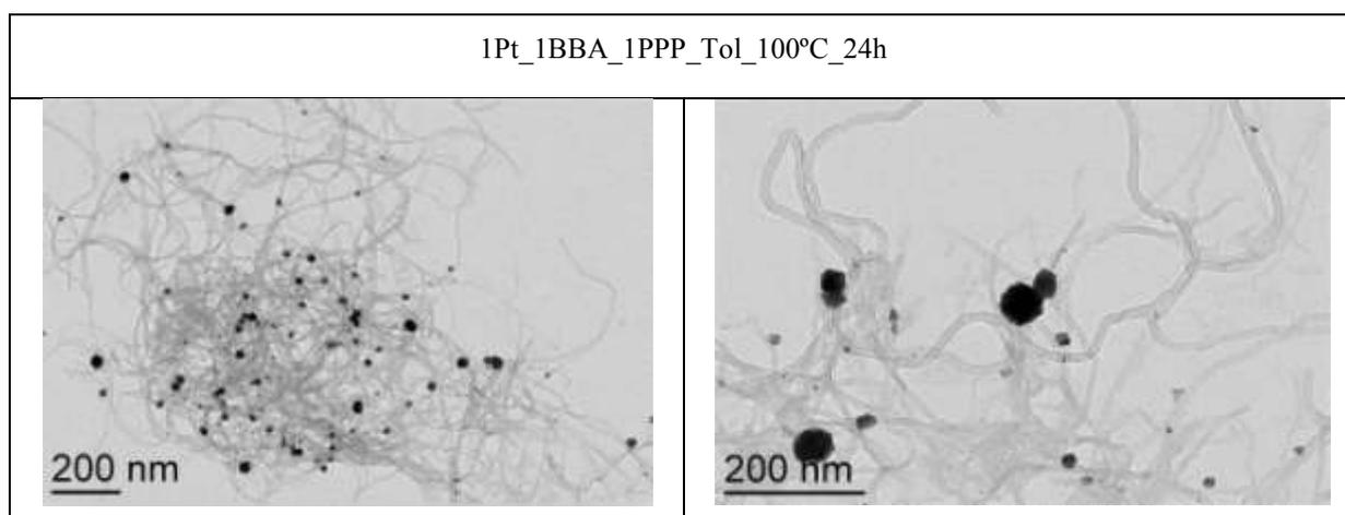
Based on this series of reactions, we can say that BBA and PPP alone or in combination cannot give rise to any confined structure inside the CNTs. This means that something related to the presence of Co assists the entrance of Pt in the CNTs and the formation of NWs, since in its absence the CNTs are always empty. In addition none of these ligands favors the stabilization of small Pt NPs.
