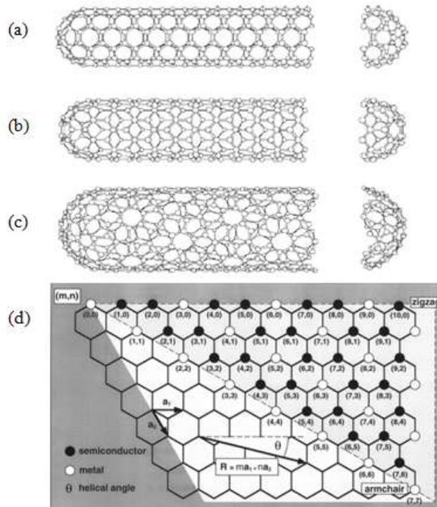
**Figure I.4: Sketches of three different SWCNT structures of (a) an armchair-type, (b) a zig-zag-type and (c) a helical type (26). (d) Sketch of the way to make a SWCNT by a graphene sheet (reproduced from ref.27).**
