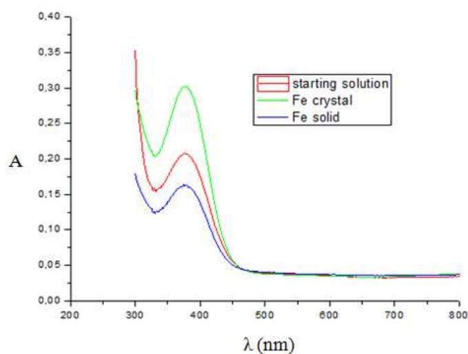
**Figure IV.40: UV-visible spectra comparison among the starting solution of "Pt\_Fe\_2BBA\_2PPP\_Tol\_100°C\_24h", the Fe crystal and the Fe solid.**
