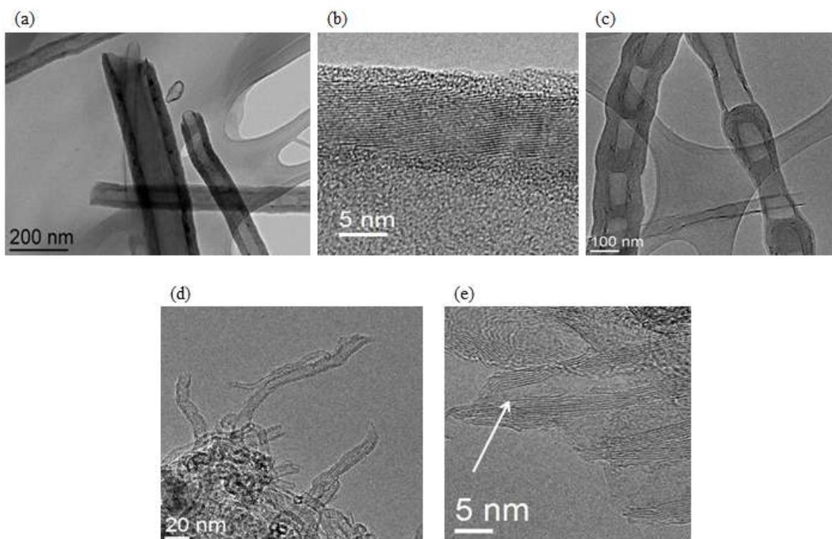
**Figure II.6: (a) TEM image of f-CNT<sub>1</sub> with various diameters; (b) HRTEM image of an amorphous structure on the outer surface of a f-CNT<sub>1</sub>; (c) presence of bamboo-like nanofibers after functionalization; HRTEM images of (d) all the opened f-CNT<sub>2</sub> and (e) a closed f-CNT<sub>2</sub> (white arrow).**
