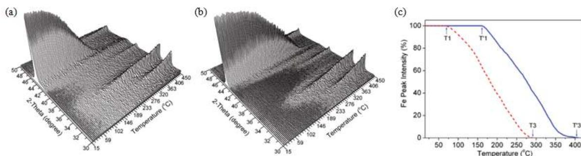
**Figure I. 9: *In situ* XRD patterns of (a) Fe-*out*-CNT; (b) Fe-*in*-CNT; (c) the intensity change of the Fe diffraction peaks during temperature programmed oxidation. The dotted red line in (c) denotes Fe-*out*-CNT, and the solid blue line, Fe-*in*-CNT (reproduced from ref.44).**
