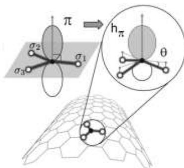
**Figure I.10: Schema showing the  $\pi$  orbital in planar graphene and deviation to hybridized  $\pi$  ( $h_{\pi}$ ) under bending together with the pyramidalization angle  $\theta$  that is the angle between  $\sigma$  and  $\pi$  orbitals minus 90 degree and describes the curvature-induced shift in  $sp^2$  hybridization. ( $0^\circ$  for the  $sp^2$  hybridization and  $19.5^\circ$  for the pyramidalization angle for tetrahedral  $sp^3$  orbital) (reproduced from ref.24).**
