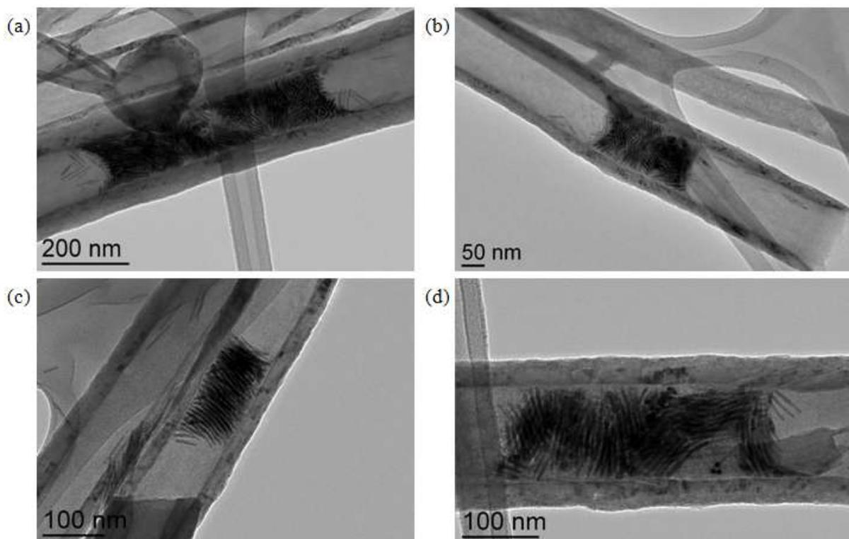
**Figure II.40: (a-d) TEM images of the functionalized Co NRs confined within the f-CNT<sub>1</sub>.**
