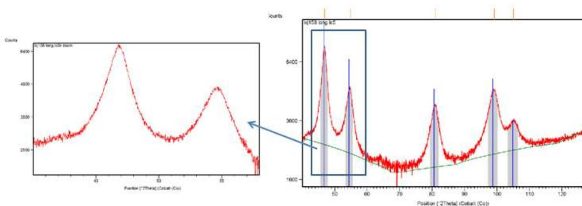
**Figure IV.20: XRD pattern of the CNT-templated Fe-Pt NWs.**
