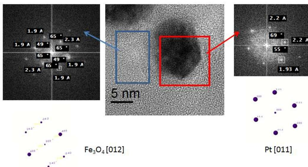
**Figure IV.25: HRTEM analysis of the core/shell nanostructure.**
