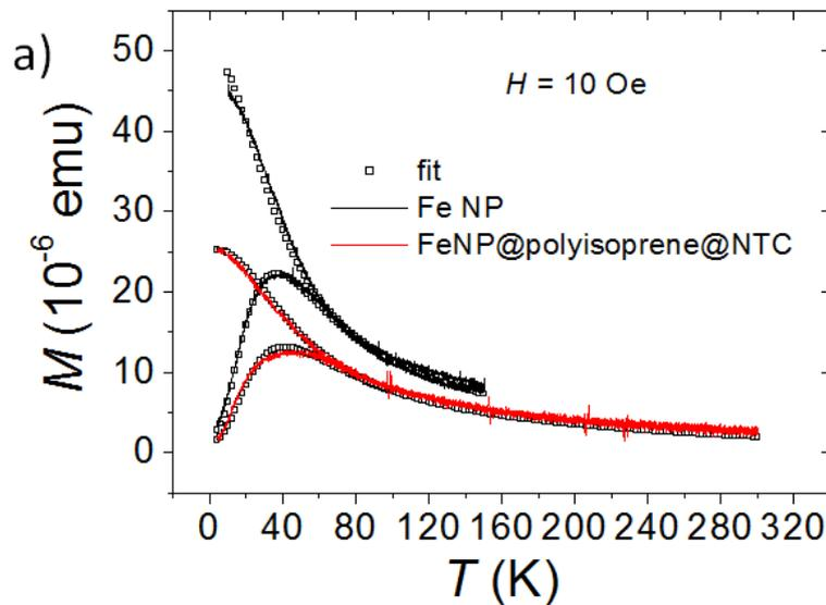
Figure III.24: Magnetic susceptibility measurement under 10 Oe for the Fe NPs and the FeNP@Fe@PI@CNT<sub>1</sub>.
