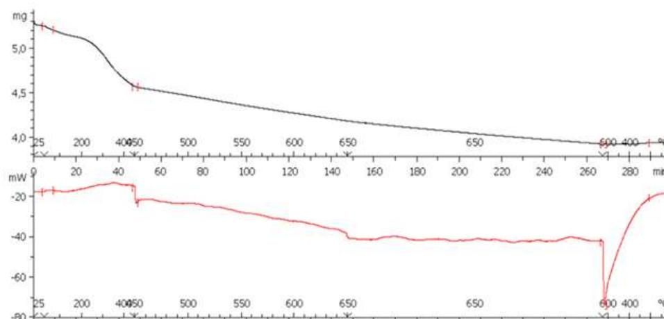
**Figure IV.44: (top) TGA performed under N<sub>2</sub> from RT to 650°C for 2 hours with the Fe-Pt NWs; (bottom) heat flow detected during the annealing.**
