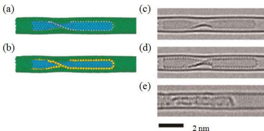
**Figure I.18: Calculated HRTEM images of (c) H- and (d) S-terminated GNRs inside a SWNT and the corresponding models (a) and (b). The experimental image (e), presented for visual comparison, shows that the contrast of the nanoribbon edge matches the model with sulfur atoms (b and d) closer than the model with hydrogen atoms (a and c) (reproduced from ref.139).**
