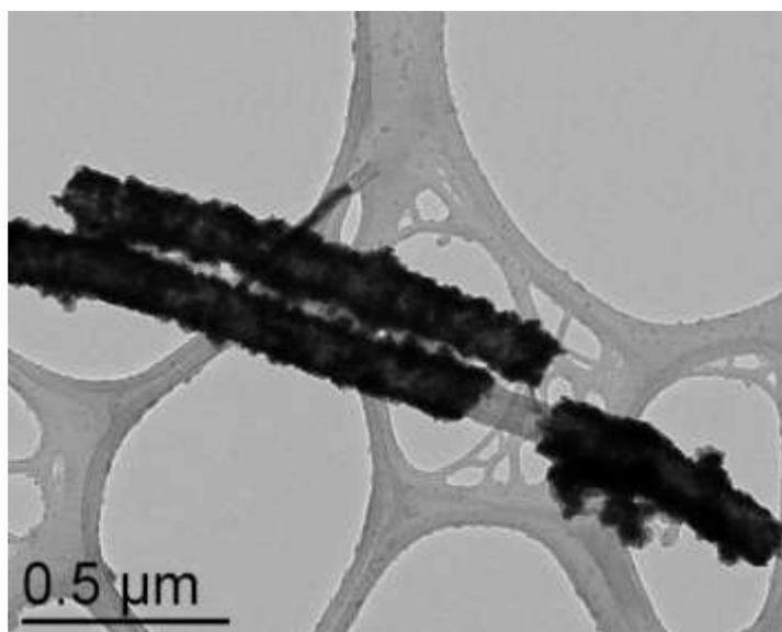
**Figure IV.6: TEM image of the metal-coated f-CNT<sub>1</sub>.**
