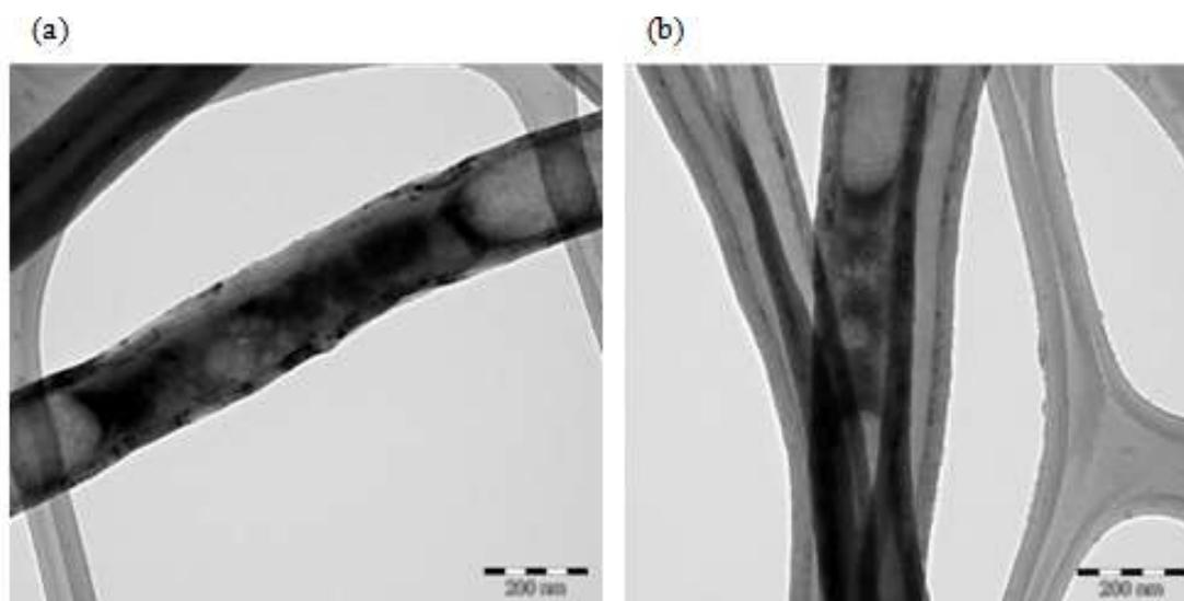
**Figure II.29: TEM images of the f-CNT<sub>1</sub> encapsulating the Fe NPs (24-hours stirring).**
