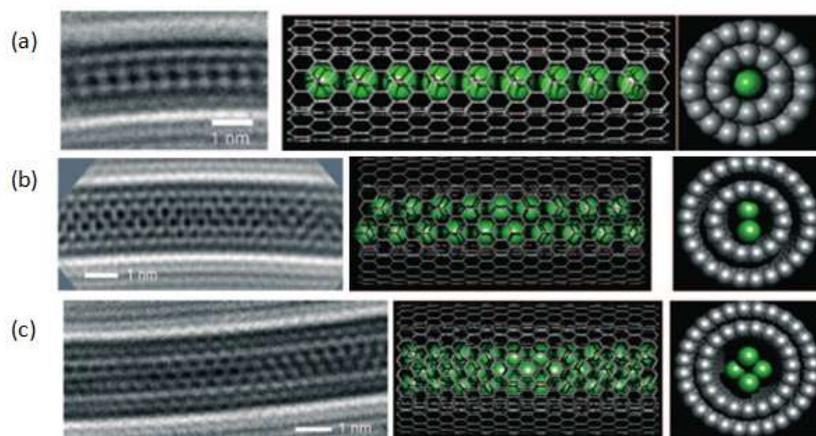
**Figure I.7: Observed HRTEM image (left), simulated HRTEM image (middle), and corresponding structure model (right) of a) single, b) two and c) four atomic chains of Eu atoms encapsulated in DWCNTs. Gray carbon, green europium (reproduced from ref.34).**
