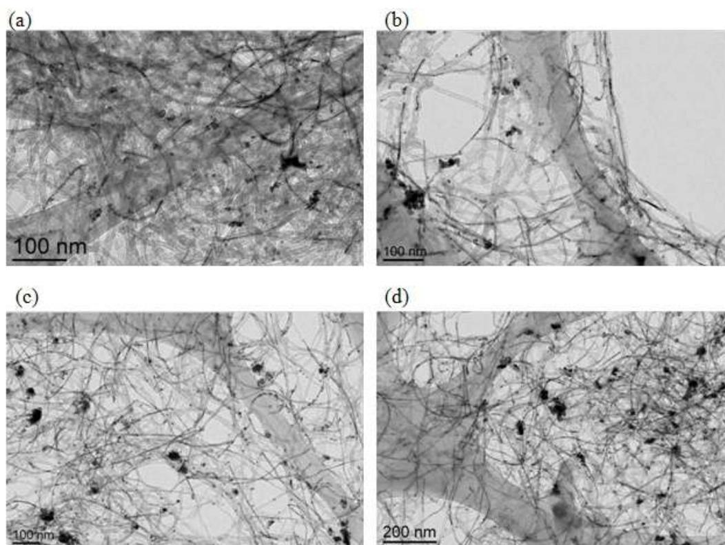
**Figure IV.15: TEM images of "Pt<sub>0.84</sub>Co<sub>0.16</sub>\_2BBA\_2PPP\_Tol\_100°C" during (a) 1h, (b) 3h, (c) 24h and (d) 48h.**
