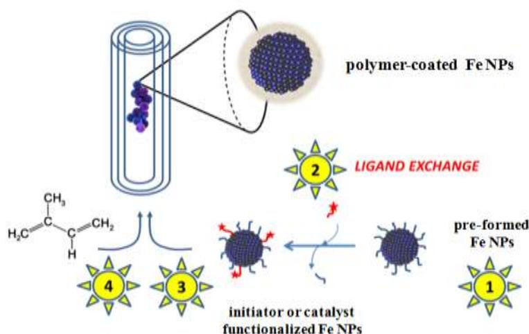
**Figure III.5: Bottom-up approach to produce air-protected Fe NPs confined in f-CNT<sub>1</sub>: (1) synthesis of Fe NPs; (2) surface-modification on the Fe NPs with an initiator or a catalyst; (3) selective confinement of the surface-modified Fe NPs in f-CNT<sub>1</sub>; and (4) polymerization of isoprene in a confined space to produce FeNP@polyisoprene/ f-CNT<sub>1</sub>.**
