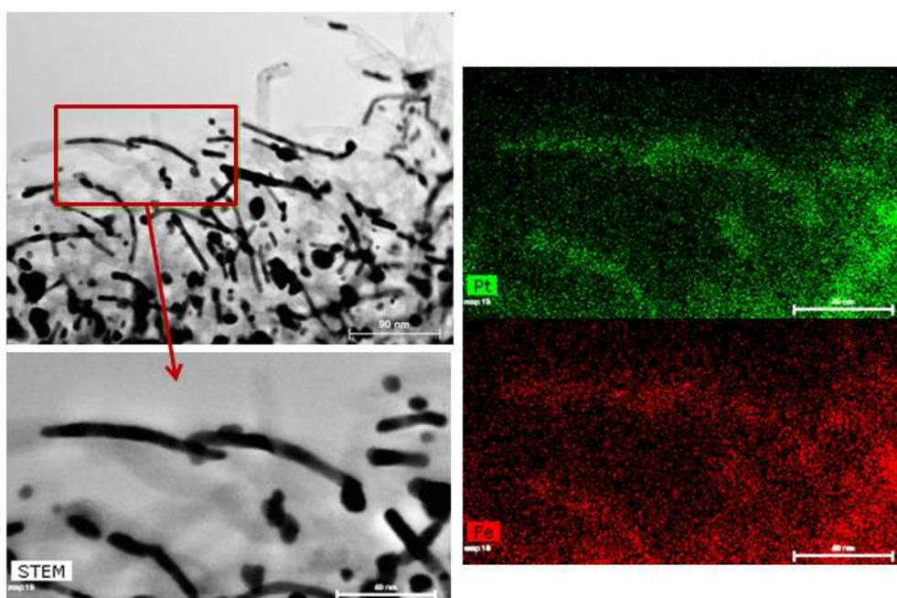
**Figure IV.48: STEM analysis of the annealed sample.**
