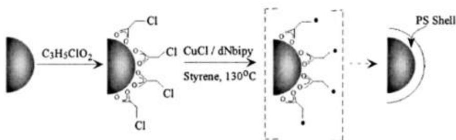
**Figure III.2: Procedure of  $\text{MnFe}_2\text{O}_4$ @polystyrene core/shell NPs synthesis (reproduced from ref.15).**
