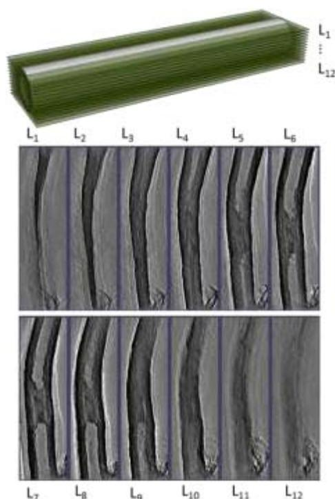
**Figure III.21: Electron tomography analysis of the FeNP@Fe@PI@CNT<sub>1</sub> nanohybrid. Sequential cuts in the Z direction extracted from the reconstruction of the electron tomogram. The upper inset gives a schematic view of the position of the volume cuts represented in the lower insets. The hollow structure of the nanotube and the partial filling is clearly visible from the cuts.**
