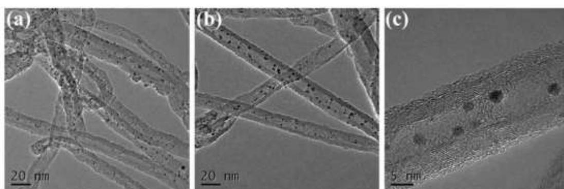
**Figure I. 25: Dispersion of Ru NPs inside the CNT channels using the wet chemistry method: (a) sample obtained without being aided by ultrasonic treatment and extended stirring; (b and c) different magnification images of sample obtained with the aid of ultrasonic treatment and extended stirring (reproduced from ref.112).**
