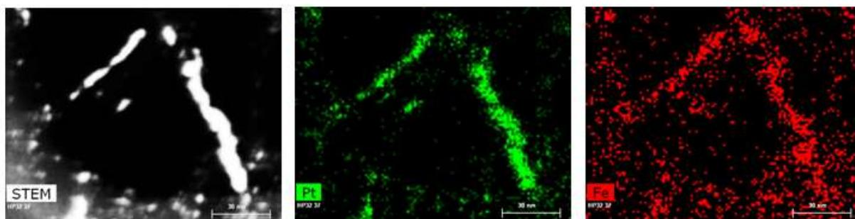
**Figure IV.28: STEM-EDX analysis of the washed sample in "1[Pt(acac)<sub>2</sub>]<sub>1</sub>Fe<sub>2</sub>BBA<sub>2</sub>PPP<sub>2</sub>Tol<sub>150</sub>°C<sub>24</sub>h".**
