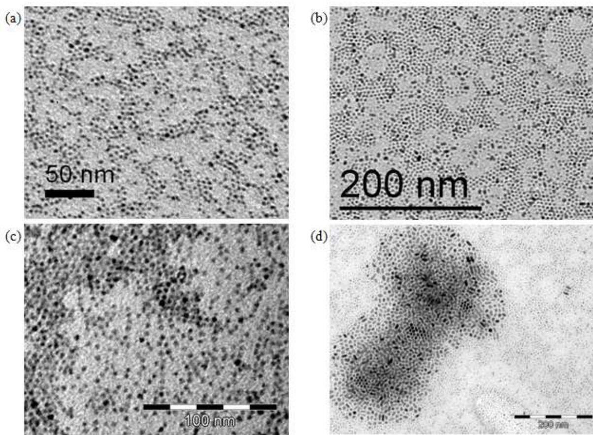
**Figure II.20: TEM images of (a) Co\_1.2LA:1.2PPP\_Mes\_150°C\_24h, (b) Co\_1.2LA:1.2PPP\_Mes\_120°C\_24h, (c) Co\_1.2LA:1.2PPP\_Ani\_150°C\_24h, and (d) Co\_1.2BBA:1.2HDA\_Ani\_150°C\_24h with "one injection" adding rate.**
