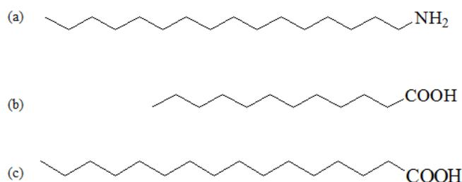
**Figure II.10: (a) Hexadecylamine (HDA); (b) Lauric acid (LA) (c) Palmitic acid (PA).**
