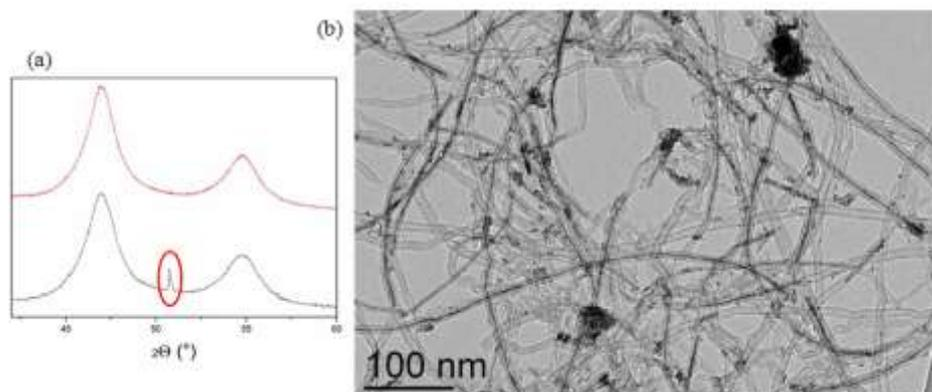
**Figure IV.12: (a) XRD pattern of the sample after HCl washing (red) and before washing (black). We can note the absence of the Co phase (red cycle); (b) TEM image of the HCl washed CNT-templated Co-Pt NWs.**
