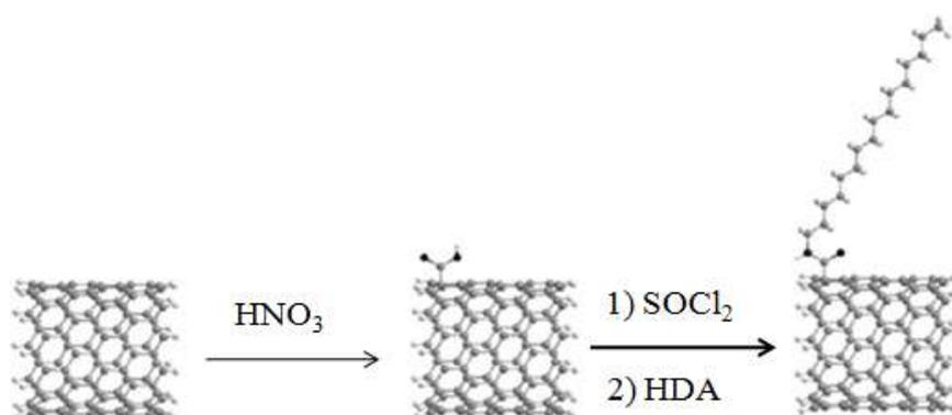
**Figure II.5: Functionalization process of pristine MWCNTs to produce f-MWCNTs (10).**
