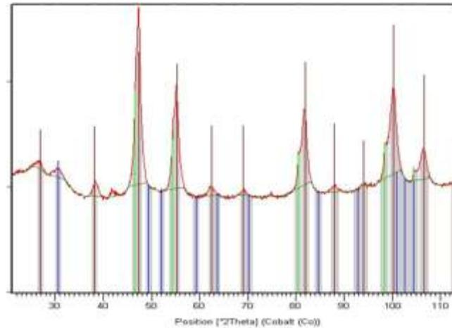
**Figure IV.45: XRD pattern of the TGA annealed Fe-Pt NWs that presents a phase associated to CNTs (blue), a ordered FePt<sub>3</sub> phase (brown) and a phase close to Pt (green).**
