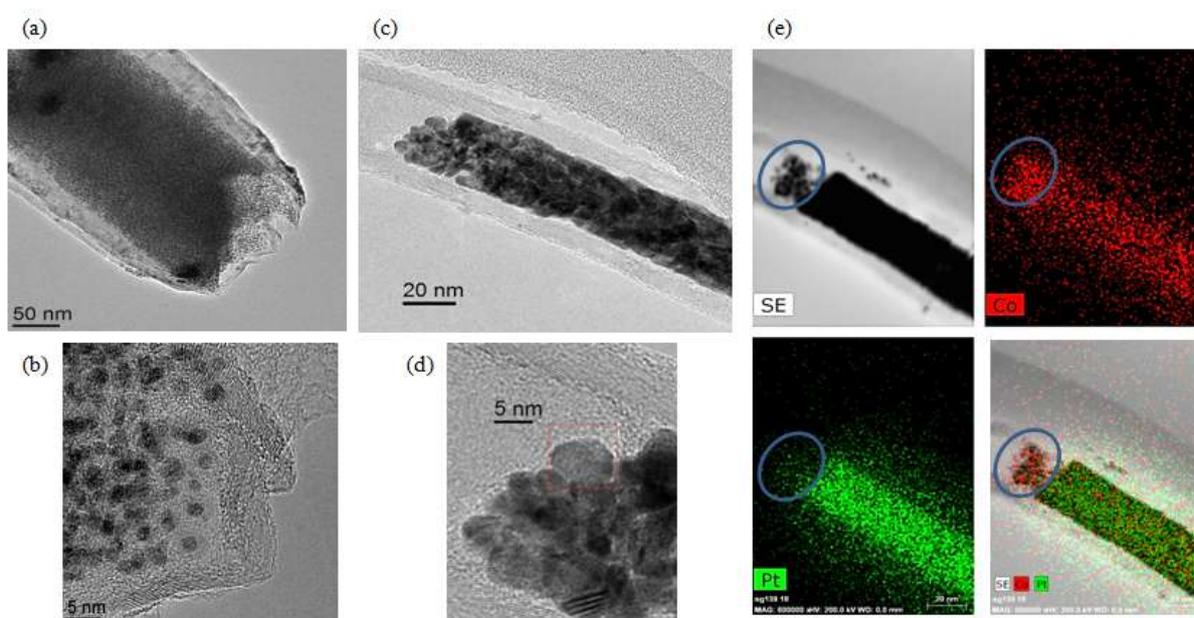
**Figure IV.5: (a-b) TEM images of the confined NPs within the f-CNT<sub>1</sub> of larger diameter; (c-d) TEM images of coalesced NPs within the f-CNT<sub>1</sub> of smaller diameter; (e) STEM analysis of the content of a tube containing both kinds of NPs (blue cycle highlight the small confined NPs rich in Co).**
