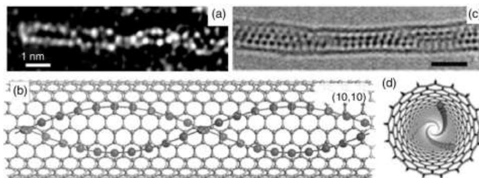
**Figure I.6: (a) High-resolution Z contrast TEM of the first example of SWCNTs filled with a double-helix chain of iodine atoms; (b) Side view of a model for the image in (a) considering a (10,10) tube as the containing SWCNT (reproduced from ref.33); (c) High-resolution TEM**
