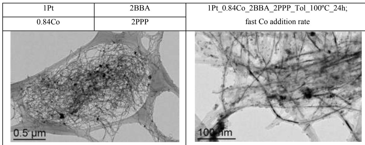
In another experiment we changed the preparation procedure of the starting solution by modifying the addition order: Co was mixed first with the acid, then the amine was added to them and finally Pt was added to the mixture. (BBA+Co+PPP+Pt) compared to the order "BBA+Pt+PPP+Co" in all other reactions. This modification led to more NPs and aggregates outside the CNTs.
