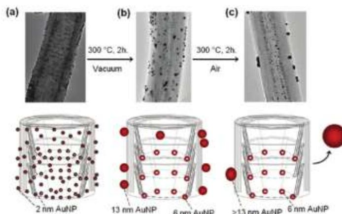
**Figure I.8: TEM images and schematic diagrams illustrating the Au NPs adsorbed on the GNF outer surface and anchored at the graphitic step-edges within the GNF (a) immediately after the deposition of 2.3nm Au NPs, (b) after heating the Au NP-GNF composite in vacuum at 300°C for 2h, and (c) after additional heating at 300°C in air for a further 2h, and post-heating in vacuum (reproduced from ref.43).**
