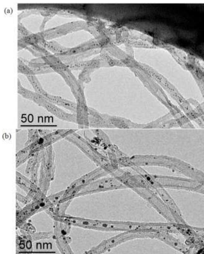
**Figure IV.55: TEM images of the sample of the CNT<sub>3</sub>-confined Fe-Pt NPs (a) before and (b) after annealing.**
