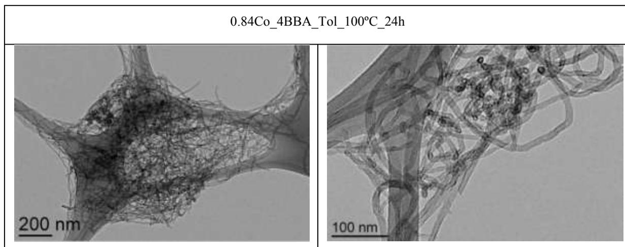
The presence of 4 equivalents of PPP results in NPs (5-15 nm) located outside the CNTs. This result is similar to the one obtained in the absence of any aromatic ligands. The HMDS alone seems to be able to stabilize Co NPs of a smaller size than the PPP and the HMDS together.
