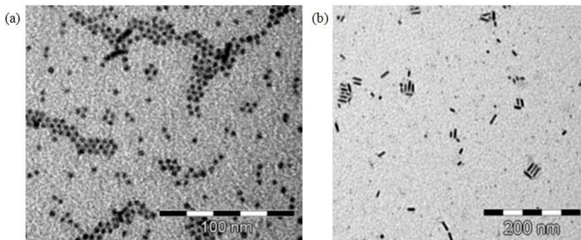
**Figure II.11: TEM images of (a) Co<sub>1.2</sub>LA:1.2HDA\_Mes\_150°C\_24h; (b) Co<sub>1.4</sub>LA:1.2HDA\_Mes\_150°C\_24h.**
