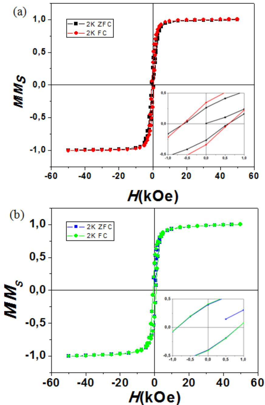
**Figure II.38: Hysteresis loops of (a) the pre-formed Fe NPs and (b) the FeNP@CNT<sub>1</sub> at 2K performed by SQUID.**
