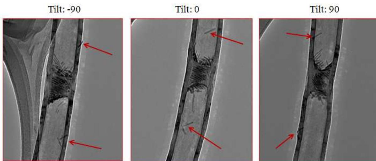
**Figure II.41: Tomography images of the confined Co NRs within f-CNT<sub>1</sub>. The NRs on the outer surface are highlighted by the red arrows.**
