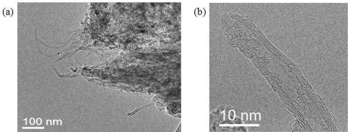
**Figure II.3: TEM micrographs of (a) the bundles of CNT<sub>2</sub> and (b) a closed CNT<sub>2</sub> with 5 walls.**
