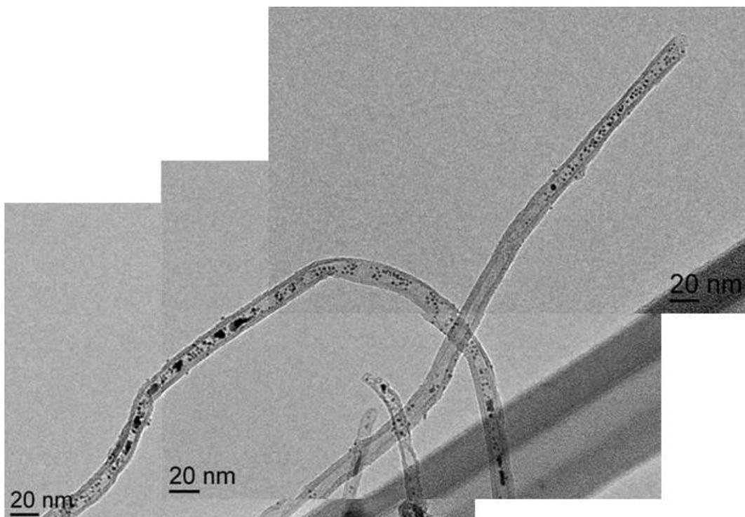
**Figure IV.29: TEM image of a well filled CNT<sub>3</sub> in which both small NPs and coalescences are formed.**
