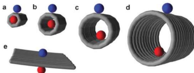
**Figure II.31: Schematic diagrams of small molecules adsorbed on the outer (blue) and inner (red) surface of CNTs with different diameters ( $d_{\text{molecule}}$  is van der Waals diameter of molecule, and  $d_{\text{CNT}}$  is internal van der Waals diameter of CNT): (a)  $d_{\text{CNT}} < d_{\text{molecule}}$ , (b)  $d_{\text{CNT}} \sim d_{\text{molecule}}$ , (c)  $d_{\text{CNT}} > d_{\text{molecule}}$ , (d)  $d_{\text{CNT}} \gg d_{\text{molecule}}$ , (e)  $d_{\text{CNT}}$  infinite (15).**
