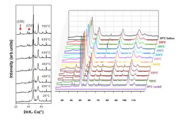
Figure IV.49: XRD pattern for the *in situ* annealing until 700 °C. The new (100) and (110) planes are indicated by red arrows on the left longitudinal comparison.
