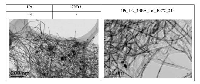
The reduction of the BBA content in the starting solution and without PPP, "1Pt\_1Fe\_1BBA\_Tol\_100°C\_24h" gave rise to core/shell NPs (12-35 nm) outside the CNTs instead of the CNT-templated NWs.
