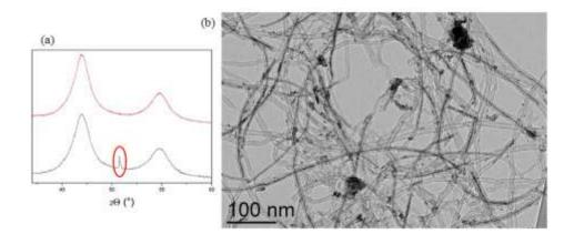
Figure IV.12: (a) XRD pattern of the sample after HCl washing (red) and before washing (black). We can note the absence of the Co phase (red cycle); (b) TEM image of the HCl washed CNTtemplated Co-Pt NWs.
