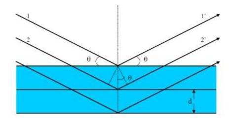
Figure A.9: Diffraction of X-rays from a crystal displaying planes separated by a distance d.
