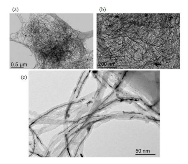
Figure IV.18: TEM images of the Fe-Pt NWs from "1Pt\_1Fe\_2BBA\_2PPP\_Tol\_100°C\_24h".
