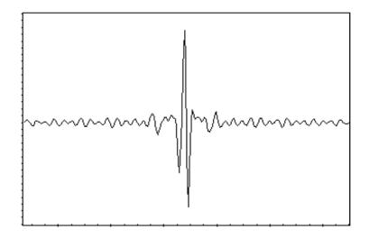
Figure A.7: Interferogram produced by the FT-IR interferometer.
