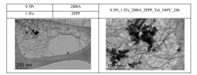
Therefore in another reaction, we kept one equivalent of Pt in order to maintain the amount of NWs, while we doubled the Fe content and the ligands in the starting solution in order to avoid the formation of aggregates. From TEM, the amount of NWs seems to be the same as that in the reference reaction "1Pt\_1Fe\_2BBA\_2PPP\_Tol\_100°C\_24h", whereas the big aggregates are still present.
