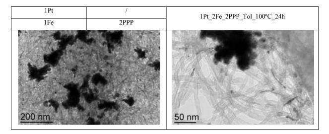
When 2 equivalents of PPP and 1 equivalent of BBA were added to the starting solution the core/shell structure was absent but some NWs and several aggregates were present. Therefore PPP plays a role for the NW formation when only one BBA is present. It is possible that in the presence of PPP, the BBA is not completely consumed by the Fe, and some of it can participate to the formation of species that can enter in the CNTs.
