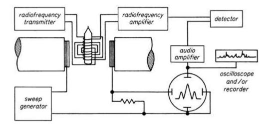
Figure A.12: Simple schematic representation of an NMR spectrophotometer.
