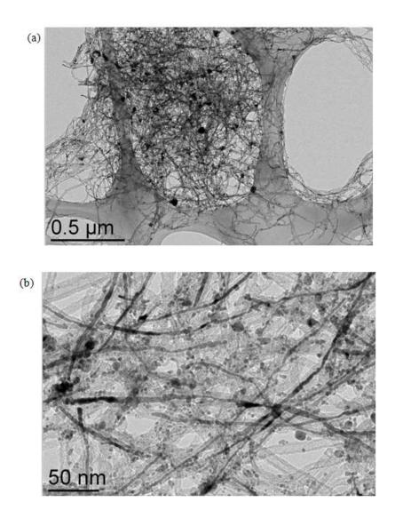
Figure IV.8: (a-b) TEM images of the CNT-templated Co-Pt NWs and the polydispersed NPs attached on the outer surface of the f-CNT<sub>2</sub>.
