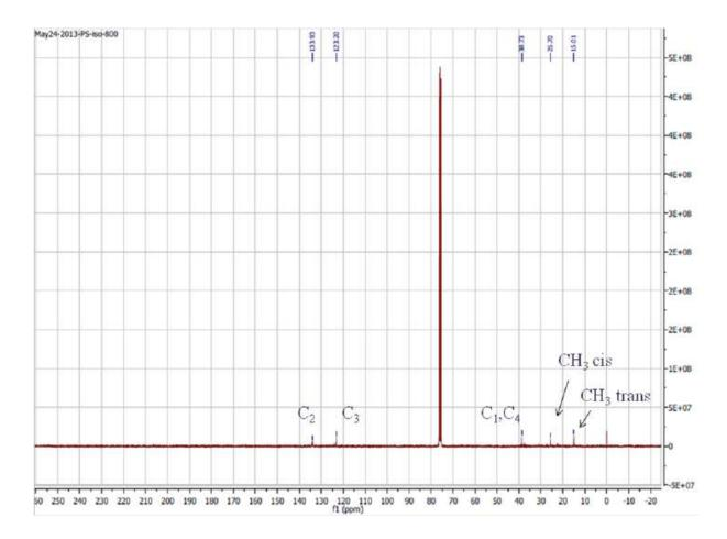
Figure V.2: NMR <sup>13</sup>C of polyisoprene in CDCl<sub>3</sub>.
