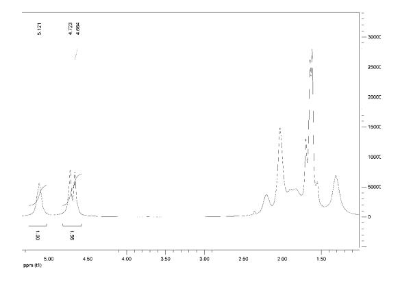
Figure V.3: NMR <sup>1</sup>H of Fe complex in CDCl<sub>3</sub>.
