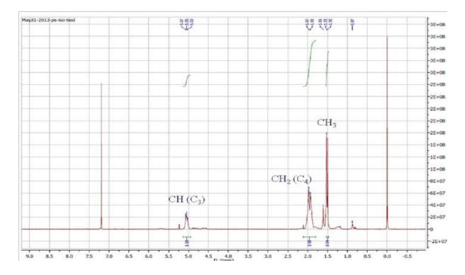
Figure V.1: NMR <sup>1</sup>H of polyisoprene in CDCl<sub>3</sub>.
