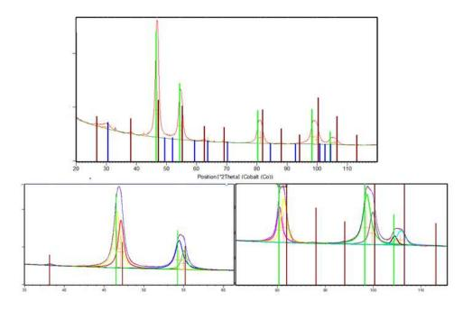
Figure IV.54: XRD pattern of the polyisoprene-coated Fe-Pt NWs at 600°C for one hour. Blue, green and brown lines correspond respectively to carbon, Pt and ordered FePt<sub>3</sub> phases.
