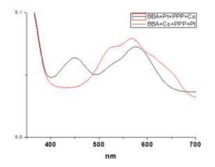
Figure IV.17: Comparison of UV-vis spectra between the addition order "BBA+Pt+PPP+Co" (black) and "BBA+Co+PPP+Pt".
