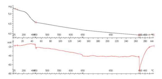
Figure IV.44: (top) TGA performed under N<sub>2</sub> from RT to 650°C for 2 hours with the Fe-Pt NWs; (bottom) heat flow detected during the annealing.
