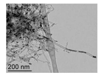
Figure IV.53: TEM image of the annealed Fe-Pt NWs which were pre-coated with polyisoprene before annealing.
