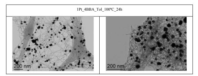
The NPs formed outside the CNTs are more polydispersed (15-100 nm), which indicates that neither BBA is able to stabilize small Pt NPs.
