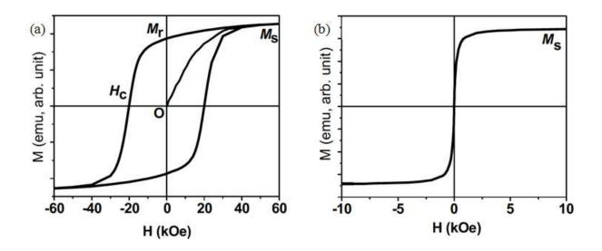
Figure B. 4: Schema of the hysteresis loops of (a) ferromagnetic NPs and (b) superparamagnetic NPs (10).
