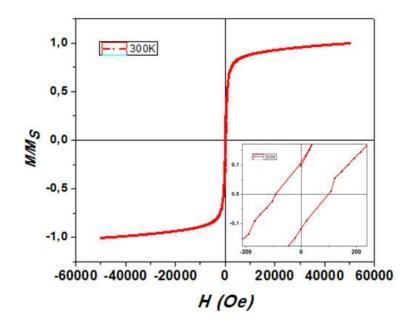
Figure IV.43: Hysteresis loop of the non-annealed Fe-Pt NWs at 300K. Inset is a magnification close to zero point.
