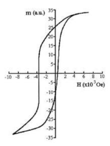
Figure B.5: Hysteresis loop of Co@CoO particles at 77K after field cooling (FC) (11).
