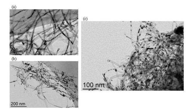
Figure IV.46: TEM images of (a) the Fe-Pt NWs before annealing and (b-c) after annealing.
