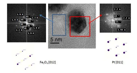
Figure IV.25: HRTEM analysis of the core/shell nanostructure.
