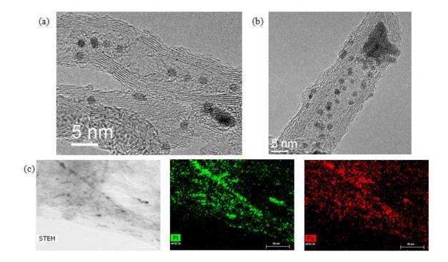
Figure IV.27: (a-b) HRTEM images and (c) STEM-EDX analysis of the washed sample in "1[Pt(acac)<sub>2</sub>]\_1Fe\_2BBA\_2PPP\_Tol\_100°C\_24h".
