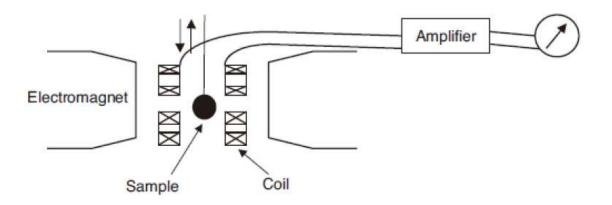
Figure A.4: Schematic representation of a VSM.
