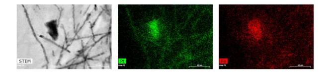
Figure IV.24: STEM-EDX analysis of the washed "1Pt\_2Fe\_4BBA\_4PPP\_Tol\_100°C\_24h" sample.
