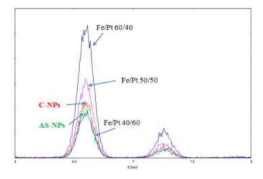
Figure IV.31: XRF Fe Kα and Fe Kβ patterns of the comparison of the C-NPs (red) and AS-NPs (green) with the standard Fe/Pt composition prepared with organometallic complexes. (Amplitudes are normalized on the Pt L pattern).
