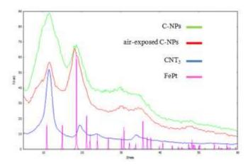
Figure IV.32: WAXS pattern of comparison among the C-NPs (green), air-exposed C-NPs (red), CNT<sub>3</sub> (blue) and standard FePt (pink).
