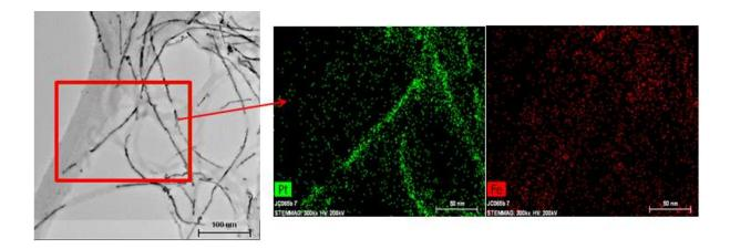
Figure IV.22: STEM-EDX analysis of the Fe-Pt NWs.
