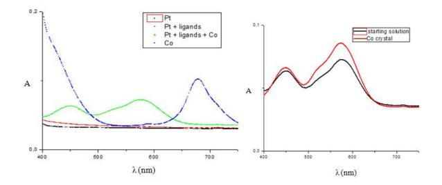
Figure IV.37: UV-visible spectrum. (left) The preparation of the starting solution of "Pt\_0.84Co\_2BBA\_2PPP\_Tol\_100°C\_24h"; (right) Comparison between the starting solution and the Co crystal in toluene.
