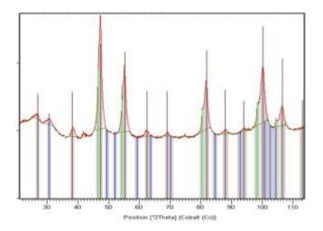
Figure IV.45: XRD pattern of the TGA annealed Fe-Pt NWs that presents a phase associated to CNTs (blue), a ordered FePt<sub>3</sub> phase (brown) and a phase close to Pt (green).
