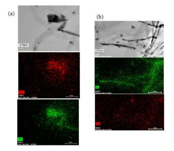
Figure IV.13: STEM-EDX analysis of HCl washing sample.
