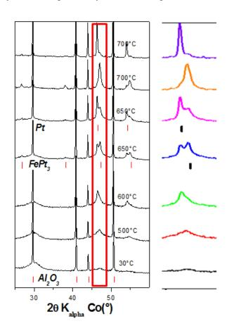
Figure IV.57: (left) Evolution of the phases detected by XRD during the *in situ* annealing; (right) magnifications of the peaks at  $2\theta = 47^{\circ}$  for all the XRD patterns.
