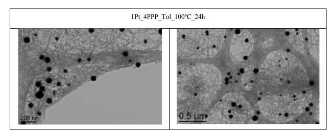
Therefore the addition of 4 equivalents of PPP gives rise to polydispersed NPs (55-100 nm) outside the CNTs while the CNTs remained empty. The NPs are smaller that in the absence of ligands but this experiment apart from the failure of complexes containing only PPP to enter and/or to be reduced into the CNTs, also indicates that PPP alone cannot stabilize small Pt NPs.
