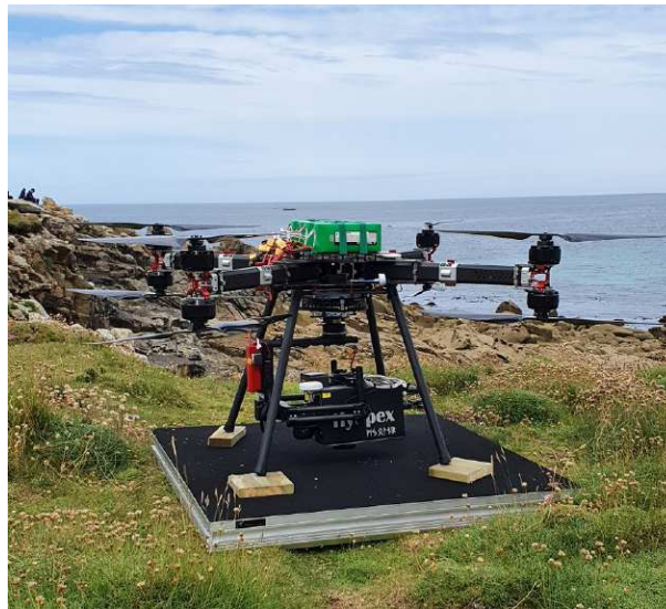
FIGURE 3.2 – UAV octocopter used for the acquisitions.
