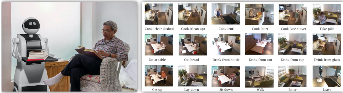
Fig. 1.1 Real-word Action Classification System and Applications. For instance, when applied within the context of robotics for elderly care, this technology holds the promise of enabling robots to not only comprehend human actions but also to anticipate needs, to offer timely aid, and to establish meaningful human-robot interactions.
