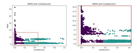
Fig. 3.8 Distribution of aggregated poses with MPJPE and Confidence. (purple: high confidence with  $\gamma >= 0.18$ , green: low confidence with  $\gamma < 0.18$ ) Zoom of the red bounding box is on the right.
