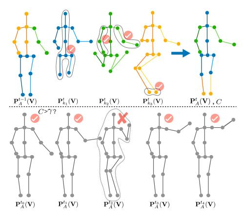
Fig. 3.4 **Two steps of SST-Aggregation**. 1) Aggregation in both spatial and temporal level (top). The pose  $\mathbf{P}_{A}^{t}(\mathbf{V})$  of current frame is aggregated from the three pose proposals  $\mathbf{P}_{k_1}^{t}(\mathbf{V})$  (blue),  $\mathbf{P}_{k_2}^{t}(\mathbf{V})$  (green) and  $\mathbf{P}_{k_3}^{t}(\mathbf{V})$  (yellow). 2) Selective temporal filter (bottom). The pose with a low confidence in the aggregated sequence will be discarded.
