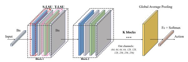
Fig. 3.5 **Overall architecture.** There are K blocks with a 1D Batch normalization layer at the beginning, a global average pooling layer and a fully connected classifier at the end. Each block contains a Spatial Long-short dependency Unit (**S-LSU**), a Temporal Long-short dependency Unit (**T-LSU**) and two Batch normalization layers.
