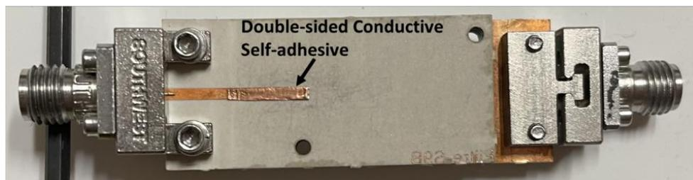
Fig. 4.19 Proposed filter with the correction.
