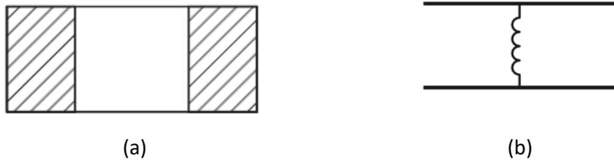
Fig. 3.19 (a) Symmetrical inductive and (b) equivalent circuit.
