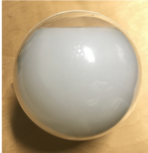
Figure 2.6: The glutamate ball phantom. The diameter of the ball is 14 cm.
