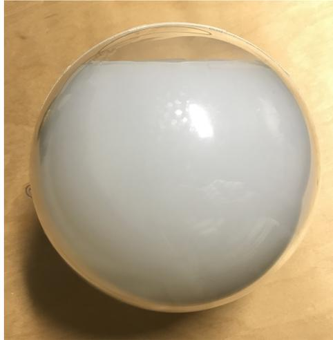
Figure 2.6: *The glutamate ball phantom. The diameter of the ball is 14 cm.*
