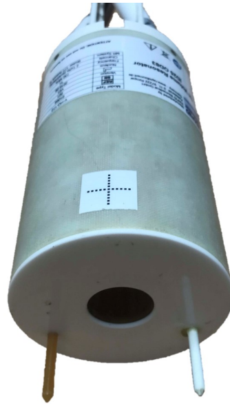
Figure 2.4: Volumic coil used for the experiments on the 17.2 T.
