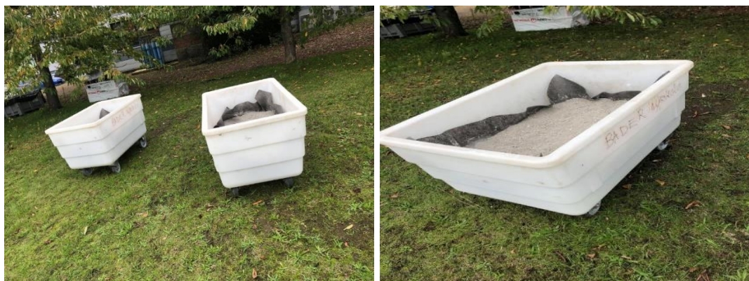
Figure 2. Pilot-scale natural carbonation processes
