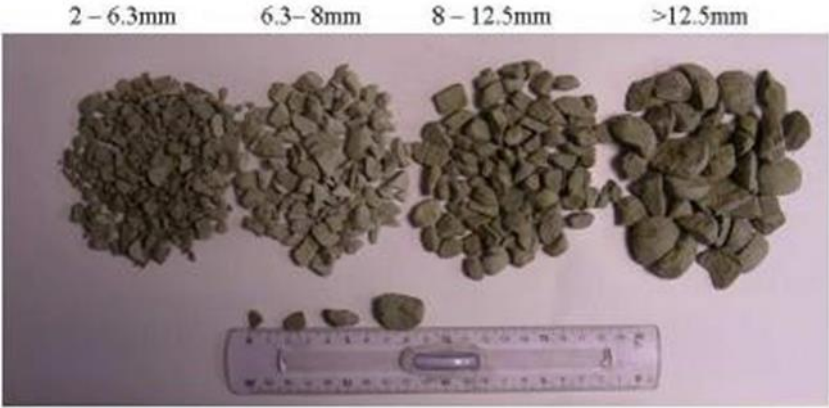
Figure 21. Marine sediment-based aggregates (Brakni 2008)
