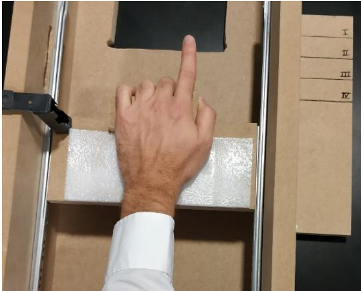
Figure 2.1: Experimental apparatus in the line reaching task. Participants pushed or pulled the platform so that their fingertip match the position of the line specified by the experimenter. Contrary to the picture, participants could not see the inside of the box, as a lid covered the apparatus.
