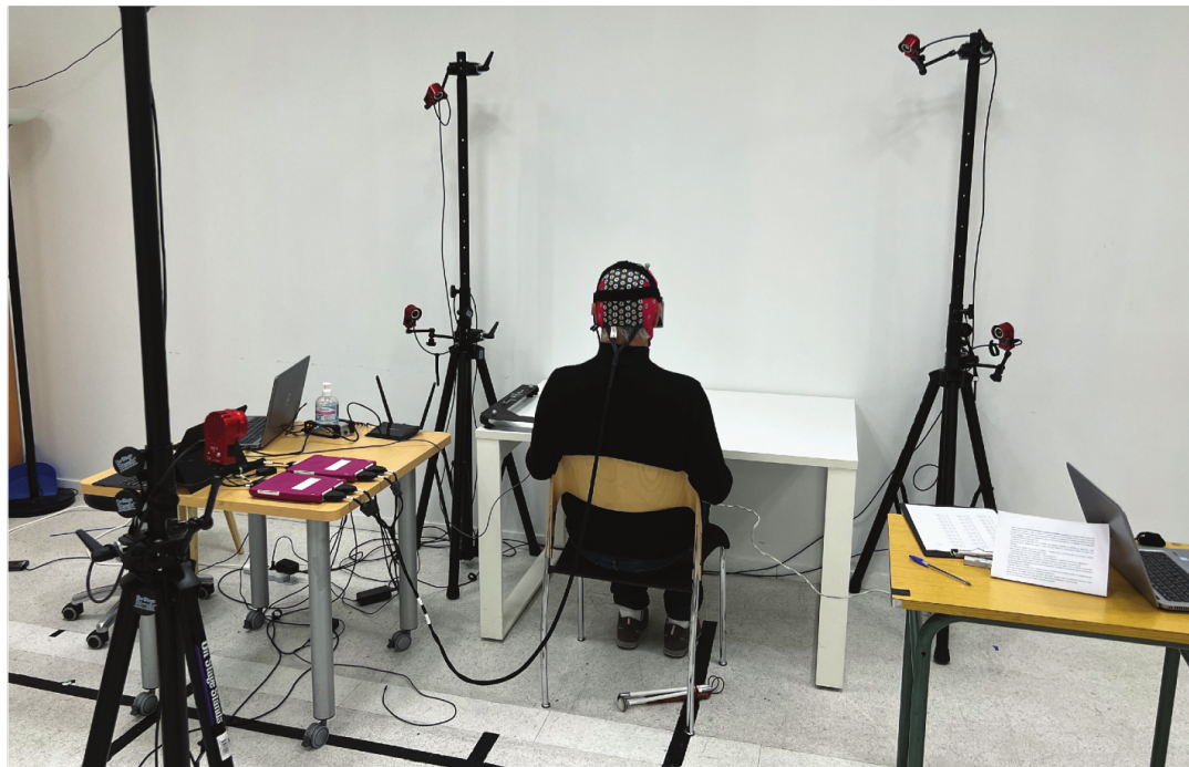
Figure 10.4: Protocol of the visual detection task coupled with EEG recordings. a. Experimental protocol. A session includes two conditions: natural monocular; and stimulated monocular. Each condition is divided into four blocks consisting of ten trials each: five object trials and five no-object trials (tumbler removed from the table). Patients are instructed to close their eyes during the first 5 s of the trials. Patients are then asked to open their eyes, are given 15 s to determine visually whether the tumbler is present on the table, and are then instructed to close their eyes. A second later, they are asked to provide their answer through a two-key response pad, and to specify the level of confidence in their answer by a number between 1 and 5 (see Section 10.2.3.2). b. Experimental setup. Behavioral responses, motion capture, and brain activity were simultaneously recorded during the test.
